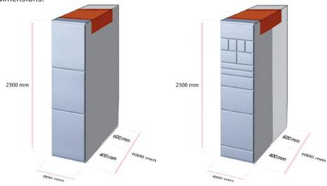
Dimensions and main busbar system configuration
