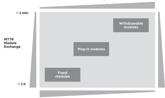
Tools required for module exchange
