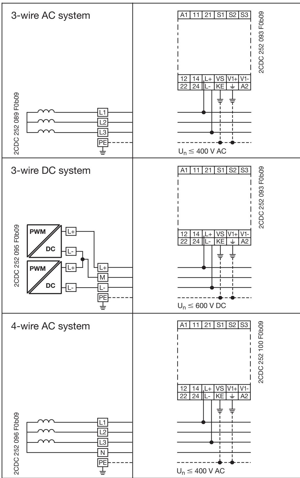
Always connect L+ and L- to different conductors. L+ and L- can be connected to any of the conductors
