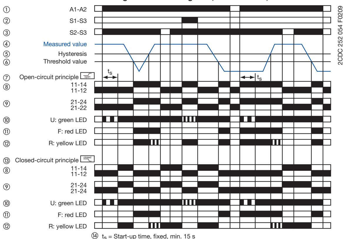
c) Insulation resistance monitoring w/o fault storage
