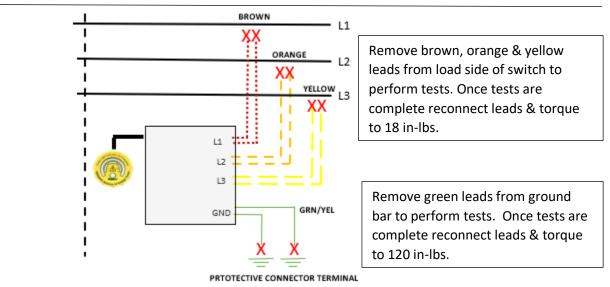
Fig. 1: Representation of VeriSafe™ AVT. The Red X's indicate the sense leads that shall be disconnected for Hi-Pot or Dielectric testing – reconnect all leads once testing is complete.
