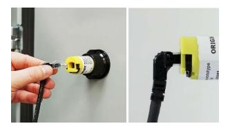
4. Insert the end of the AVT system cable with the right-angle connector in the back of the yellow indicator module. Press firmly into the opening until you feel it latch. Pull back on the connector to verify that it has properly latched. Verify the black tabs on either side are engaged to lock in the cable.
