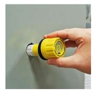
1. Remove the indicator module (yellow device) from the packaging and insert in the 30mm knockout hole, aligning the antirotation notch. Ensure the rubber washer is on the outside of the enclosure.
