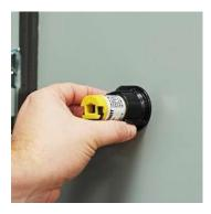
3. Tighten the panel nut until both it and the sealing washer make full contact with the enclosure surface. Then, tighten an additional <sup>1</sup>/<sub>4</sub> turn. Tighten the panel nut with fingers only, **do not overtighten**.
