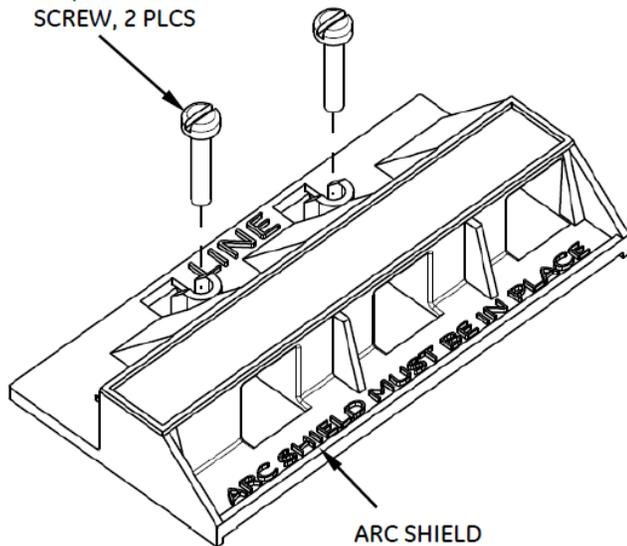
**Fig.1: Representation of Arc Shield**
