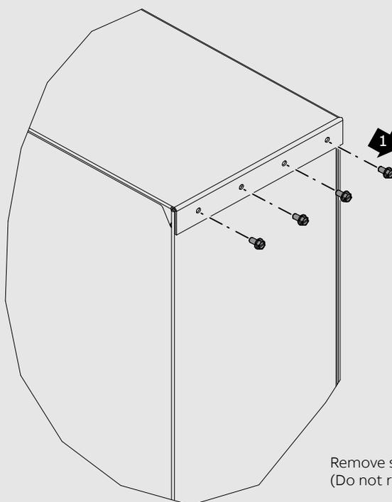
Remove screws from both sides of existing top panel
