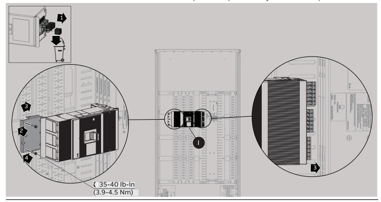
Horizontal main - XT5 B-phase components only included for 3-phase assemblies
