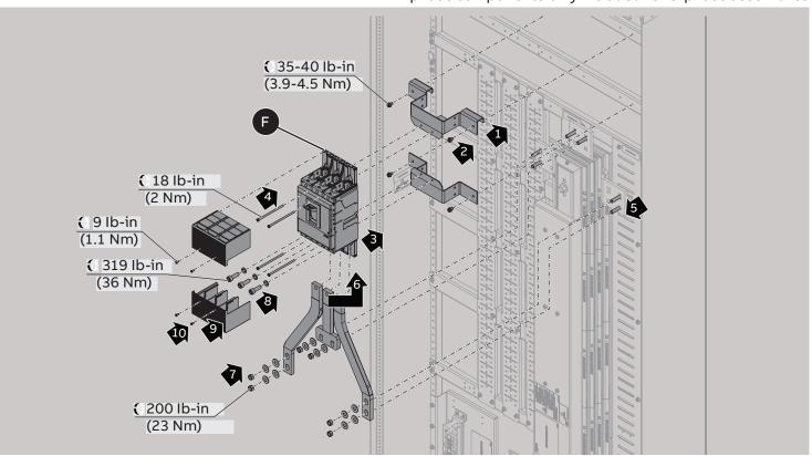
Horizontal main - XT7 B-phase components only included for 3-phase assemblies
