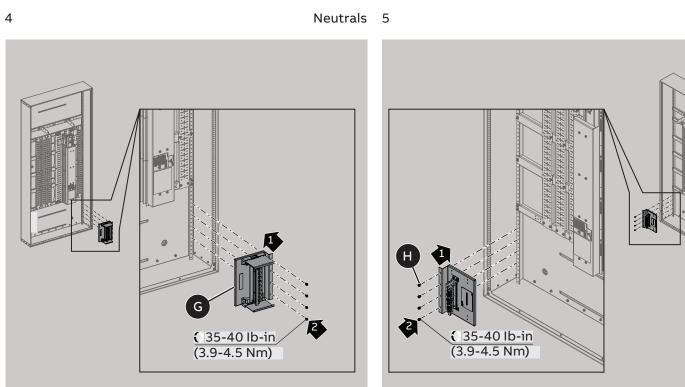
Can be installed in any of the four corners
