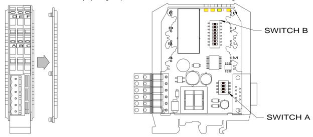
SWITCH A: used for hardware configuration of RS485
