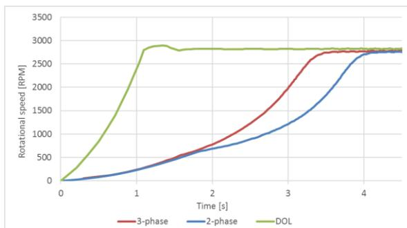
**Figure 16:** Speed comparison between DOL and the two softstarter technologies with voltage ramp. The DOL start is completed
