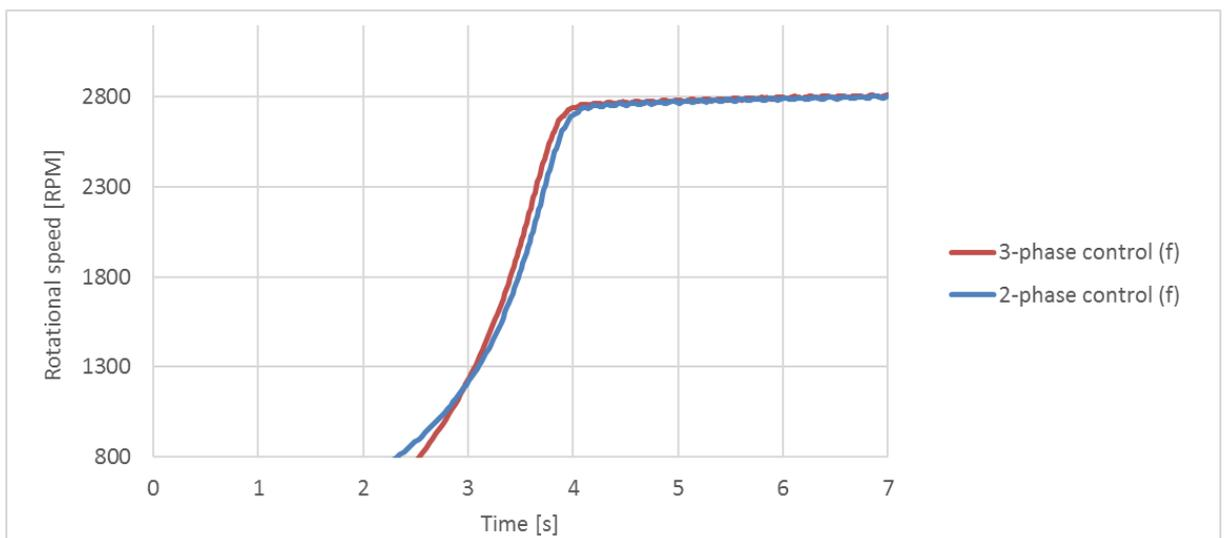
**Figure 15:** Time-shifted graph for comparison of ramps between 700 and 2800 RPM.
