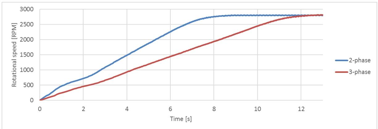
**Figure 18:** Rotational speed over time with torque ramp with a light load for both 2- and 3-phase controlled softstarters with different acceleration times. Both ramps are equally good but finishes the acceleration at different times.
