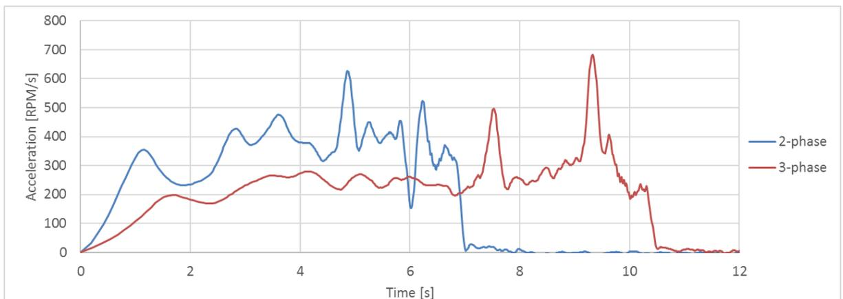
**Figure 20:** Acceleration comparison between 2- and 3-phase softstarters with torque control for the speed-time curves from Figure **Figure 18** above. Both accelerations are many times lower compared
