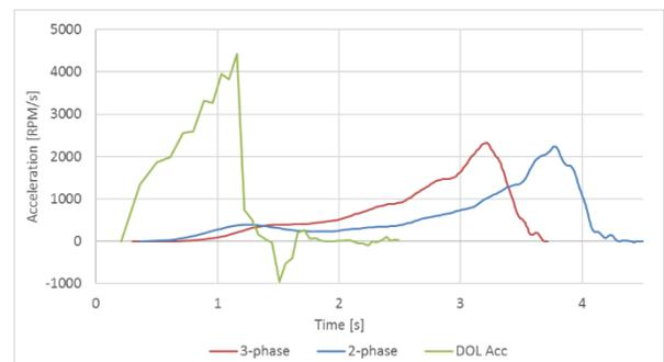
**Figure 17:** Acceleration comparison between DOL and the two different softstarter technologies with voltage ramp.
