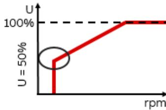
**Figure 1:** Voltage during softstarter.
