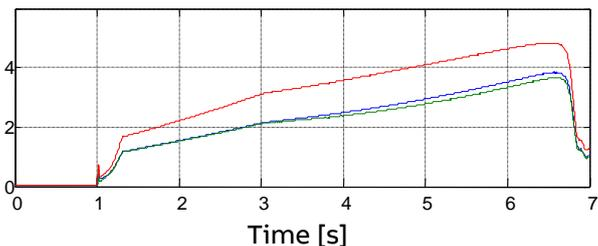
**Figure 8:** RMS current with 2-phase control without current limit.
