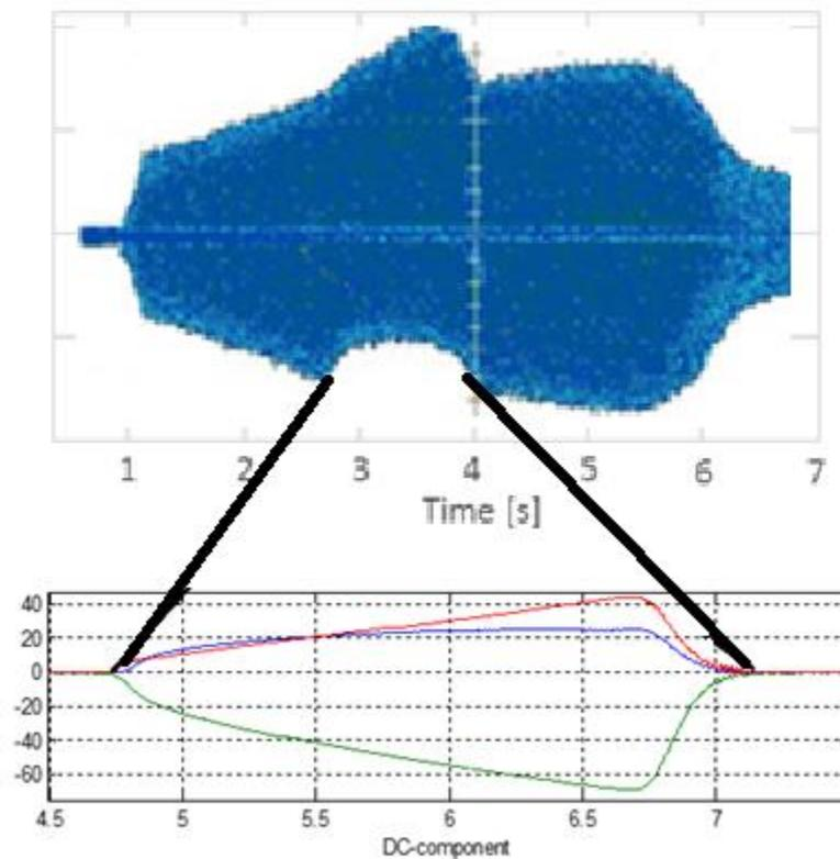
**Figure 11:** The DC component visualized, and how it's related to the individual phase currents.
