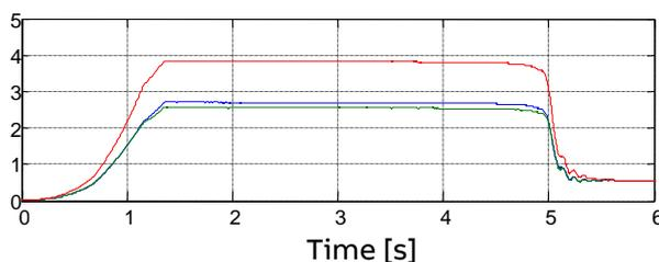
**Figure 7:** RMS current with 2-phase control with current limit.
