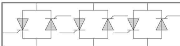
**Figure 4:** Thyristor topology of a "3-phase softstarter": 3 sets of anti-parallel thyristors.
