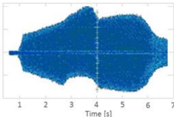
**Figure 12:** DC component from a 2-phase controlled softstarter without compensation algorithm.
