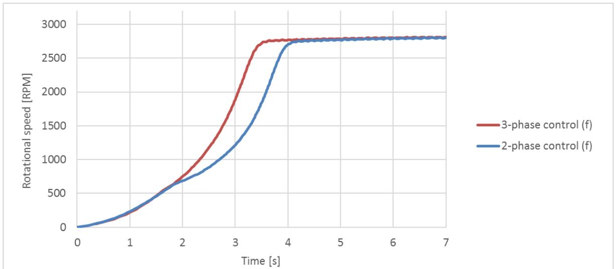
**Figure 14:** Rotational speed with voltage ramp with a light load for both 2- and 3-phase controlled softstarters with different acceleration times. Both ramps are equally good and the application would experience very similar behavior.
