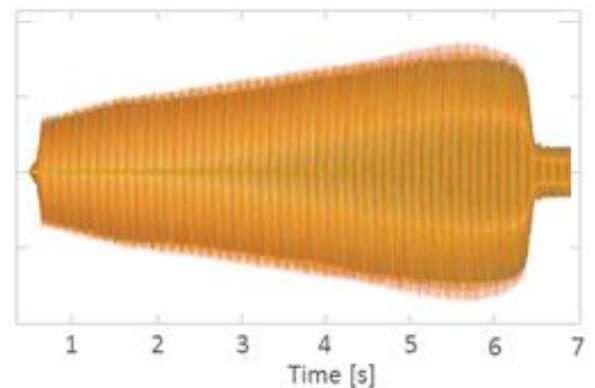
**Figure 13:** 2-phase controlled softstarter with compensation algorithm.
