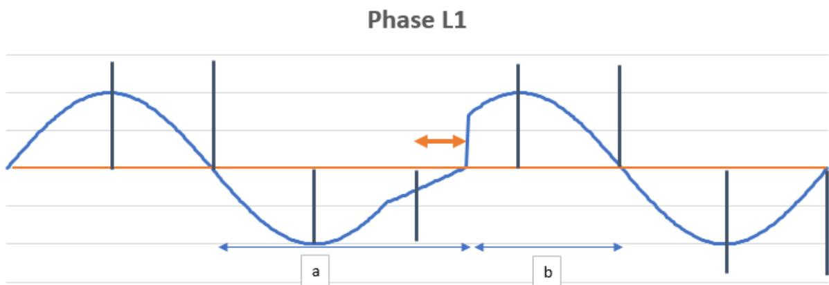
**Figure 10:** How the zero-crossing can have an offset during the ramp.
