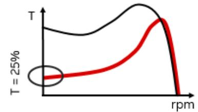
**Figure 3:** Torque during ramp with softstarter (red) and DOL (black).
