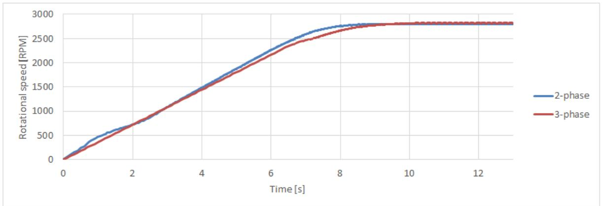
**Figure 19:** Rotational speed over time with torque ramp with a light load for both 2- and 3-phase controlled softstarters with the same acceleration times. The ramps are equally good: shape profile and acceleration time coincides.
