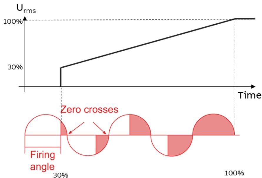
**Figure 6:** RMS voltage and thyristor triggering process relative to 50/60 Hz sine wave during softstarter starting sequence.
