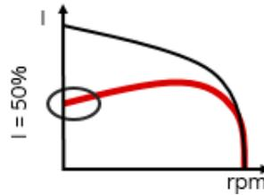
**Figure 2:** Current during start with (red) softstarter and DOL (black).
