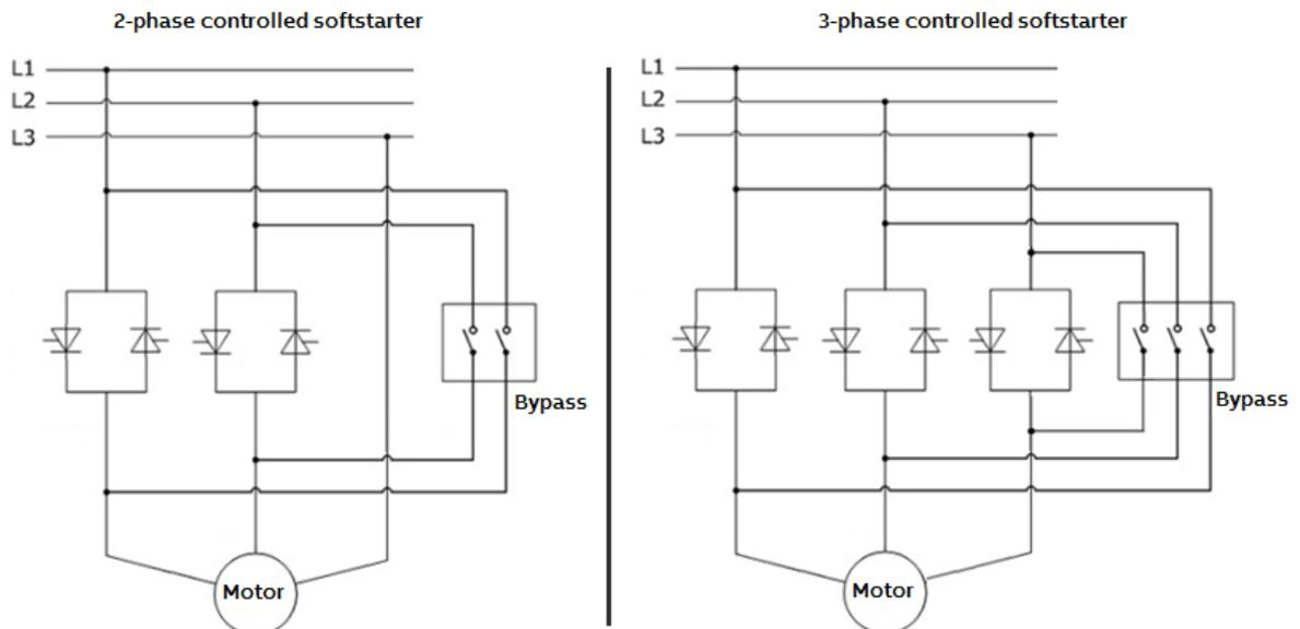
**Figure 21:** Softstarter main circuit topology comparison between 2- and 3-phase controlled softstarters. To the left two phases can be controlled with the thyristors and the bypass, where the third phase is connected directly to the motor. To the right, all phases can be controlled with thyristors and bypass.
