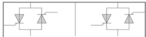
**Figure 5:** Thyristor topology of a "2-phase softstarter": 2 sets of anti-parallel thyristors.
