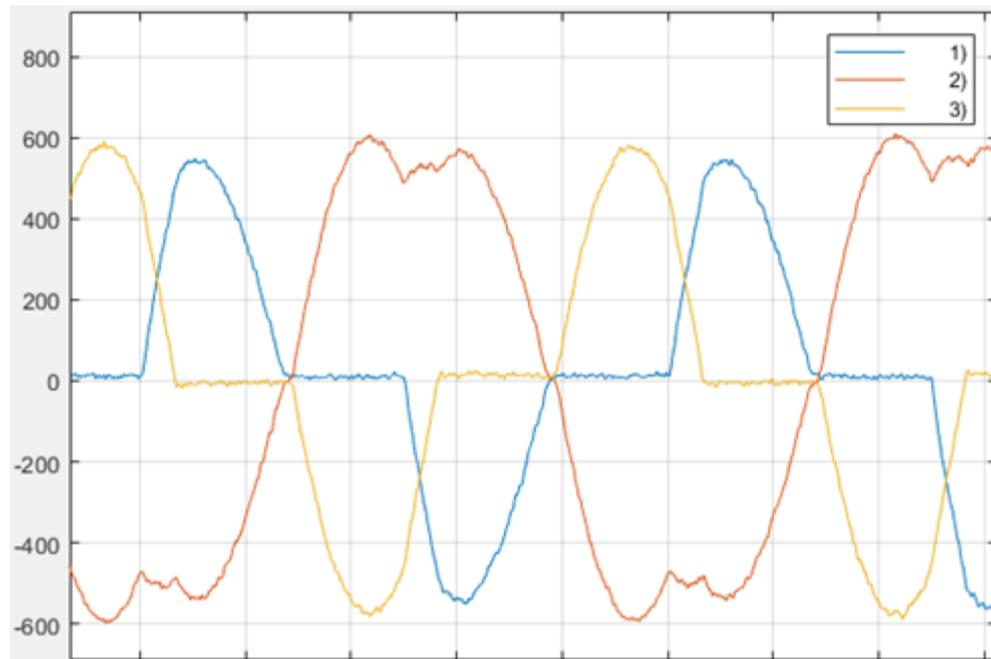
**Figure 9:** The three phase currents when triggering angle is 5 ms. The distance between vertical lines represent 4 ms.
