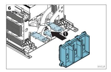
7. Fasten screws to bottom bar holder 1 Fasten (2x) () Torx 30 M6x16 (8Nm) to the lower corners of the bar holder. 2 Fasten (6x) Torx 30 M6x16 (8Nm) to attach the bar holder to the phase bars.
