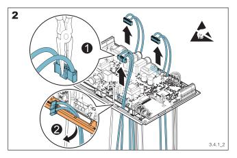
terminal on the PCBA using a long-nose plier.
