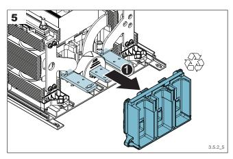
6. Place new bottom side bar holderPlace the new bar holder onto phase bars.
