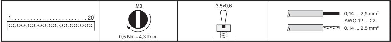
Figure 23: Tightening torques and cable dimensions (1 mm=0.0394 in)
