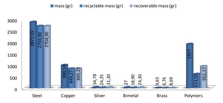
The recyclability and recoverability rate has been calculated based on the guidelines of the IEC/TR 62635 Edition 1.0 (2012-10-19)
