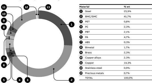
Tmax XT2 with thermal-magnetic release. The total weight of the product is 1.251 gr. Tmax XT3 with thermal-magnetic release. The total weight of the product is 1.471 gr.
