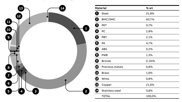
Tmax XT5 with thermal-magnetic release. The total weight of the product is 4.198 gr.
