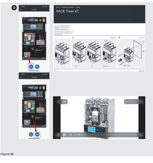
QR Code The new QR code function developed for EPiC allows the user to scan the QR code and obtain further useful information about the scanned circuit-breaker.
