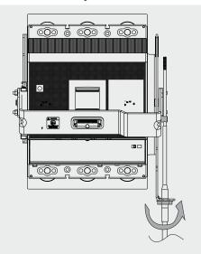
Ensure gap between Edge Guard and Breaker Handle as shown before inserting the Drive Pin into the hole of Yoke.
