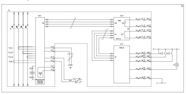
PR222DS/PD, PR223DS electronic trip unit connected with the AUX-E auxiliary contacts
