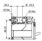
Front for copper/aluminium cables - FC CuAl 2x240 mm<sup>2</sup>
