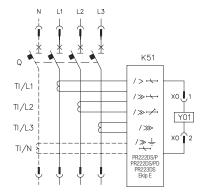
Three-pole or four-pole circuit-breaker with PR222DS/P, PR222DS/PD, PR223DS, or Ekip E electronic trip unit for T4, T5 and T6 (PR222DS/PD for T5 and T6 only)
