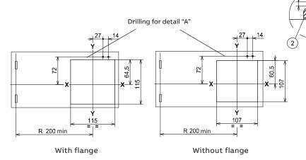
Drilling template for support sheet
