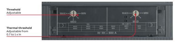
TMA = thermomagnetic trip unit with adjustable thermal threshold ( $I_1 = 0.7...1 \times In$ ) and adjustable magnetic threshold ( $I_3 = 5...10 \times In$ ) \*T4N/PV-E is only available with TMF trip unit (both thermal and magnetic thresholds are fixed)
