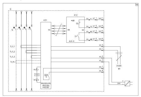
PR222DS/PD, PR223DS electronic trip unit connected with the AUX-E auxiliary contacts and the MOE-E actuation unit
