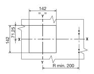
Drilling template for support sheet
