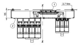
Drilling templates for fixing the circuit-breaker on the support sheet
