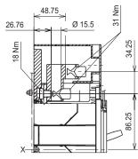
Front for copper/aluminum cables -FC CuAl 1x240 mm<sup>2</sup>
