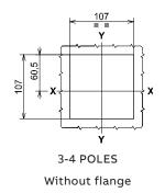
Drilling templates for support sheet
