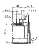
Front for copper/aluminium cables - FC CuAl 4x150 mm<sup>2</sup>
