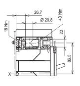
Front for copper/aluminium cables - FC CuAl 300 mm<sup>2</sup>
