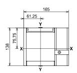
Drilling template for compartment door and fitting flange
