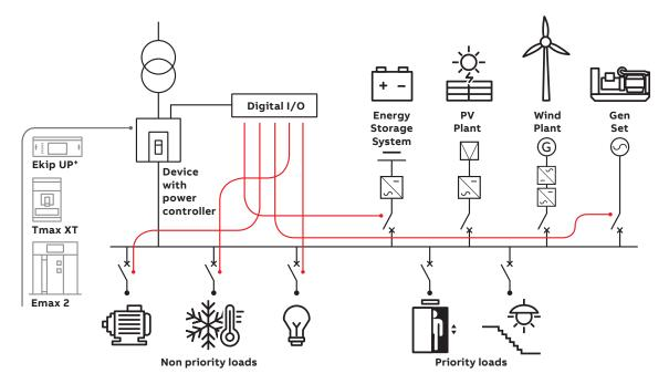
Ekip Power Controller is a function that drives peak shaving by managing different loads and generators. It represents an optimum compromise between reliability, simplicity and cost-effectiveness. This function is embedded on request in the Ekip electronic trip unit and avoids complex control systems and implementation of dedicated software programs.
