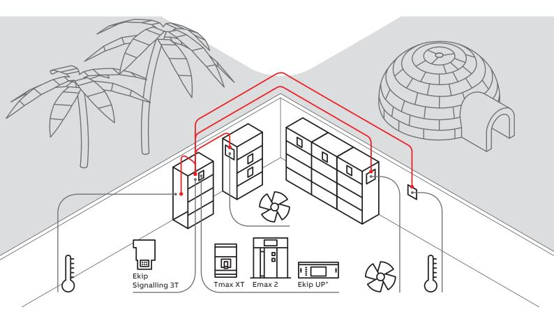
01 Ekip Signalling 3T Understanding and monitoring environmental parameters is the key to prevent system failures or other unsafe conditions.
