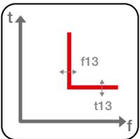
**Overfrequency (OF - ANSI 81H):** with constant trip time ( $t = k$ ), function is tripped when network frequency exceeds the set threshold.
