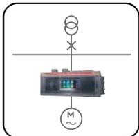
**Reverse active power (RP - ANSI 32R):** with constant trip time ( $t = k$ ), function is tripped when total active power – in the opposite direction of the current - exceeds the set threshold.
