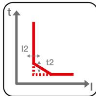
**Time-delayed overcurrent (S - ANSI 51 & 50TD):** with constant tripping time ( $t = k$ ), or with constant specific let-through energy ( $t = k/I^2$ ), this provides 15 current thresholds and 8 curves, for fine adjustment.
