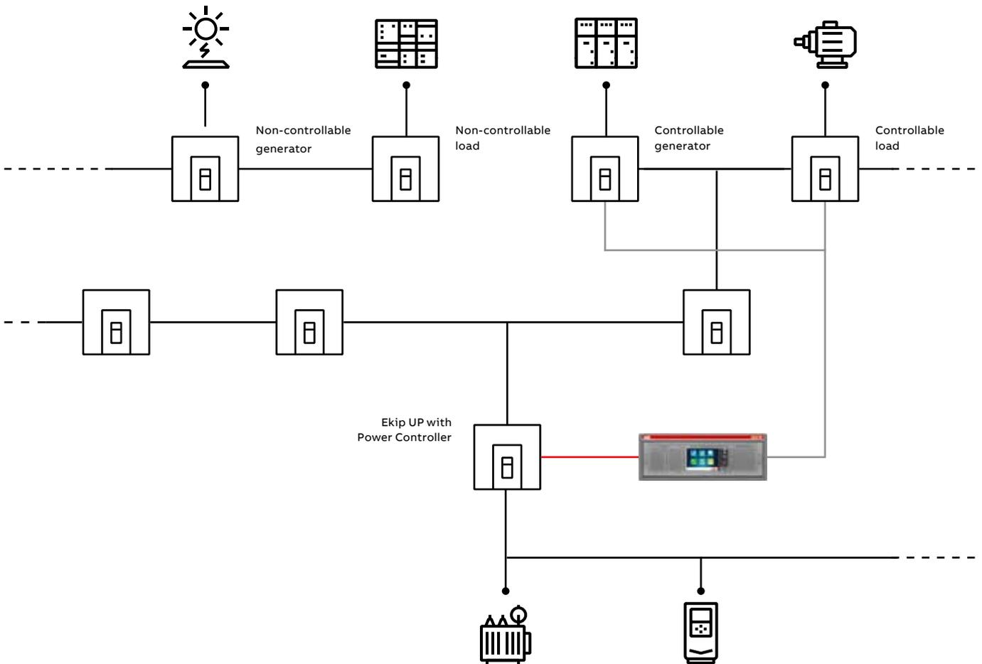
In installations that are already equipped with energy management systems, the load limit can be controlled remotely. OpenADR communication standards (see Chapter 4) provides another way to receive power set-points from load aggregators or utilities.
