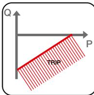
**Loss of field or reverse reactive power (RQ – ANSI 40 or 32RQ):** with constant trip time ( $t = k$ ), the switching device tripped when the total reactive power absorbed by the generator exceeds the set threshold. It is possible to select the constant threshold ( $k=0$ ) or a function of the delivered active power of the generator ( $k \neq 0$ ).
