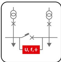
**Synchrocheck (SC - ANSI 25):** the synchronism control function compares the voltages in the modules as well as the frequencies and phases of two switching devices to which the switching device is connected. Ekip UP indicates that conditions have been reached also with display synchronism indicators that enable the two lines to be made parallel.
