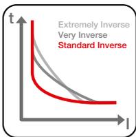
**Overload (L - ANSI 49):** available with three different types of trip curve:
