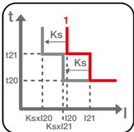
**Second protection against voltage controlled overcurrent protection (S2(V) - ANSI 51V):** available in addition to the protection S(V), enables total selectivity to be achieved in all installations.
