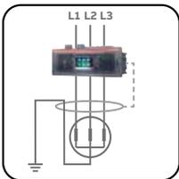
**Differential ground fault (Rc - ANSI 87N):** protects against internal earth fault on generator winding. It is required that the toroid hugs the active conductors and the ground conductor. Rc protection is integrated by a dedicated residual current rating plug and the external toroid.
