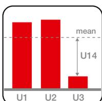
**Voltage unbalance (VU - ANSI 47):** with constant trip time ( $t = k$ ), protects against an unbalance between the voltages of the individual phases that are protected by the circuit-breaker.
