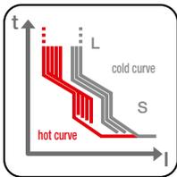
**Thermal memory:** for protections L and S it is used to protect the components, such as transformers, against overheating following overloads. The protection adjusts the trip time of the protection according to how much time has elapsed after the first overload, taking account of the overheating caused.
