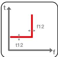
**Underfrequency (UF - ANSI 81L):** with constant trip time ( $t = k$ ), function is tripped when network frequency falls below set threshold.
