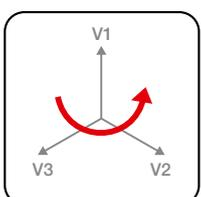
**Cyclical direction of the phases (ANSI 47):** indicates an alarm through inversion of the phases sequence.
