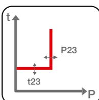
**Active underpower (UP – ANSI 32LF):** with constant trip time ( $t = k$ ), the function is tripped when the active power delivered by the generator is lower than the set threshold. It is possible to disable the protection temporarily, to manage the start-up phase, by setting a time window from the closing of the switching device, by using an electrical signal or via incoming communication to a relay.
