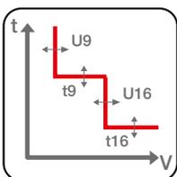
**Second protection against undervoltage and overvoltage (UV2 and OV2 – ANSI 27 and 59):** enables two minimum and maximum voltage thresholds to be set with different delays in order to be able to discriminate, for example, between voltage dip transients due to the start-up of a motor and an actual fault.
