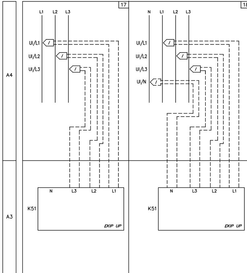
**19A) Bridges for Ekip UP without current connections**
