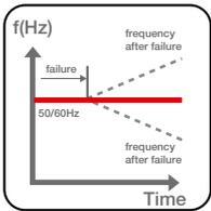
**Rate of change of frequency (ROCOF – ANSI 81R):** enables both positive and negative frequency variations to be rapidly detected. The protection is constant and is tripped when the frequency variation in Hz/s is greater than the set threshold.
