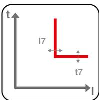
**Current unbalance (IU - ANSI 46):** with constant trip time ( $t = k$ ), protects from an unbalance between the currents of the single phases protected by the switching device.
