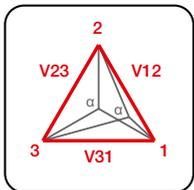
**Residual overvoltage (RV – ANSI 59N):** with constant trip time ( $t = k$ ), protects against insulation loss in systems with insulated neutral or with neutral earthed with impedance.
