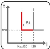
**Voltage controlled overcurrent protection (S(V) - ANSI 51V):** protection from maximum current with a constant trip time ( $t = k$ ) that is sensitive to the voltage value. The set current threshold, following a voltage drop, decreases by steps or linearly.
