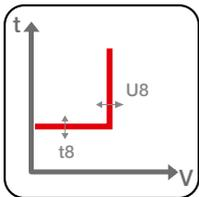
**Undervoltage (UV - ANSI 27):** with constant trip time ( $t = k$ ), function is tripped when phase voltage falls below set threshold.
