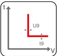
**Overvoltage (OV - ANSI 59):** with constant trip time ( $t = k$ ), function is tripped when phase voltage exceeds the set threshold.
