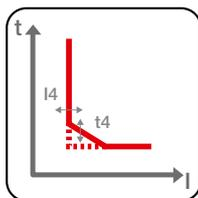
**Earth fault (G - ANSI 51N & 50NTD):** with trip time independent of the current ( $t = k$ ) or with constant specific let-through energy ( $t = k/I^2$ ). A pre-alarm indication is also available when 90% of the threshold is reached to activate corrective measures before the protection is tripped. The function also enables the trip to be excluded so that only the alarm is indicated, for use in installations where continuity of service is an essential requirement.
