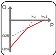
**Second protection against loss of field or reverse reactive power (RQ – ANSI 40 or 32R):** enables the generator’s de-energization curve to be followed very accurately, thereby avoiding any unnecessary disconnection.
