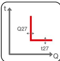
**Reactive overpower (OQ – ANSI 32OF):** with constant trip time ( $t = k$ ), the function is tripped when reactive power exceeds the set threshold in the generator to network direction.
