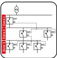
**Zone selectivity for S and G protection (ANSI 68):** can be used to minimize circuit-breaker trip times closer to the fault. The protection is provided by connecting all the zone selectivity outputs of the trip units belonging to the same zone and taking this signal to the trip unit input that is immediately upstream.
