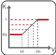
On the other hand, in linear mode (restrained mode) two voltage limits are selected within which the protection is tripped at the set threshold ( $I_{20}$ ) reduced by the factor  $K$  corresponding to the measured voltage. The variation of the factor  $K$  is proportional to the voltage, and for voltages greater than the upper threshold ( $U_h$ ) the threshold  $I_{20}$  works, whereas for voltages below the lower threshold ( $U_l$ ) the minimum threshold ( $I_{20} * K_s$ ) applies.
