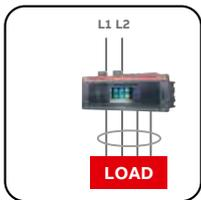
**Residual current (Rc – ANSI 64 & 50NDT):** with constant temperature ( $t=k$ ) protects against indirect contacts and is integrated into Ekip UP Protect and Ekip UP Protect+ by a dedicated residual current rating plug and external toroid. The protection is an alternative to the functions G and Gext and it is activated by dedicated rating plugs.
