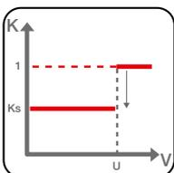
In step mode (controlled mode) the protection is tripped at the set threshold ( $I_{20}$ ) if the voltage is above  $U$ , whereas it is tripped at the lower threshold of the factor  $K_s$  ( $I_{20} * K_s$ ) if the voltage is below  $U$ .
