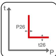
**Active overpower (OP – ANSI 32OF):** with constant trip time ( $t = k$ ), the function is tripped when the active power exceeds the threshold set in the delivering direction of the generator.
