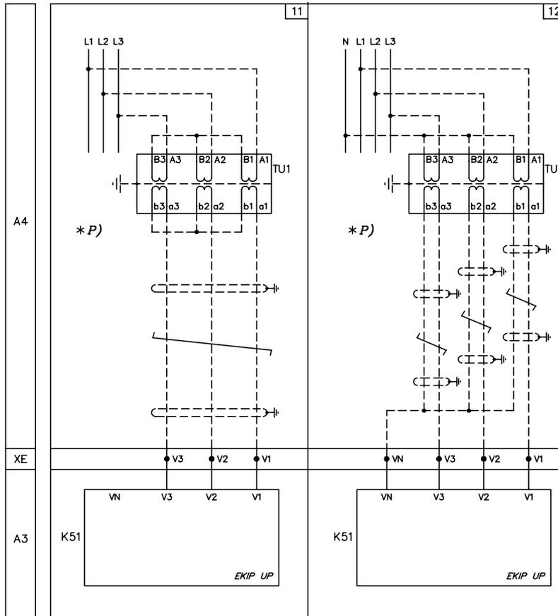
**13) Ekip UP without external voltage transformer and 3P configuration**
