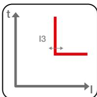
**Instantaneous overcurrent (I - ANSI 50):** with trip curve without intentional delay, it offers 15 tripping thresholds.
