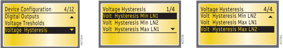
Figure 7.32 Voltage Hysteresis (min and max) settings for Line 1 and Line 2
