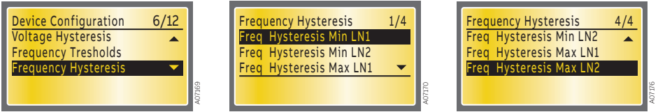
Figure 7.37 Frequency Hysteresis (min and max) settings for Line 1 and Line 2
