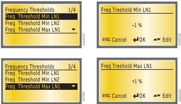
Figure 7.36 Frequency Threshold LN1, factory settings: min -1%, max 1%
