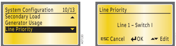
Figure 7.19 Line Priority, Line 1 - Switch I is the default
