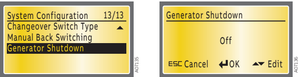
Figure 7.22 Generator Shutdown, Off is the default
