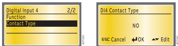
Figure 7.26 Digital Input 4 – Contact Type, NO is the default
