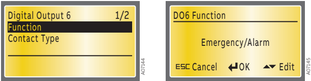
Figure 7.28 Digital Output 6 - Function, Emergency/Alarm is the default
