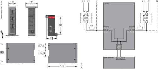
Picture 5. Dimensions of the device
