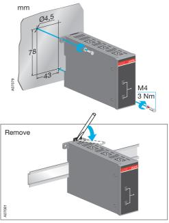
Picture 3. Drilling hole distances/screw mounting
