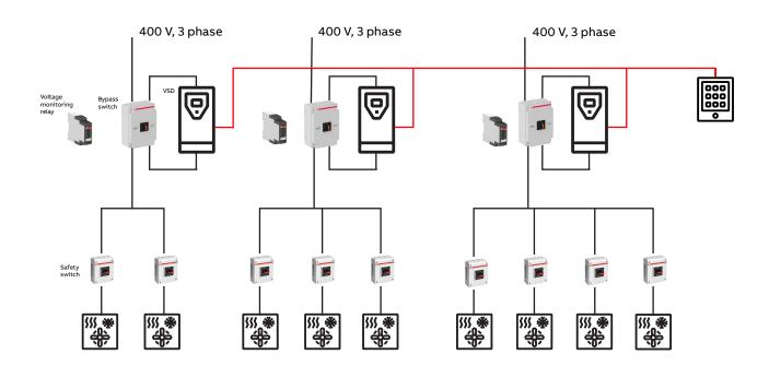
$Application\ example:\ ventilation\ system\ with\ variable\ speed\ drives,\ including\ by pass\ switches\ and\ voltage\ monitoring\ relays.$
