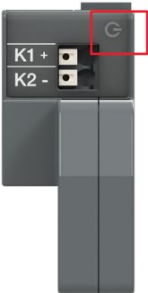
Fig. 5.8 Signals of auxiliary power supply module OXEA1
