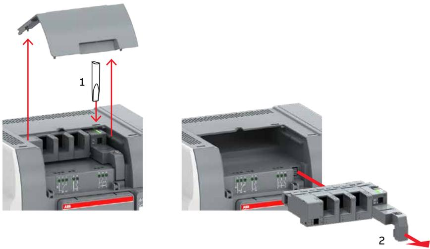
Fig. 9.7 Removing the auxiliary power supply module OXE1 and Ekip –modules from the automatic transfer switch
