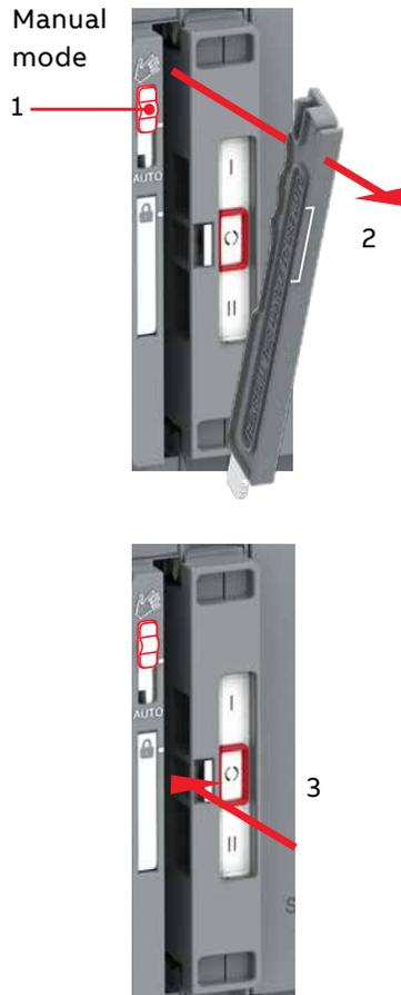
Fig. 8.11 Mounting the handle to the operating position; turn the slide switch to the Manual mode (Hand), lift the handle and place it to the operating position
