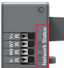
Fig. 5.21 Signals of Ekip Com DeviceNet -module
