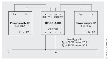
True redundancy using a CP-C.1-A-RU redundancy unit
