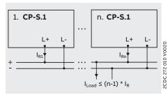
Parallel operation, redundancy (n  $\leq$  3)
