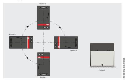
In order to ensure a sufficient convection in mounting position 1, the minimum distance to other modules must not be less than 50 mm in vertical direction and 30 mm in horizontal direction. For the derating of the output current, see the characteristic curve of temperature. Details for other mounting positions on request.
