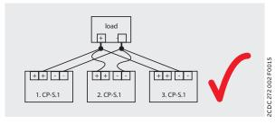
Correct wiring for increased power
