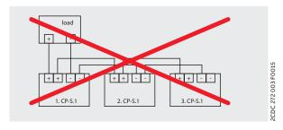
Incorrect wiring for increased power
