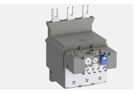
ABB's TF140DU thermal overload relays are economic electromechanical protection devices for the main circuit. They are used mainly to protect motors against overload and phase failures. Starter combinations are setup together with contactors.
