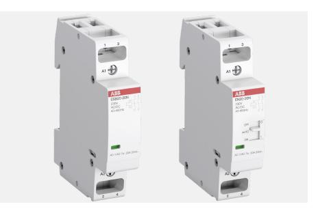
ABB's ESB..N installation contactors are premium electromechanical switching devices widely used for controlling lighting, heating, ventilation, motors and pumps. The range covers ratings up to 100 A, includes various accessories and is fully compatible with other modular DIN-rail components.
