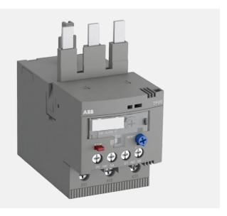
ABB's TF65 thermal overload relays are economic electromechanical protection devices for the main circuit. They are used mainly to protect motors against overload and phase failures. Starter combinations are setup together with contactors.
