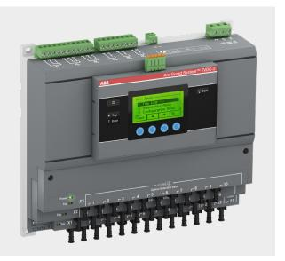
When an arc flash occurs, TVOC-2 with the system breakers cuts the power before the energy can increase. The arc flash is detected by the fiber optic sensor and a signal is sent to the TVOC-2 arc monitor. Finally, the TVOC-2 arc monitor sends a trip signal to trip the circuit breaker. All of this occurs in under 1 ms
