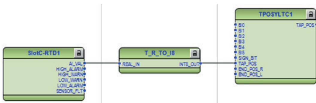
Figure 822: RTD/analog input configuration example
