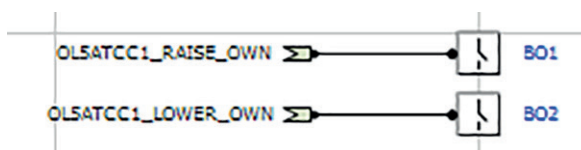
Figure 42: ACT diagram for transformer TR3 (Relay 3) in example case 2 – Output section
