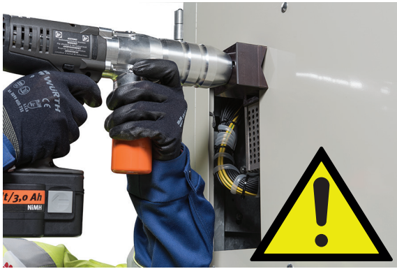
Figure 7: Cutting head in the starting position. Keep your hands away from the area where the cutting tool is used.
