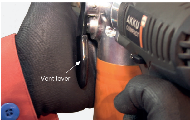
Figure 8: Pressing the vent lever
