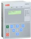
601 provides basic protection and control for feeder and motor applications. It is very compact, easy to install and engineer, having a built-in test function. The use is convenient with basic settings and an alphanumeric display. It has a very wide auxiliary voltage range with a universal power supply module, reducing the variants needed. The relay is offered with an optional galvanic communication module including several protocols.
