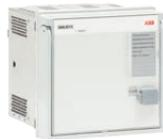
SMU615 is a dedicated substation merging unit intended for measuring current and voltage signals from the instrument transformers and merging them into the standard digital output format that other devices can further use for various power system protection application purposes. SMU615 itself includes no protection functionality but it offers the physical interface into the switchgear primary equipment, that is, circuit breaker, disconnector and earthing switch.
