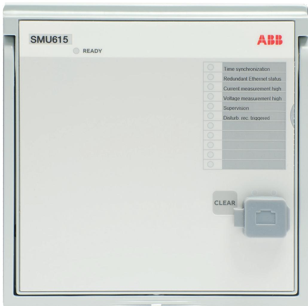
Figure 13: Programmable LEDs on the right side of the LHMI
