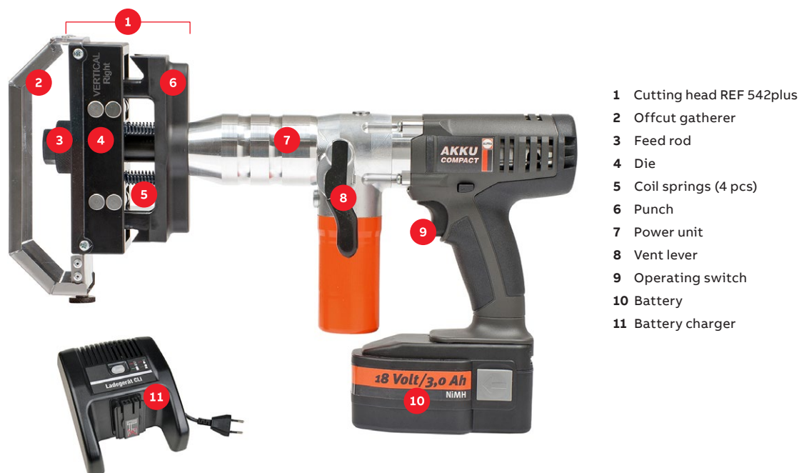
Figure 1: Cutting tool components
