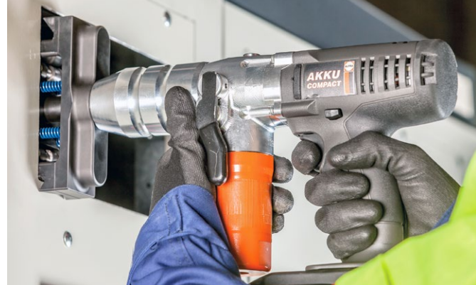
Figure 7: Cutting head in the starting position. Keep your hands away from the area where the cutting tool is in use.
