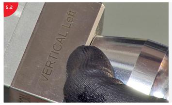
Ensure that the text on the cutting head, indicating the desired cutting direction, is facing you!
