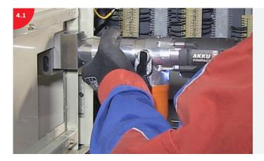
To cut horizontally, place the cutting head guiding against the top or bottom edge of the opening.
