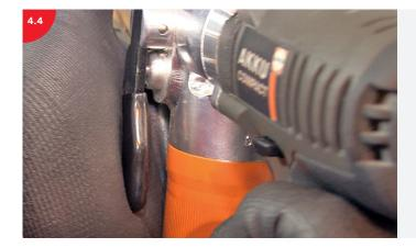
Push the vent lever to ensure that the punch is released after each cutting cycle.
