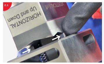
To set the cutting head for **horizontal** guiding: push the cutting head against the edges, as indicated with arrows in the image.
