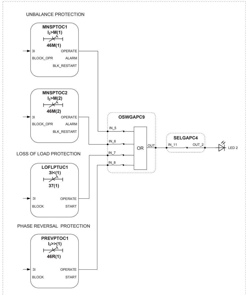
Figure 19: Unbalance, loss of load and phase reversal protection
