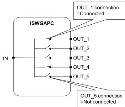
Figure 9: Input switch group ISWGAPC
