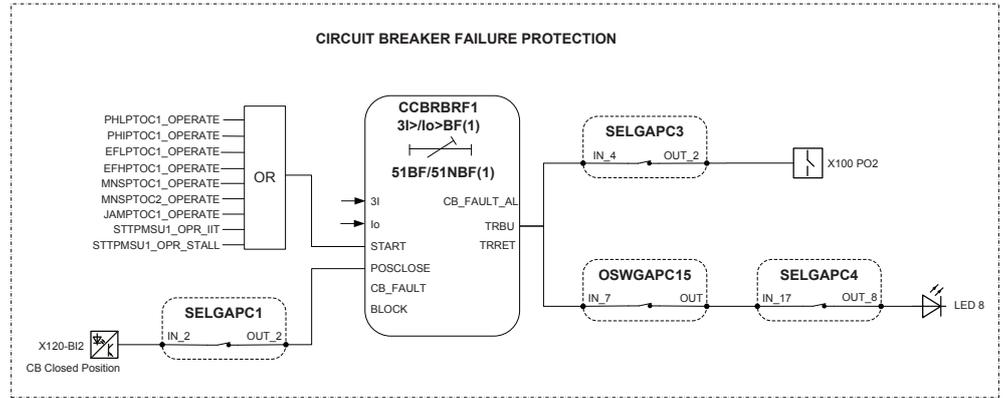
Figure 20: Circuit breaker failure protection
