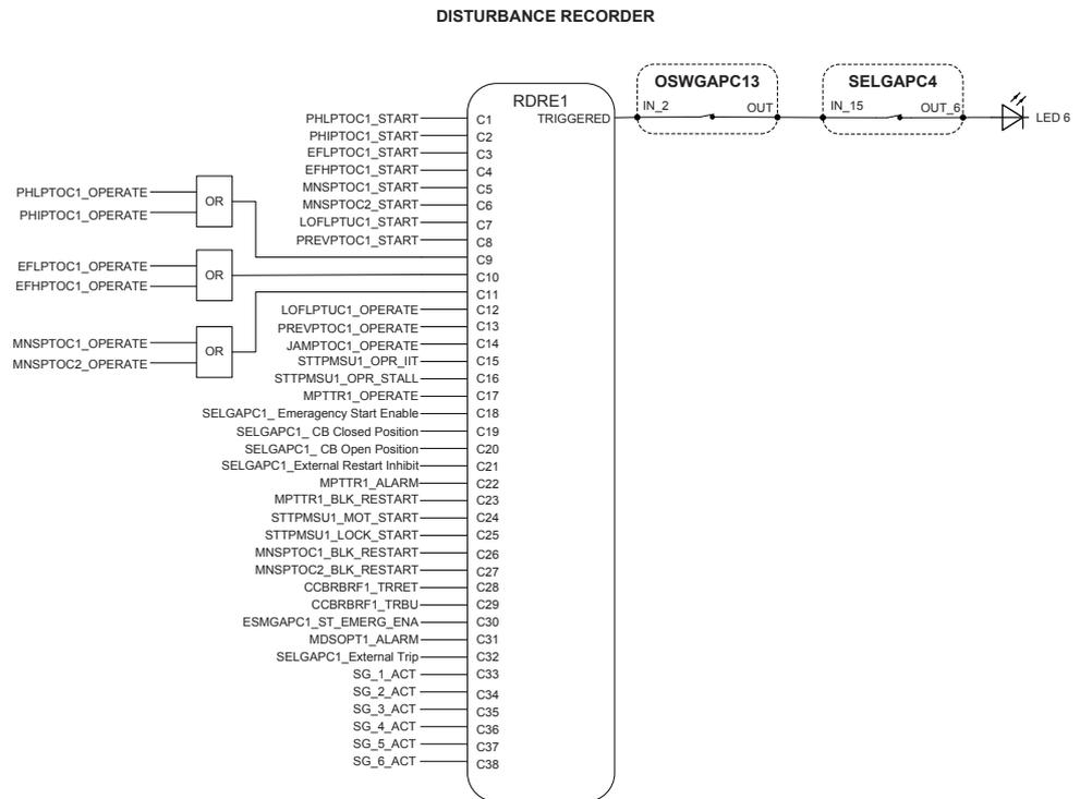
Figure 21: Disturbance recorder
