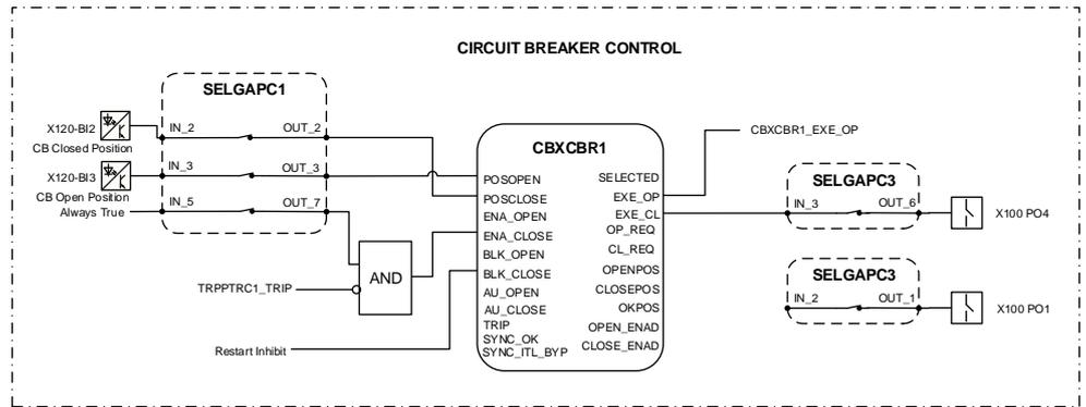
Figure 24: Circuit breaker control
