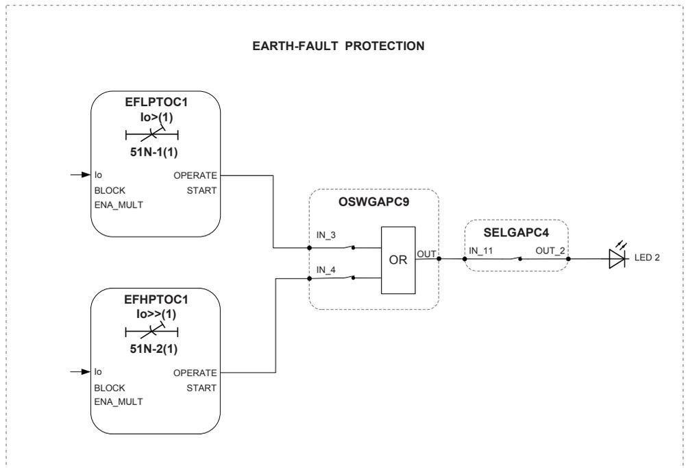
Figure 16: Earth-fault protection
