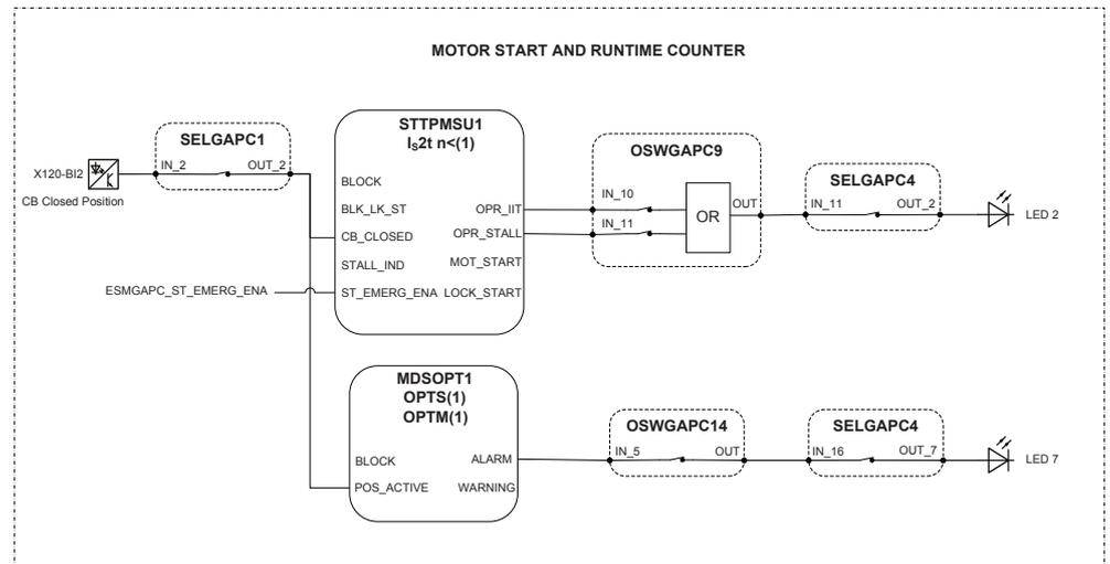
Figure 18: Motor startup supervision
