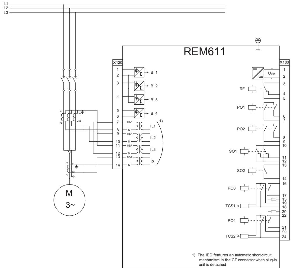
Figure 12: Connection diagram for configuration A when used with a circuit-breaker-controlled motor drive
