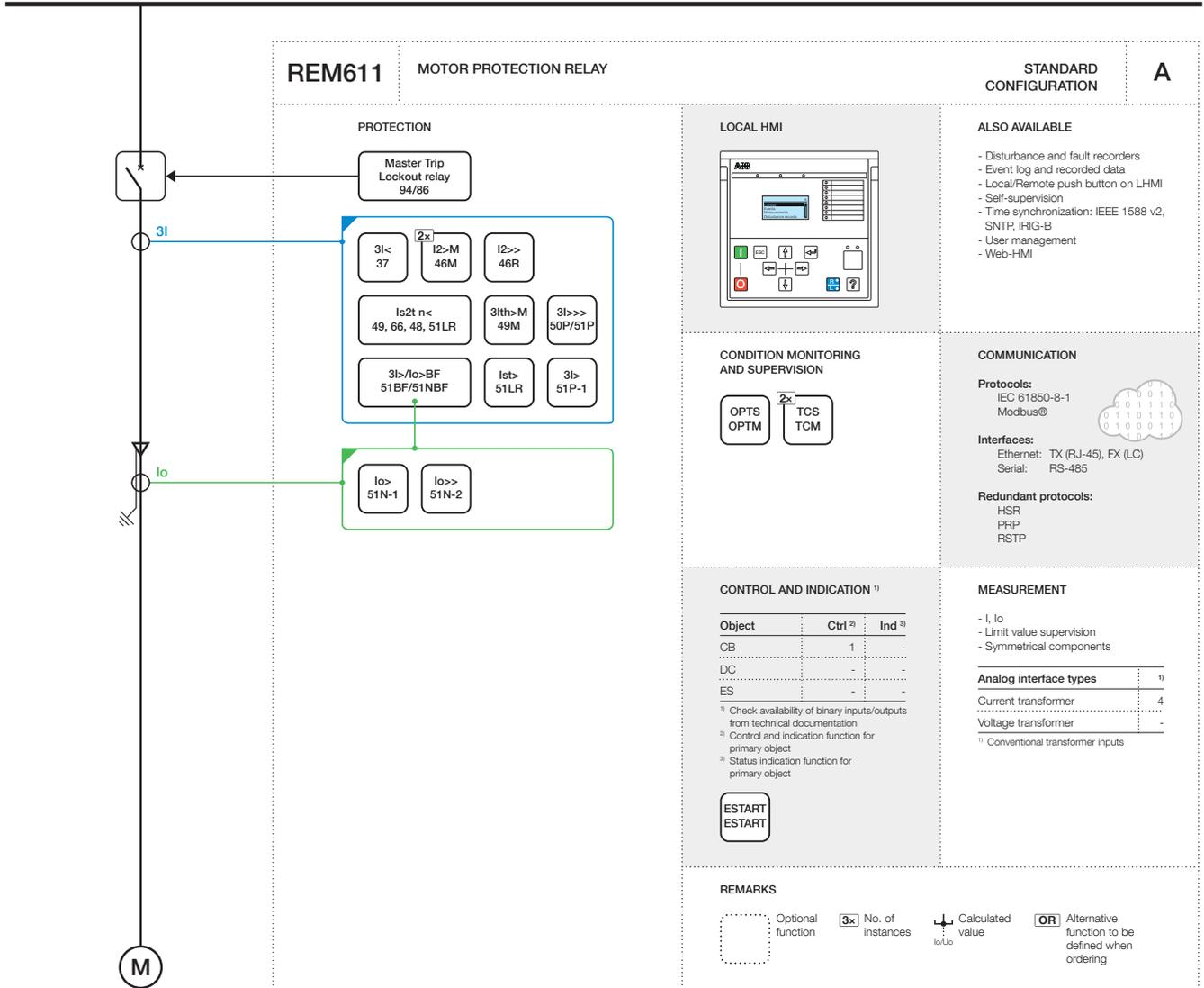
Figure 14: Functionality overview for configuration A
