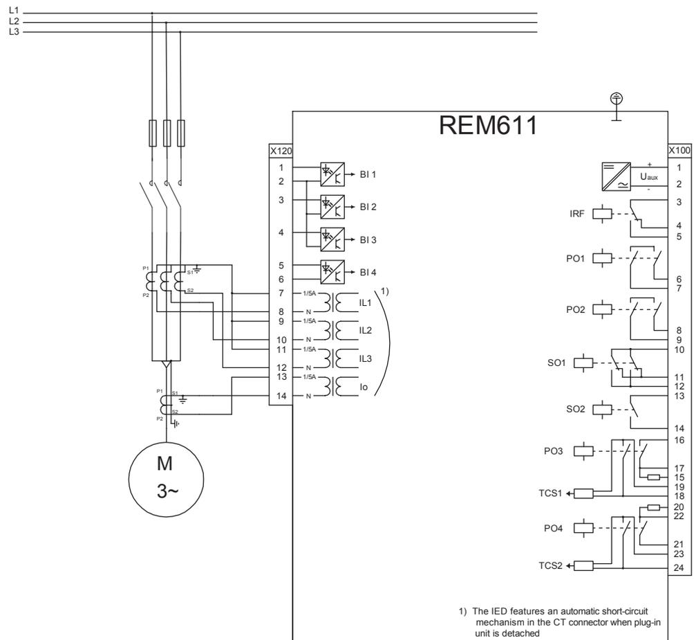
Figure 13: Connection diagram for configuration A when used with a contactor-controlled motor drive
