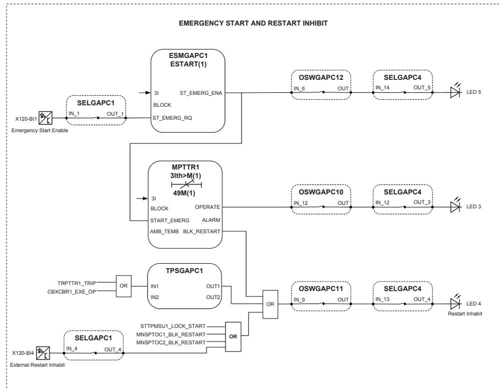
Figure 17: Emergency start and restart inhibit
