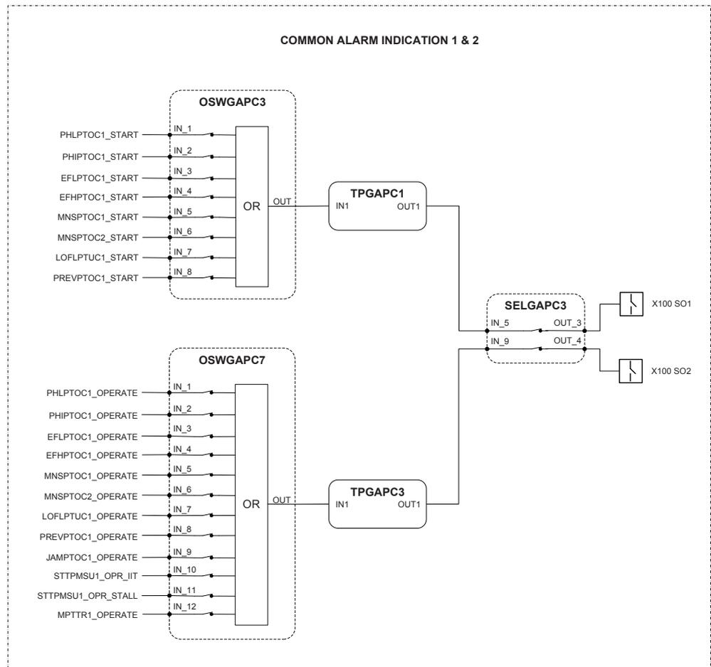
Figure 25: Common alarm indication
