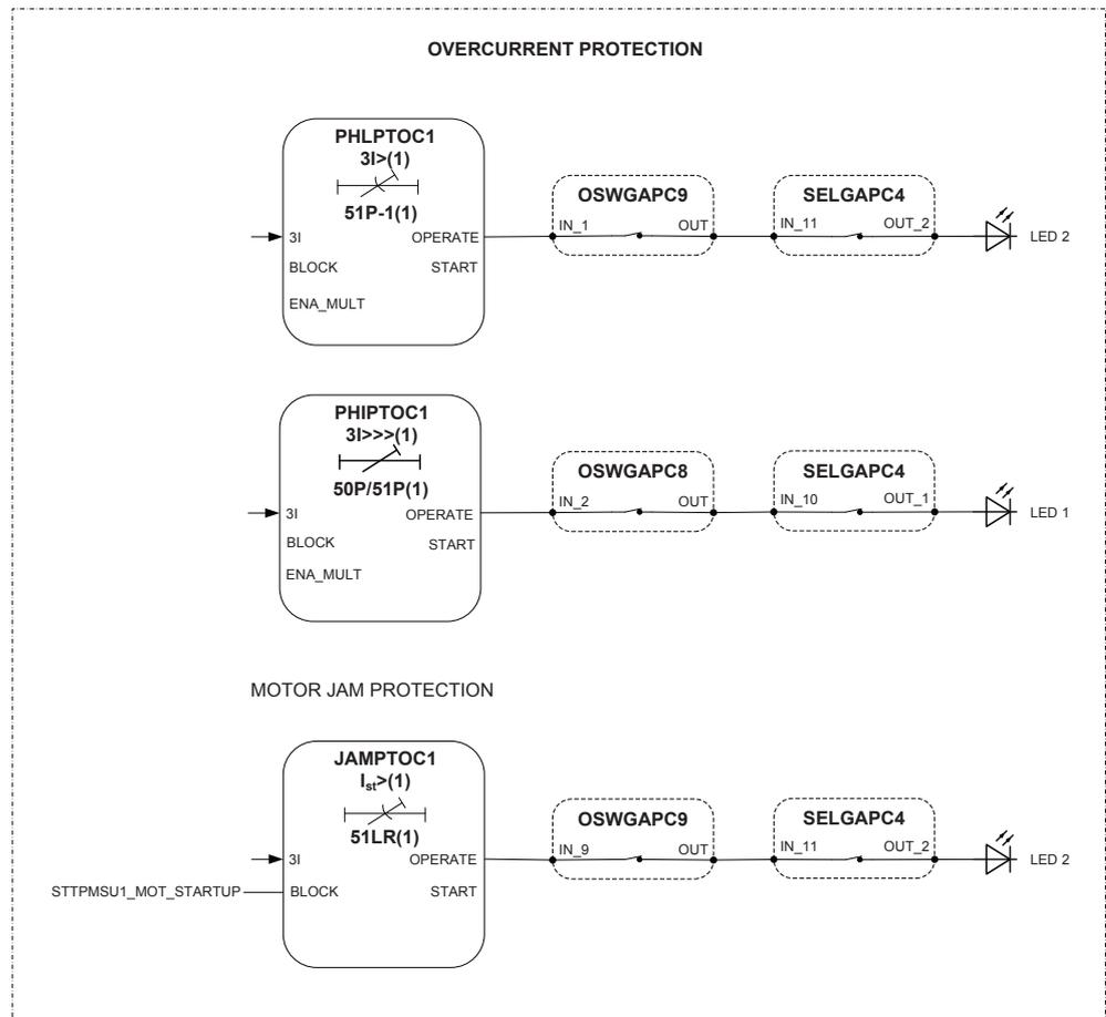
Figure 15: Overcurrent protection
