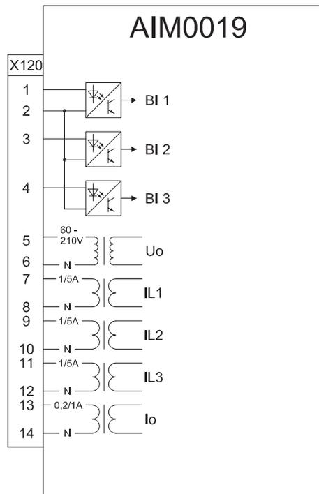
Figure 31: Example of AIM0019 card variant (4 I + Uo with 0.2/1 A Io channel)
