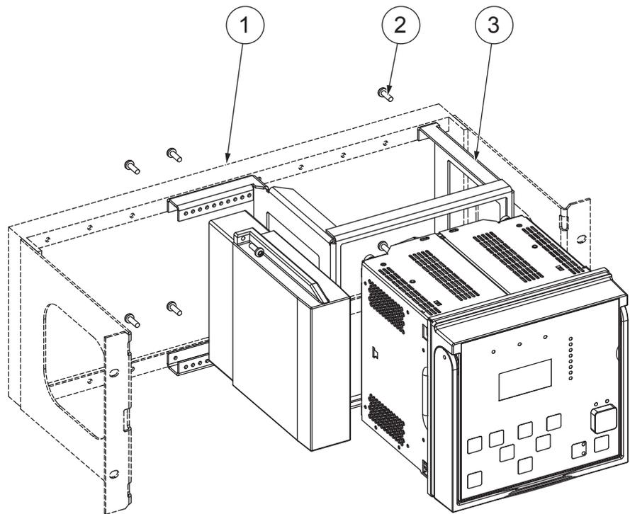
*Figure 23: Protection relay and the test switch*
