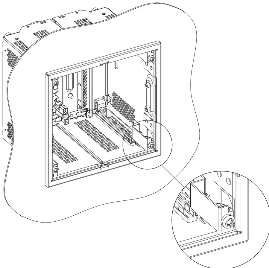
*Figure 8: Flush mounted case, tightening the M5 fixing screws*
