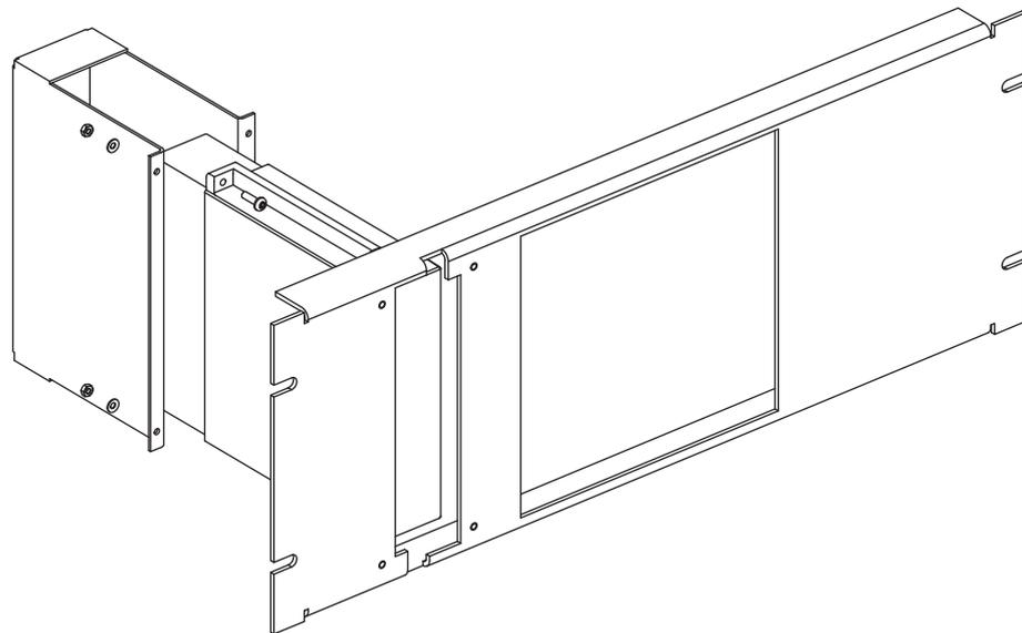
*Figure 20: Mounting of the metallic frame for an RTXP 18 test switch*
