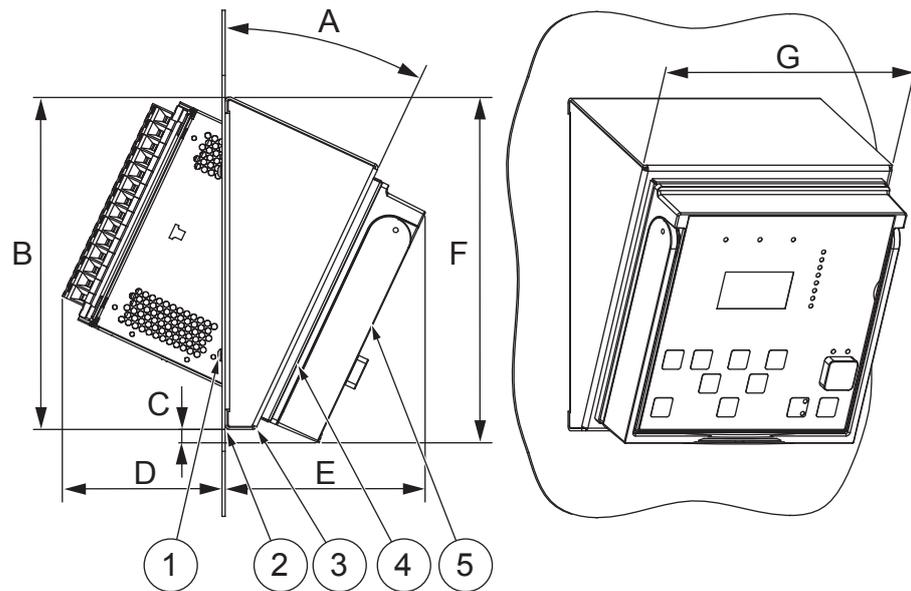
Figure 14: protection relay semi-flush mounted inclined
