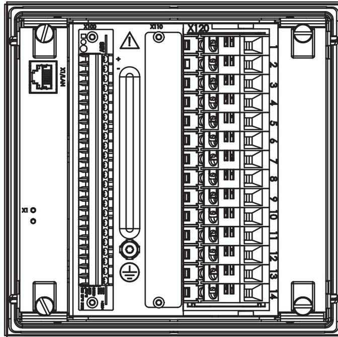
Figure 37: Rear view of a 611 series protection relay with communication module
