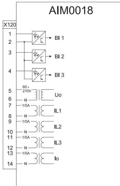
Figure 30: Example of AIM0018 card variant (4 I + Uo with 1/5 A Io channel)
