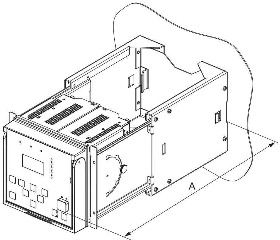
Figure 17: Wall mounting the protection relay
