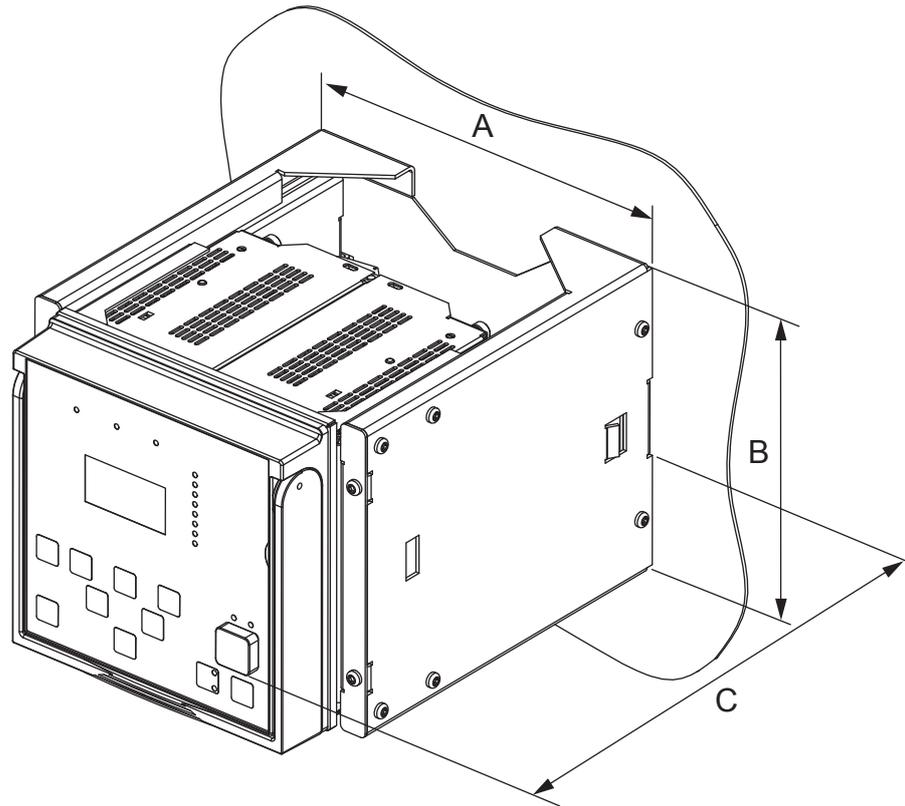
*Figure 18: Wall mounted protection relay*
