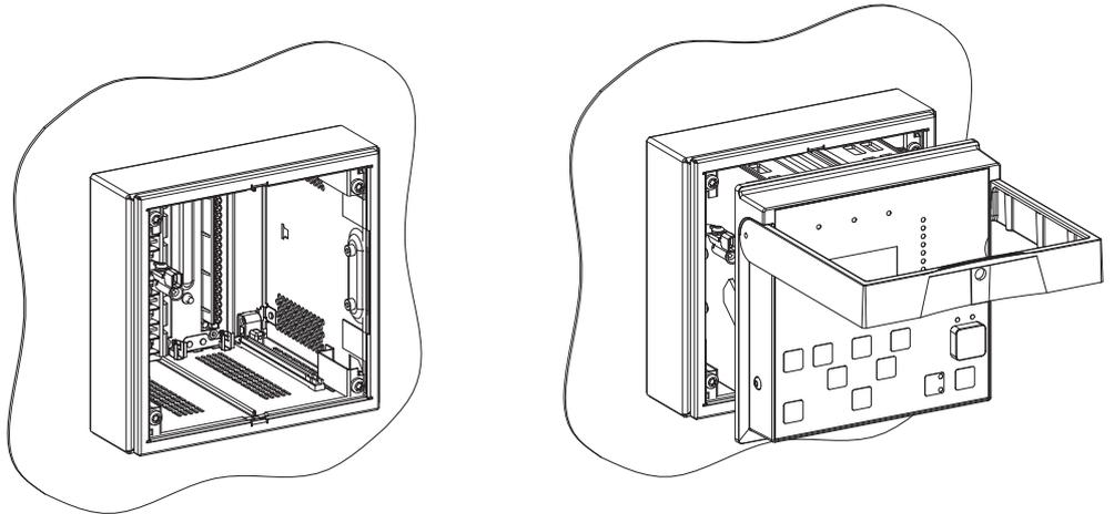
Figure 11: Mounting the case
