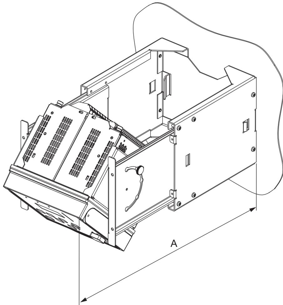
Figure 19: Wall mounted protection relay in rotated position
