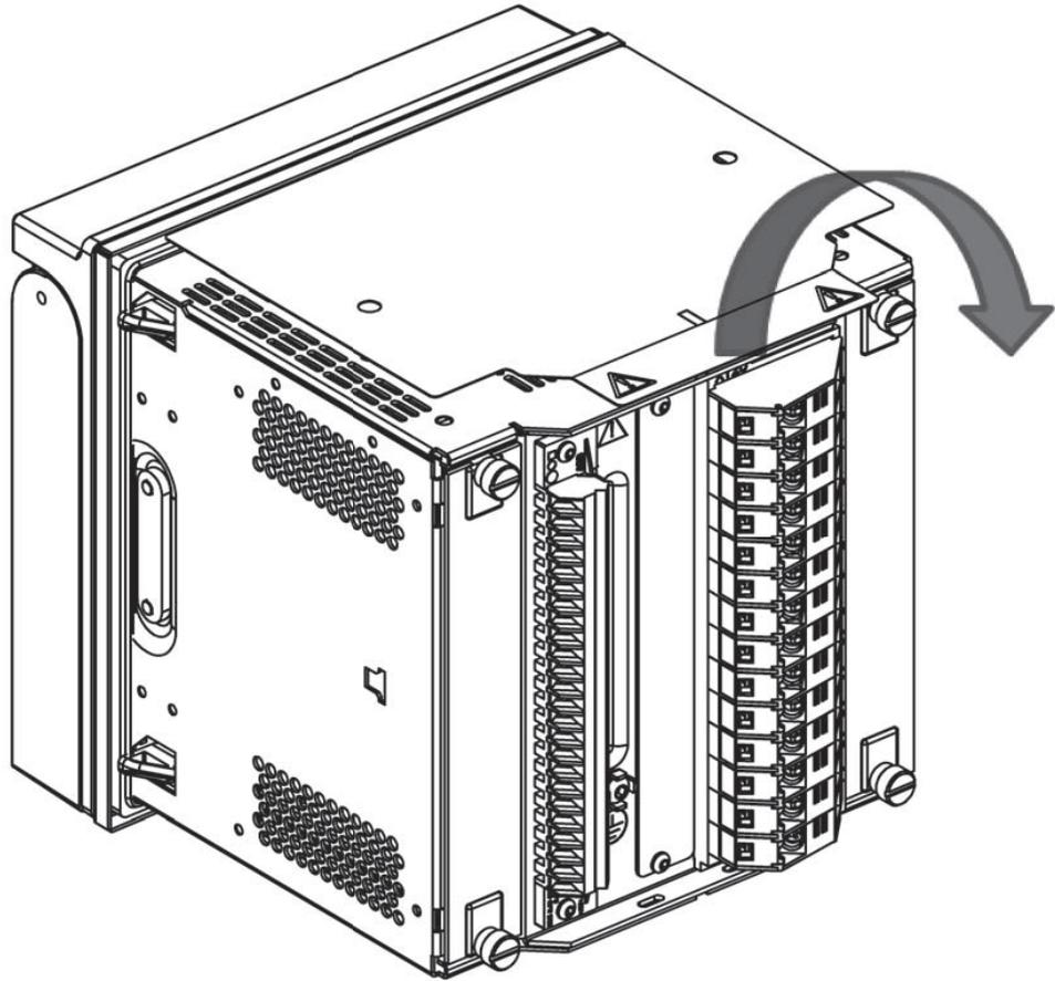
*Figure 34: Removing the protective film*
