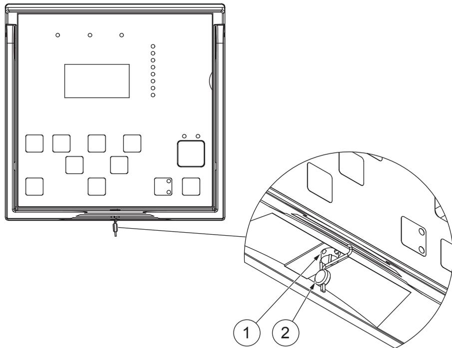
Figure 5: Sealing screw
