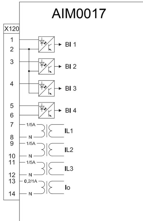
Figure 29: Example of AIM0017 card variant (4 I with 0.2/1 A Io channel)
