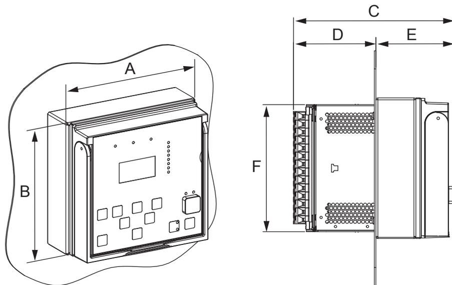
Figure 12: *Semi-flush mounted protection relay*
