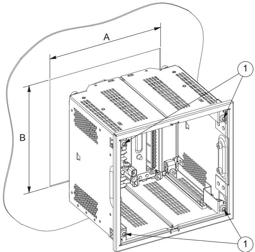
Figure 7: Flush mounting a case into a panel cut-out
