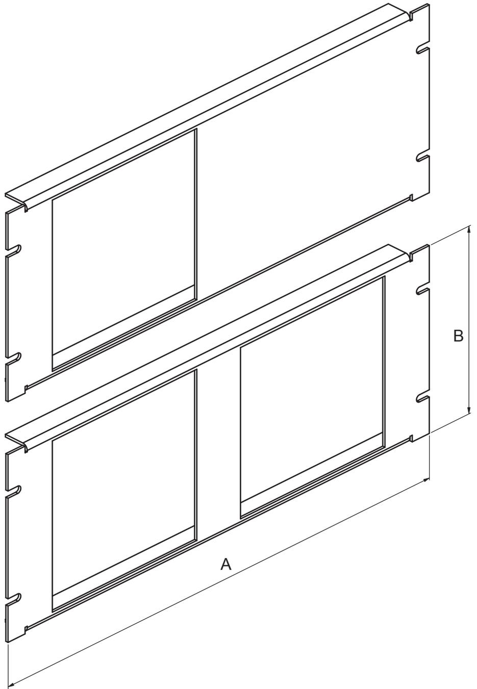
Figure 15: 19" rack mounting panels
