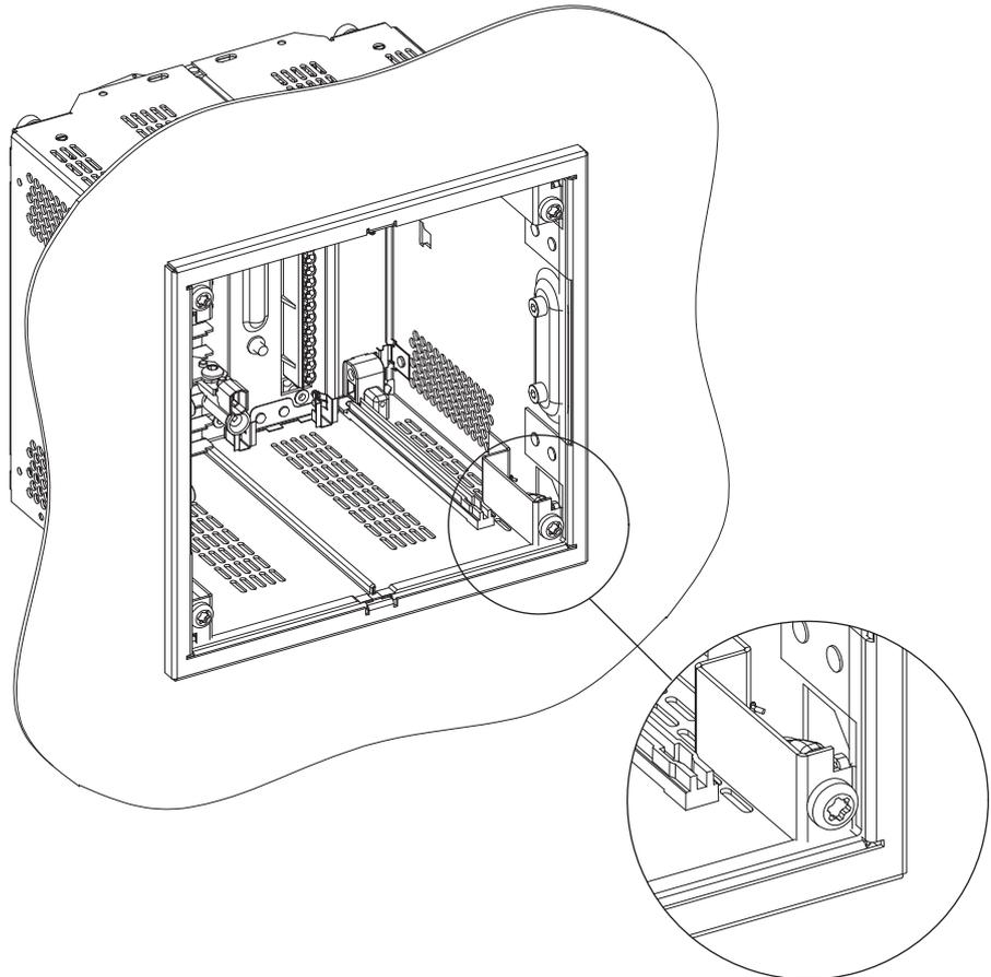
*Figure 35: Loosening the M5 screws*
