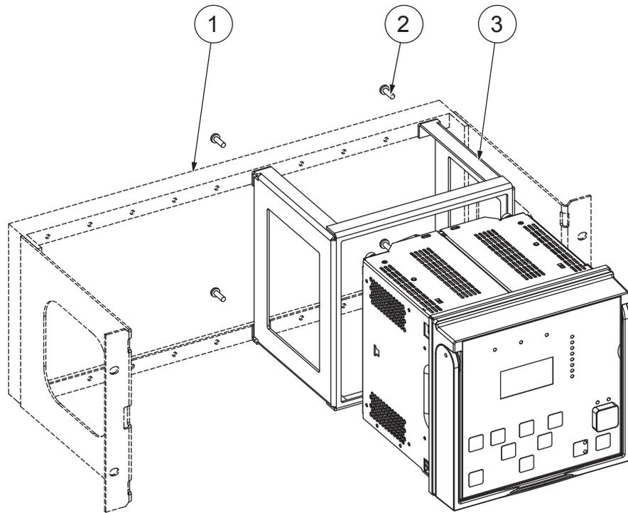
*Figure 22: Mounting the protection relay into a 19" combiflex equipment frame*
