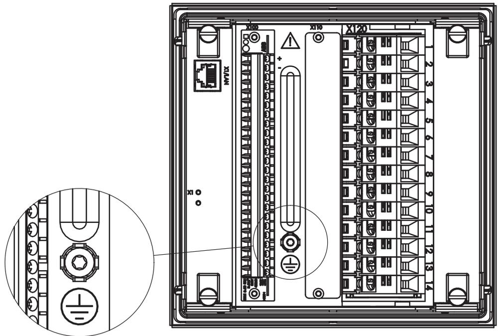
Figure 26: The protective earth screw is located between connectors X100 and X110
