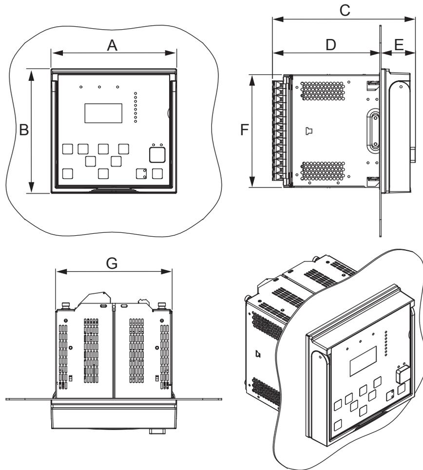
Figure 9: Flush mounted case and plug-in unit
