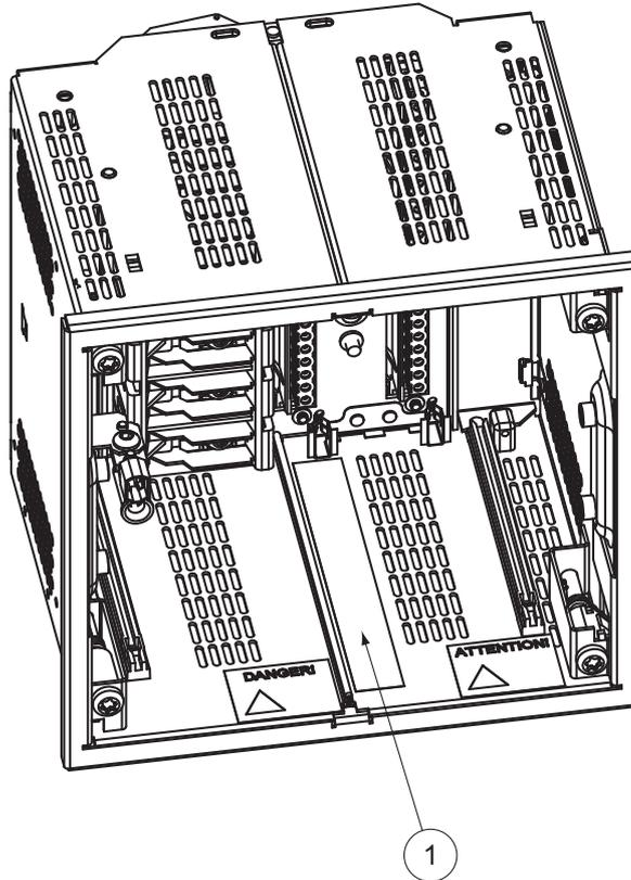
Figure 3: Serial number in the case
