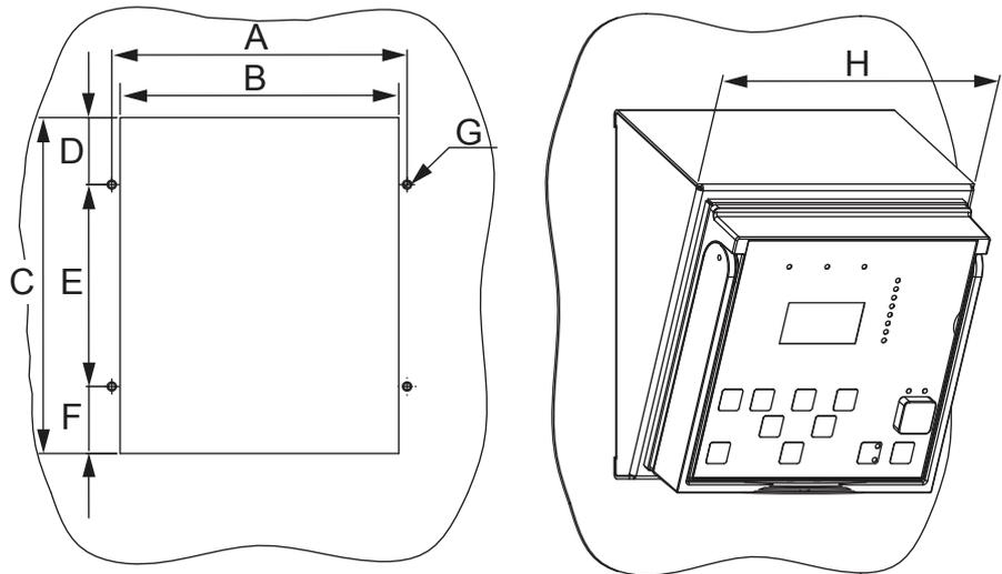
Figure 13: Mounting the angled frame
