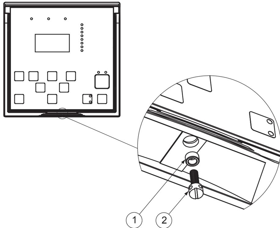
Figure 6: Sealing screw with spacer
