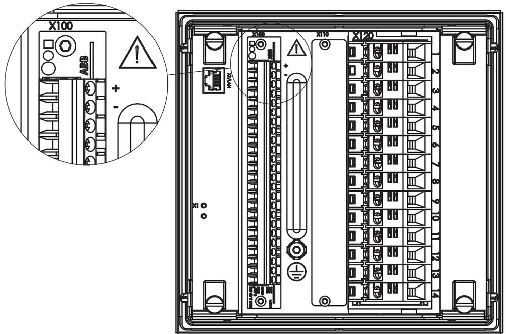
Figure 33: Connecting auxiliary voltage
