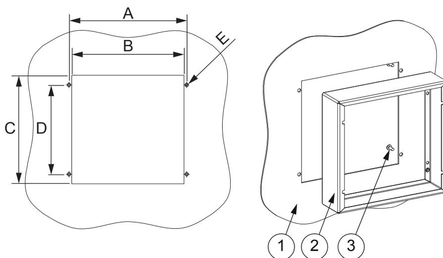
Figure 10: Mounting the raising frame
