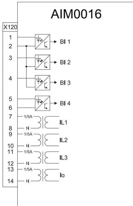
Figure 28: Example of AIM0016 card variant (4 I with 1/5 A Io channel)
