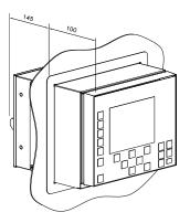
Figure 12. Semi-flush mounting
