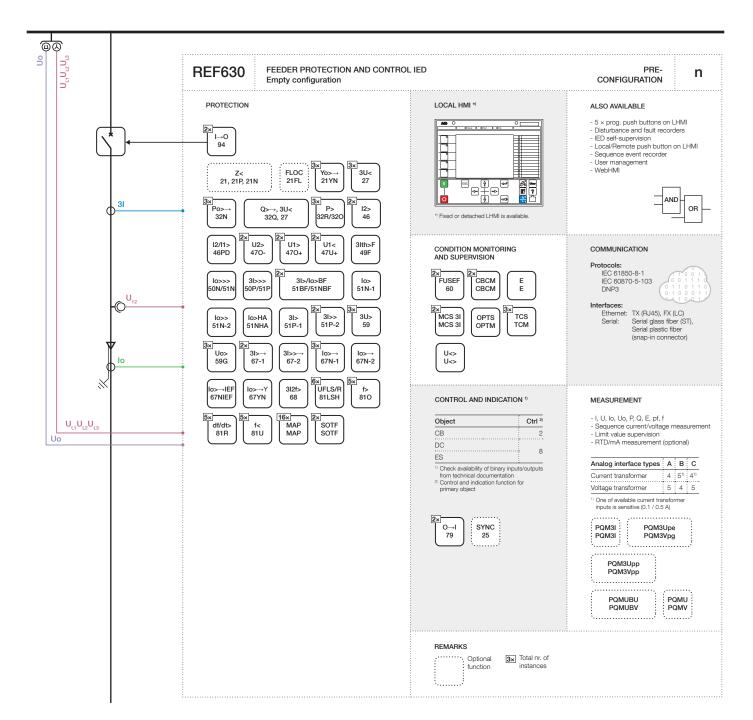
Figure 9. Functionality overview for preconfiguration n
