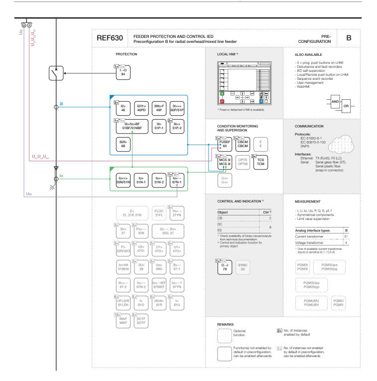
Figure 6. Functionality overview for preconfiguration B
