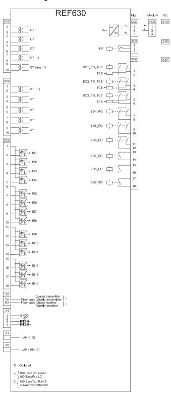
Figure 16. Terminal diagram for REF630
