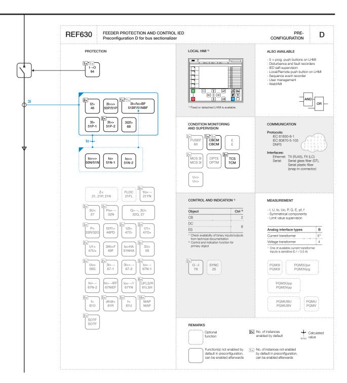
Figure 8. Functionality overview for preconfiguration D
