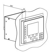
Figure 11. Flush mounting
