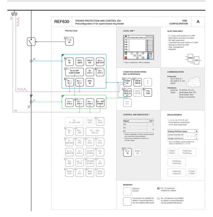
Figure 5. Functionality overview for preconfiguration A
