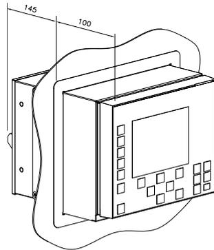
Figure 12. Semi-flush mounting
