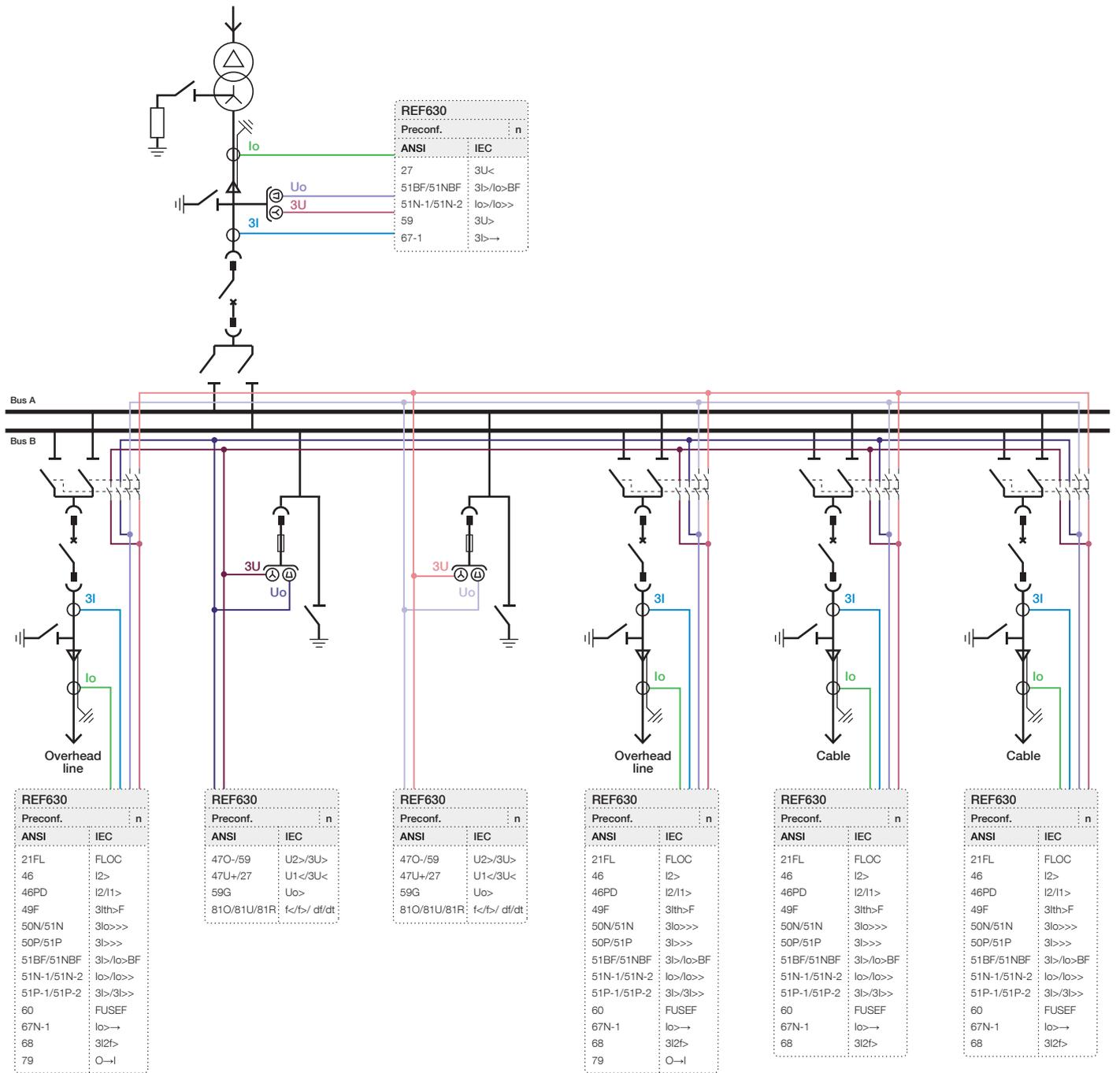
Figure 1. Application example with double busbar switchgear arrangement with one incoming feeder and several outgoing feeders for overhead line and cable feeders in preconfiguration n
