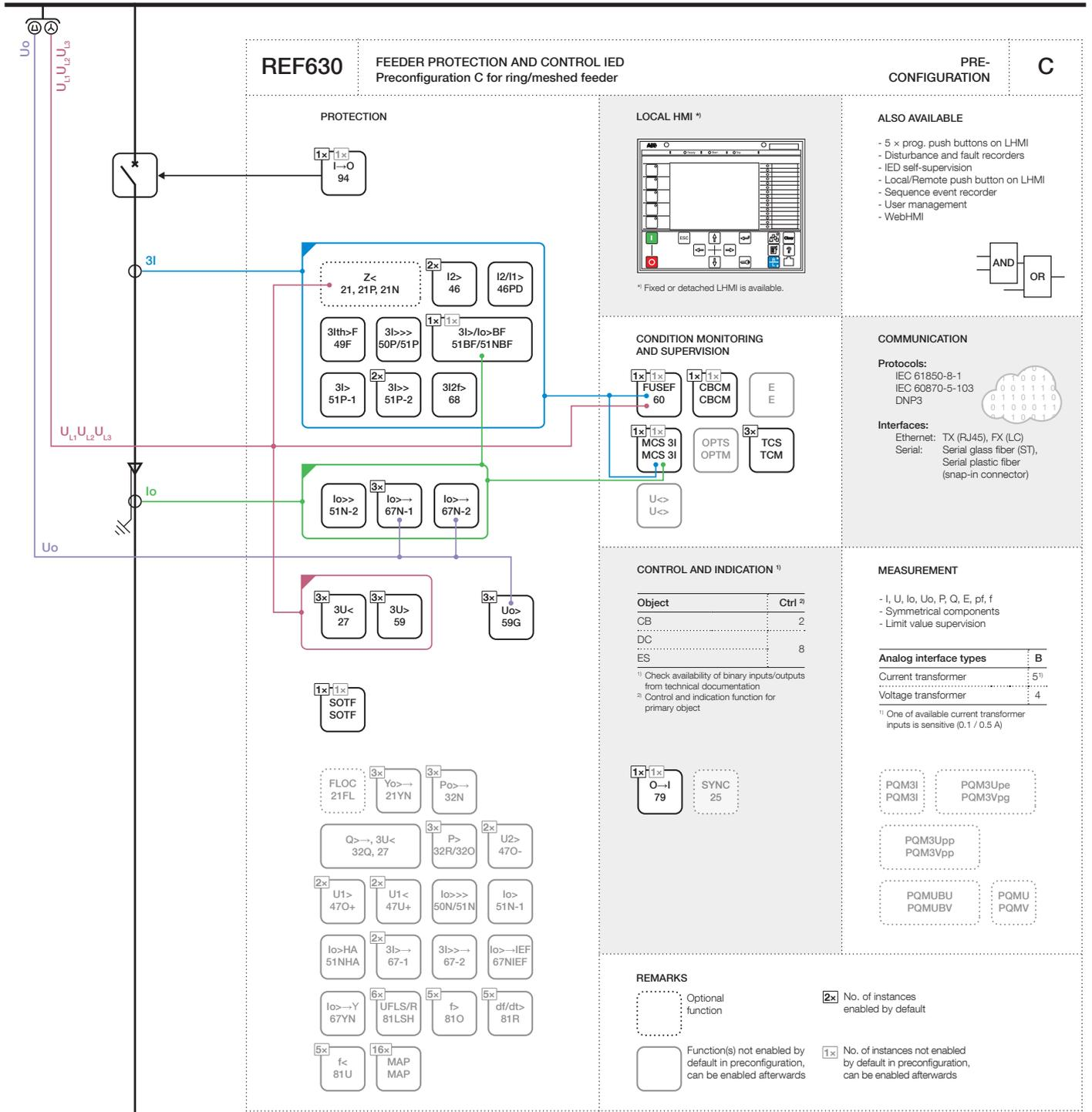
Figure 7. Functionality overview for preconfiguration C
