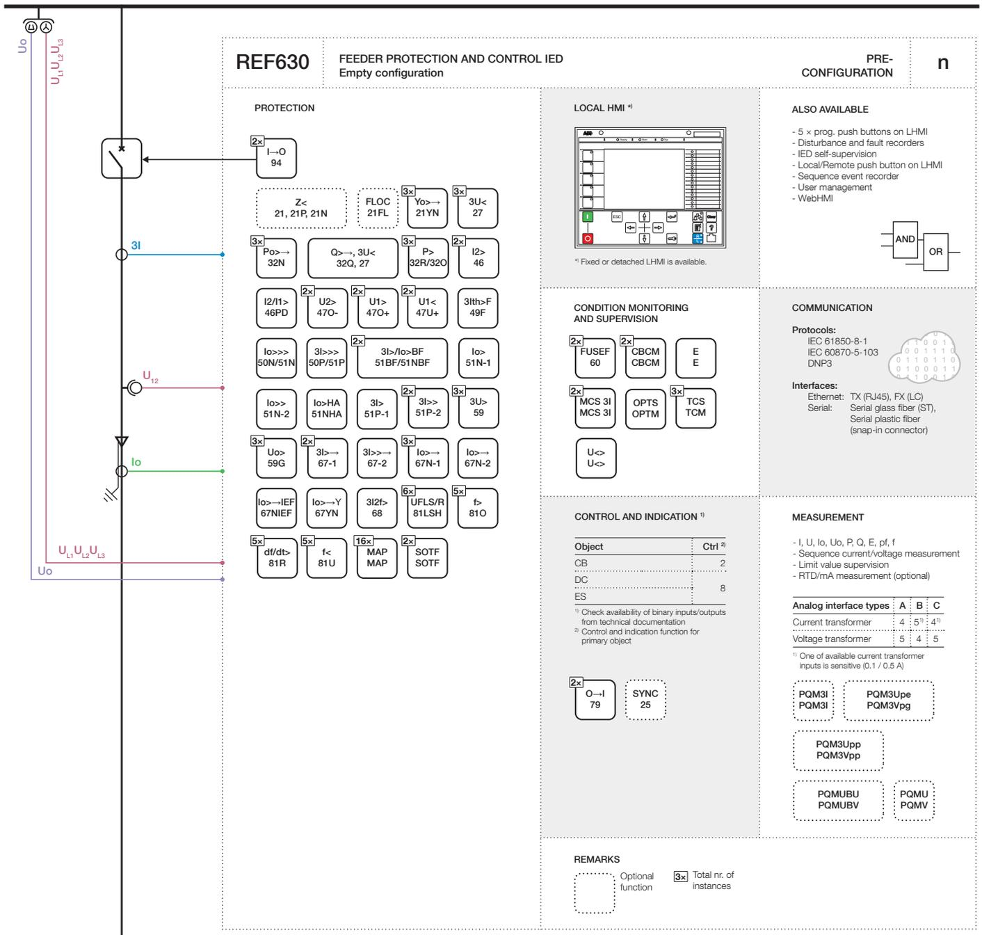
Figure 9. Functionality overview for preconfiguration n
