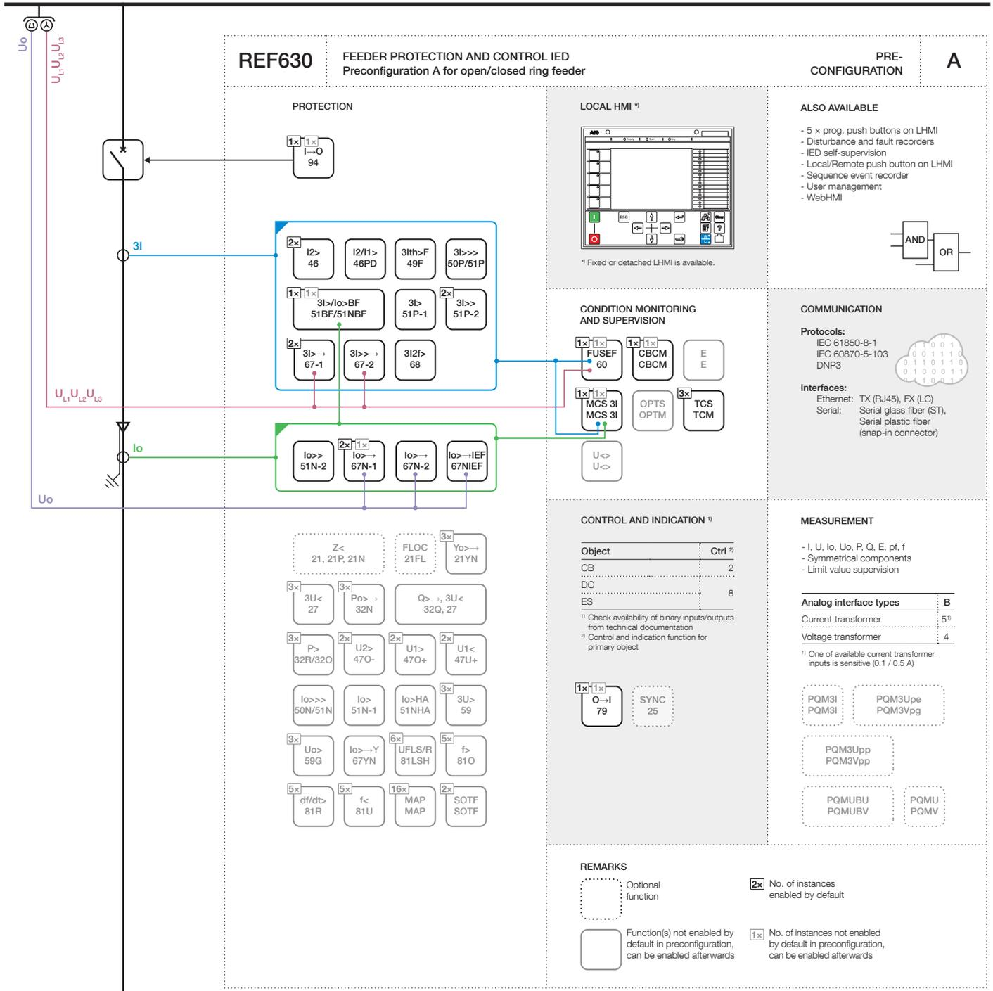
Figure 5. Functionality overview for preconfiguration A
