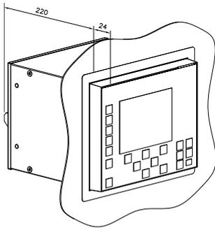
Figure 11. Flush mounting
