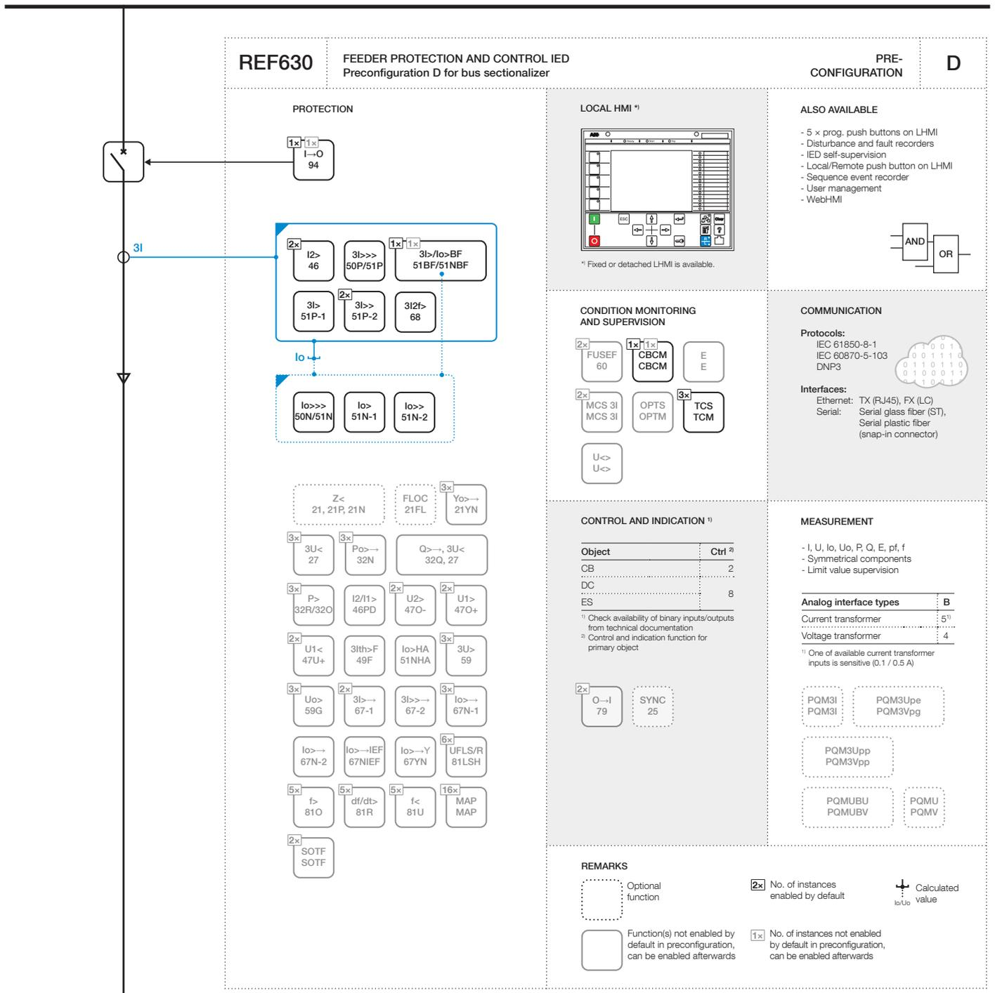
Figure 8. Functionality overview for preconfiguration D
