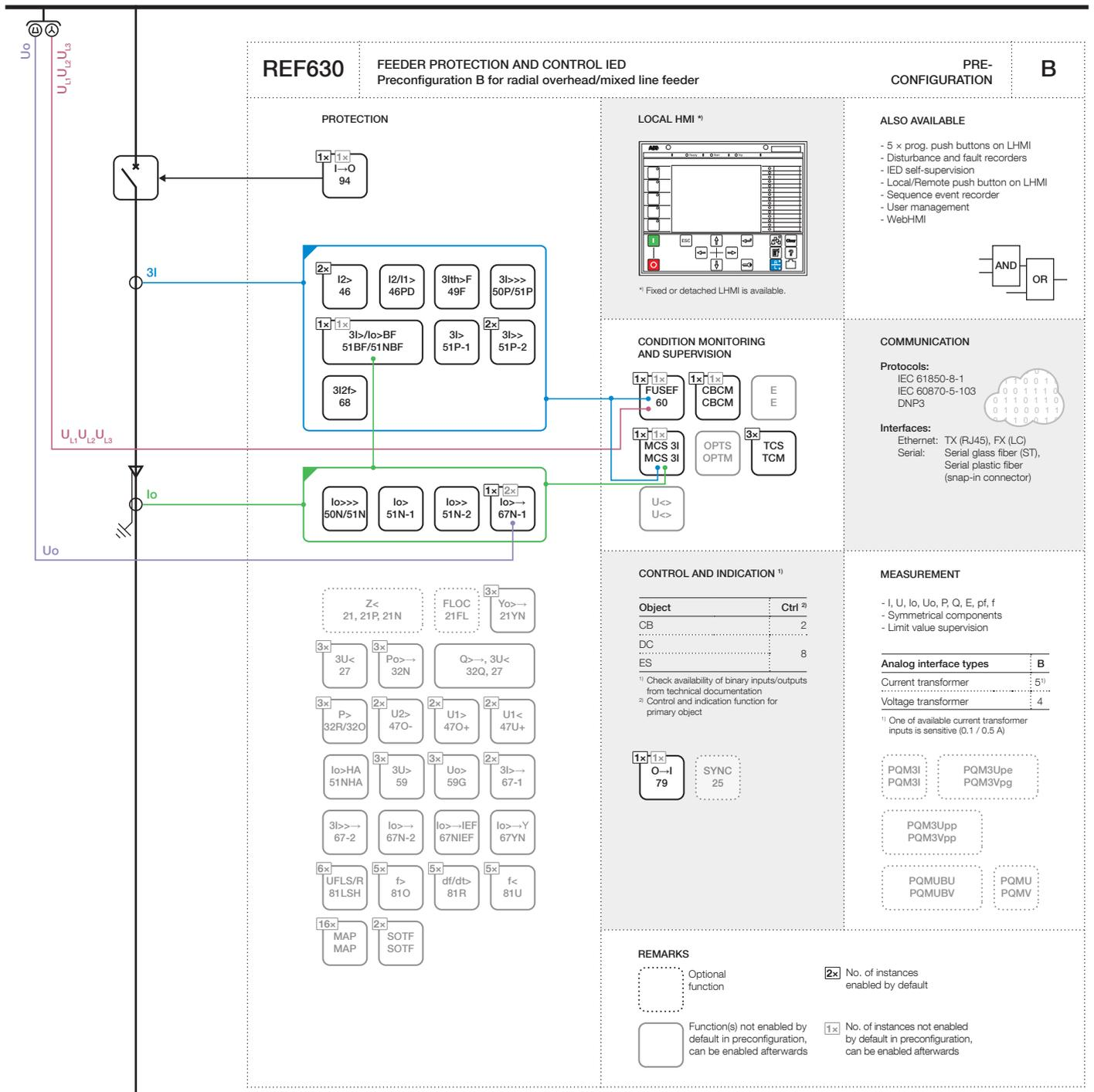
Figure 6. Functionality overview for preconfiguration B
