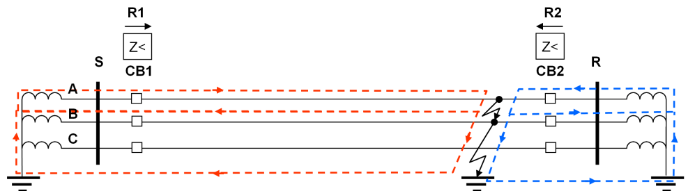
Figure 382: Two-phase-to-earth fault in low-impedance earthed system
