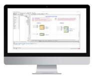
Application configuration allows you to easily create, change or view an IED configuration. The colors of the function blocks relate to the function status in the configuration: unconnected (gray), partially connected (yellow) or fully connected (green).
