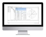
The parameter setting tool allows you to change or view all the parameters that an IED has, for all the setting groups. When reading the parameters from the IED, you can easily compare the values in the PC with the ones in the IED. The graphical representation of protection characteristics supports you in visualizing, for example, distance protection parameter setting.
