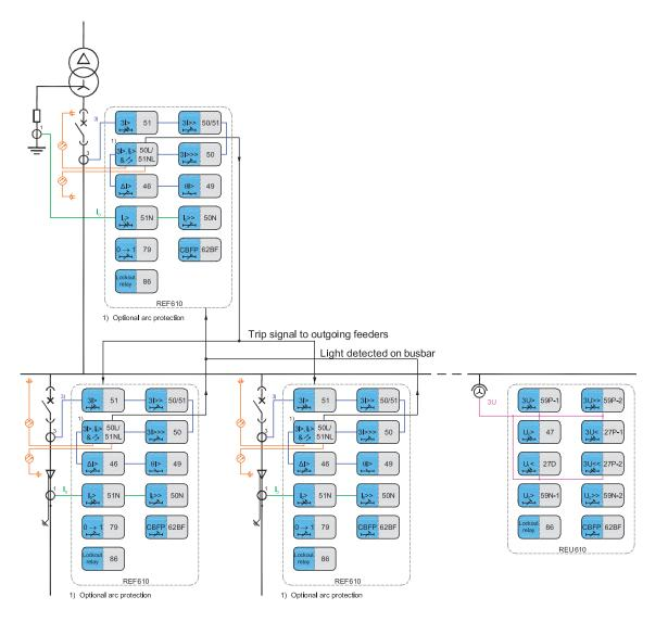
Figure 2. Substation O/C and E/F protection based on 610 series protection relays. Equipped with an optional hardware module REF610 also provides fast and selective arc fault protection.
