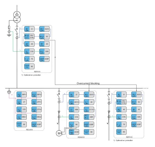
Figure 3. Substation feeder O/C and E/F protection, and substation busbar protection based on 610 series protection relays. The operate time of the busbar protection has been speeded up using the principle of upstream interlocking.
