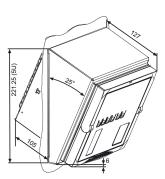
Figure 6. Semi-flush mounting in a 25° angle
