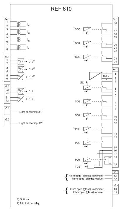
Figure 9. Terminal diagram of REF610
