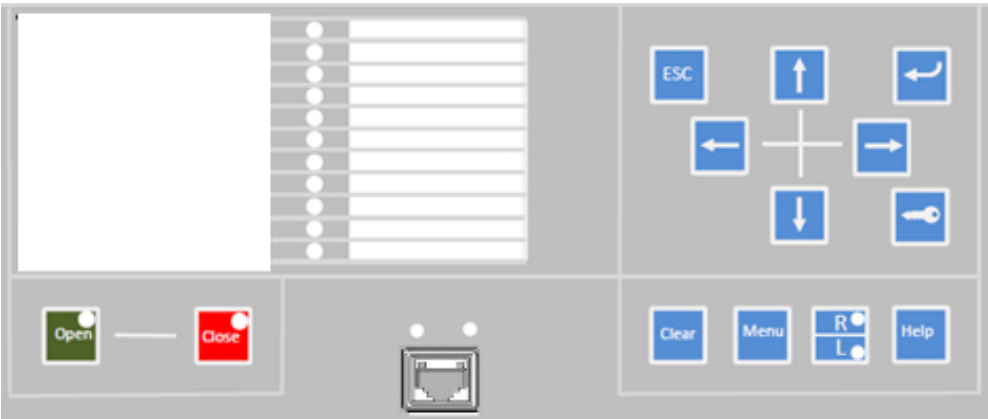
Figure 7a: LHMI (ANSI) keypad with object control, navigation, display, LEDs and command pushbuttons and RJ-45 communication port
