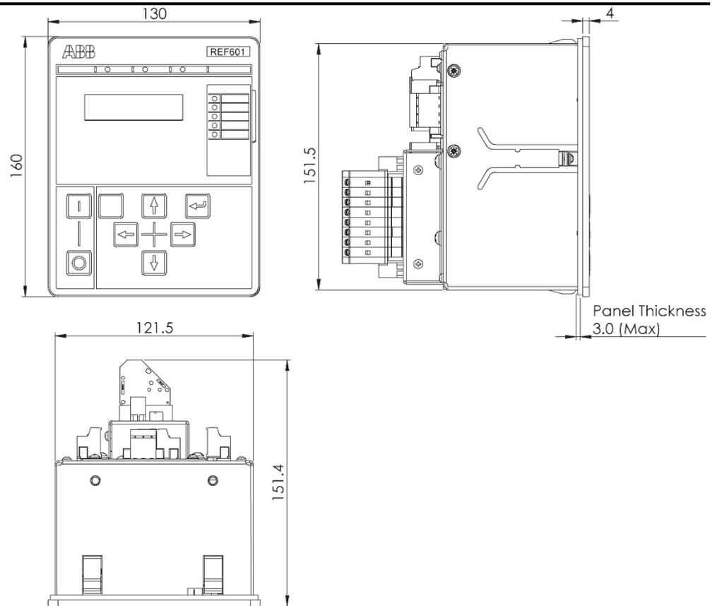
Figure 33: Overall mounting dimension of REF601 / REJ601
