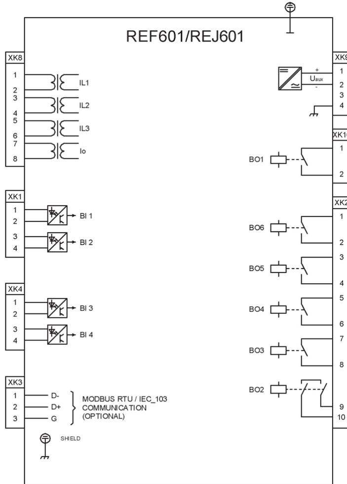
Figure 35: Connection diagram of relay REF601 / REJ601
