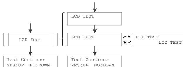
Figure 27: Hardware test menu of relay REF601 / REJ601 with its submenu
