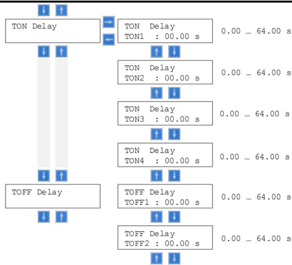
Figure 24: Configuration menu of relay REF601 / REJ601 with its submenu, continue
