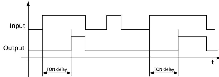
Figure 11 : Behavior of On delay timer TON
