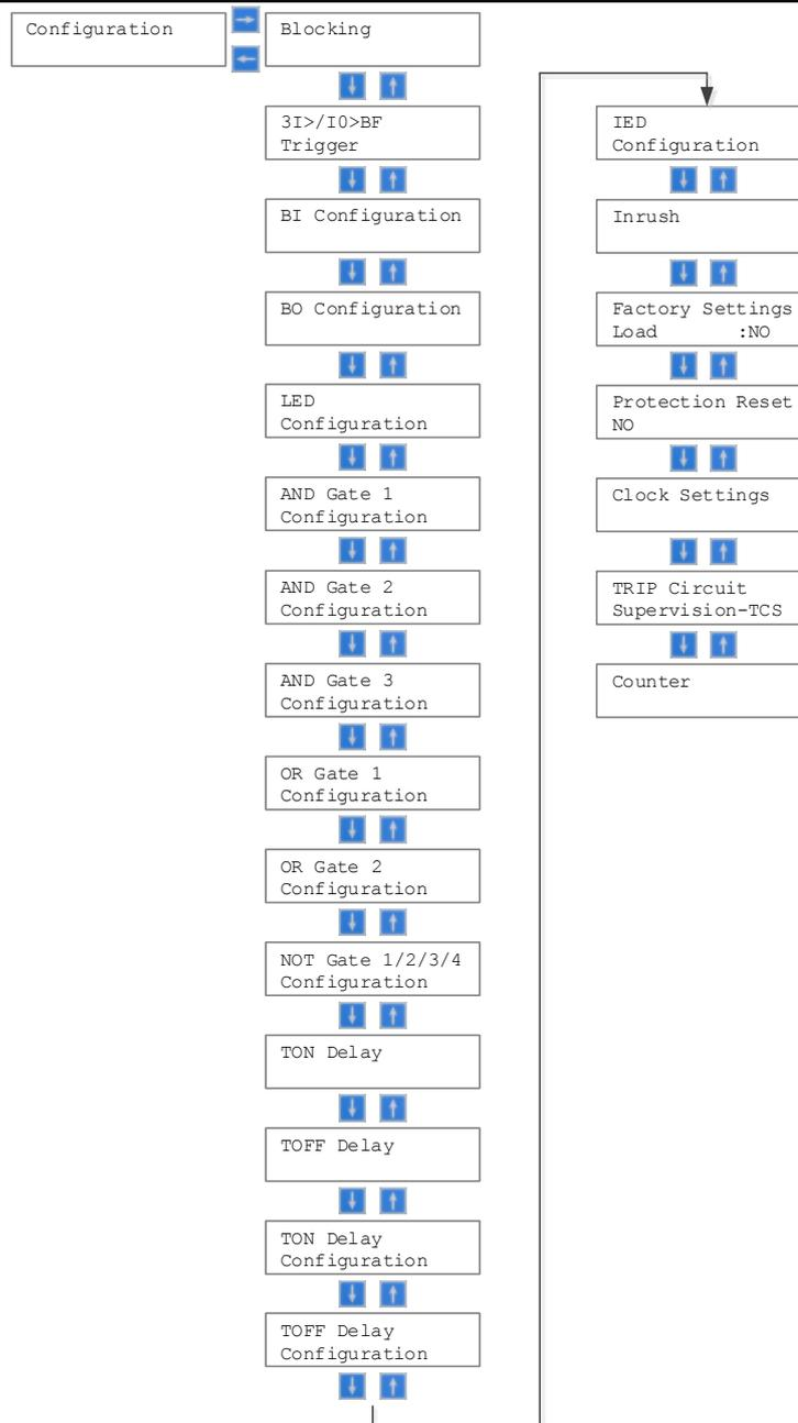
Figure 24: Configuration menu of relay REF601 / REJ601 with its submenu
