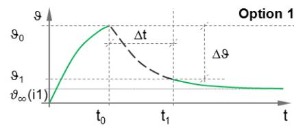
Option 1: When the power is restored after  $\Delta t$ , the new value of current after power on will be considered (which can be more or less compared to when power was interrupted) to calculate new value of thermal image for  $\Delta t$ .
