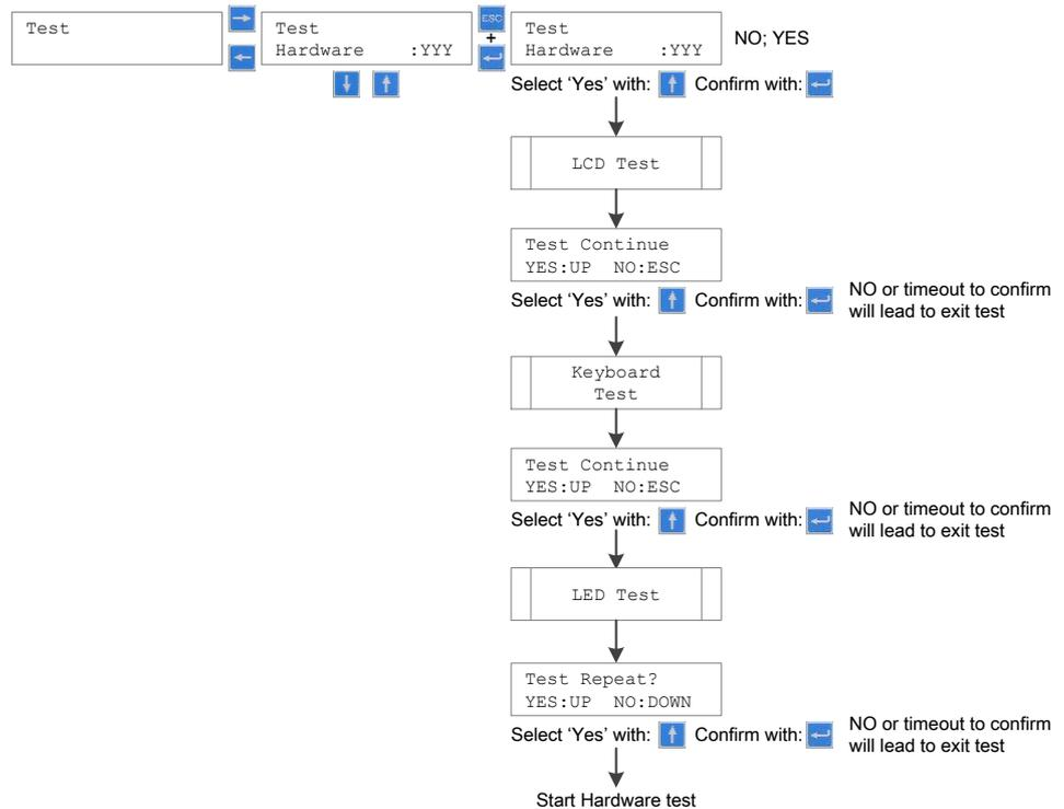
Figure 26: Hardware test menu of relay REF601 / REJ601 with its submenu
