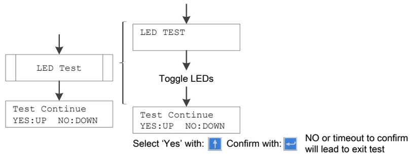
Figure 28: Hardware test menu of relay REF601 / REJ601 with its submenu (Continue)
