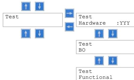
Figure 25: Test menu of relay REF601 / REJ601 with its submenu
