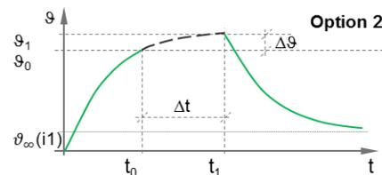
Option 2. When the power is restored after  $\Delta t$ , the new value of thermal image is calculated for  $\Delta t$  considering that the current has remained constant at the value when the power was interrupted.
