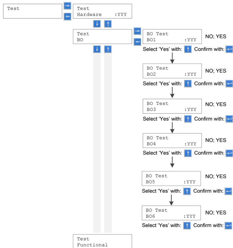
Figure 29: Binary output test menu of relay REF601 / REJ601 with its submenu
