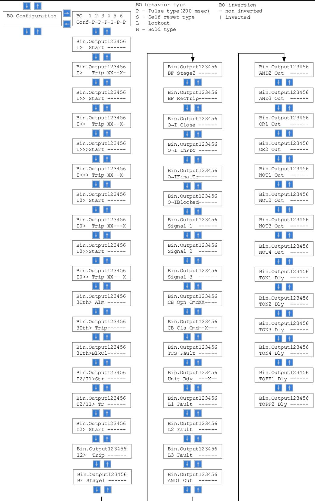
Figure 24: Configuration menu of relay REF601 / REJ601 with its submenu, continue
