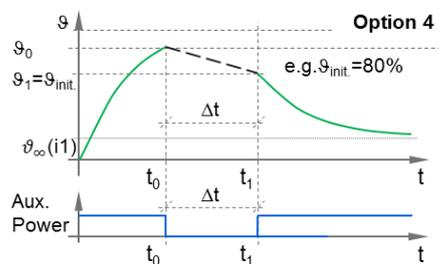
Option 4: Power interruption of the IED resets the thermal image to the set value defined by setting  $\vartheta_0$ .
