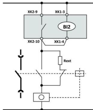
Figure 13: Application diagram of TCS function
