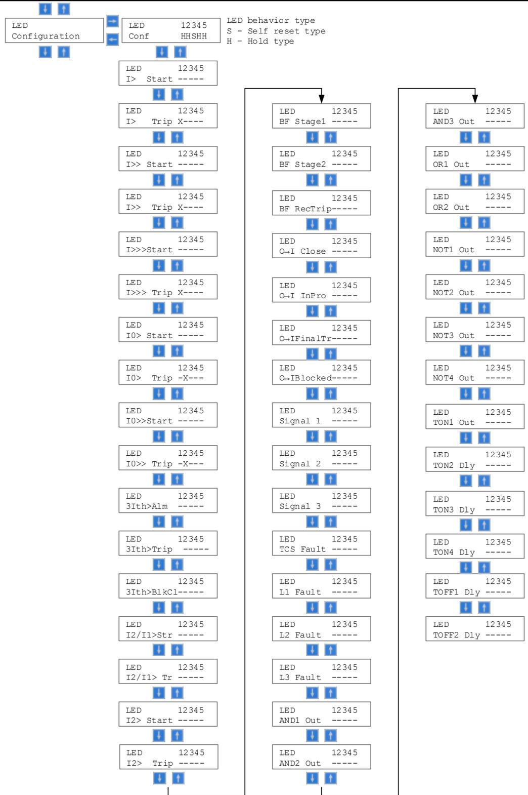
Figure 24: Configuration menu of relay REF601 / REJ601 with its submenu, continue
