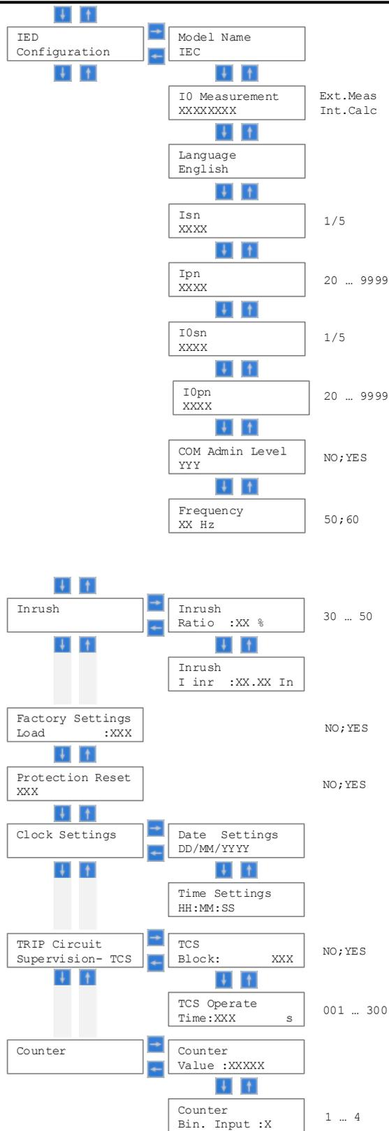
Figure 24: Configuration menu of relay REF601 / REJ601 with its submenu
