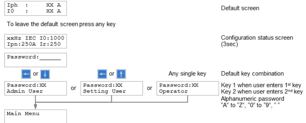
Figure 15: Login process of relay REF601 / REJ601
