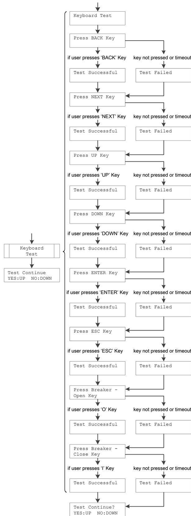
Figure 28: Hardware test menu of relay REF601 / REJ601 with its submenu (Continue)
