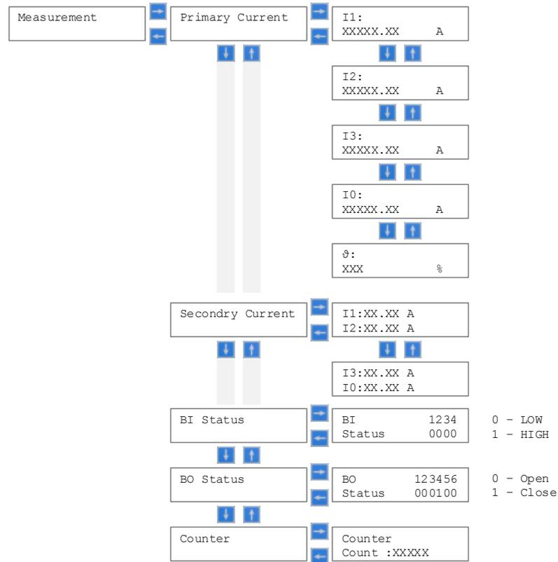
Figure 20: Measurement menu of relay REF601 / REJ601
