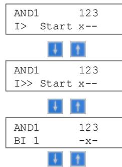
*Figure 8: Example of multiple input configured to AND Input 1*
