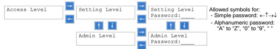
Figure 16: Password configuration in relay
