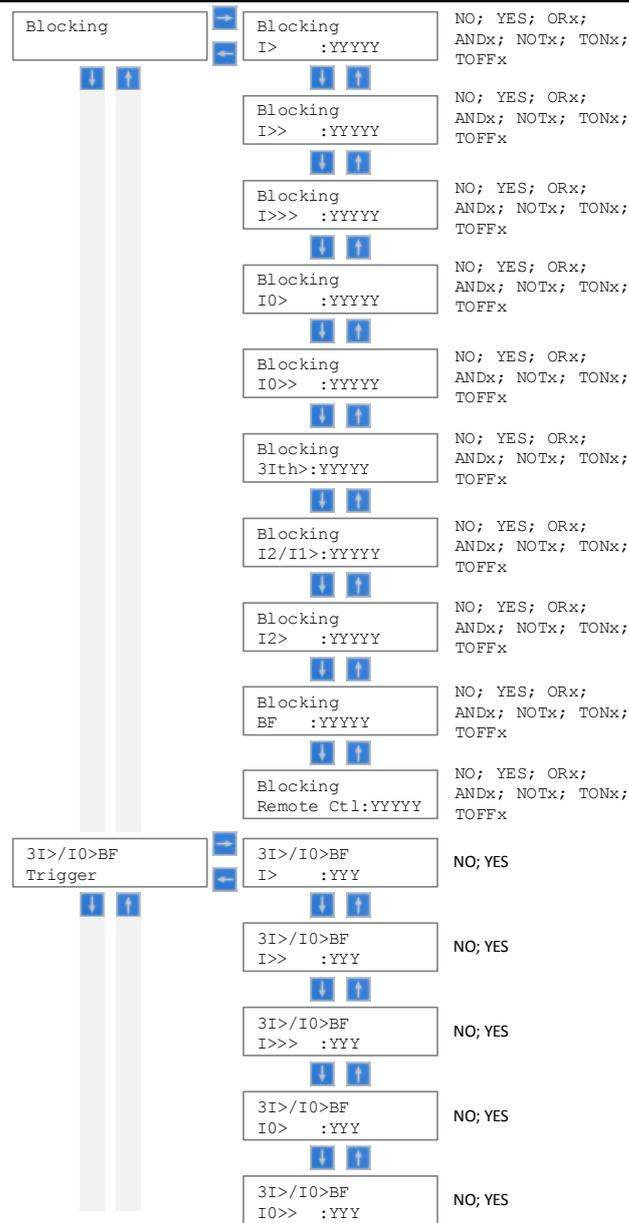
Figure 24: Configuration menu of relay REF601 / REJ601 with its submenu, continue
