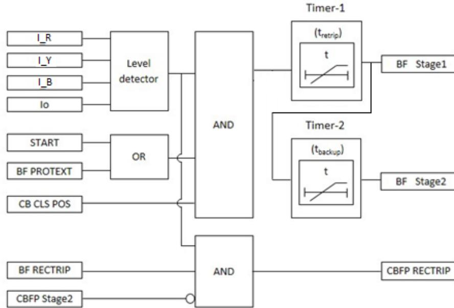
Figure 3: Circuit breaker failure protection functional module diagram
