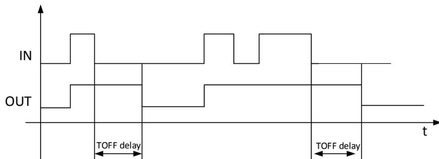
Figure 12: Behavior of Off delay timer TOFF
