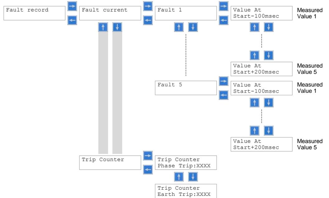
Figure 21: Fault record data menu of relay REF601 / REJ601
