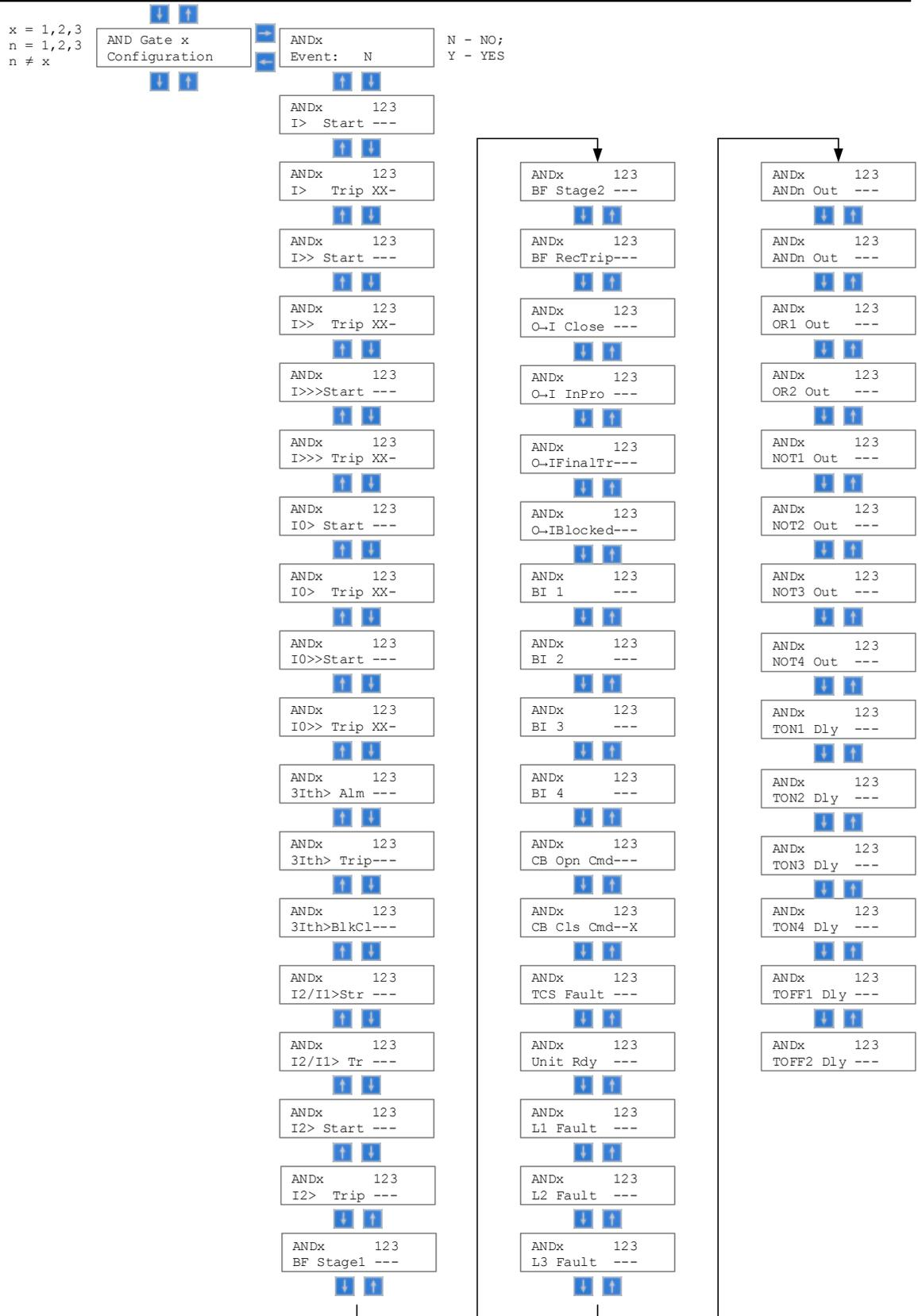
Figure 24: Configuration menu of relay REF601 / REJ601 with its submenu, continue
