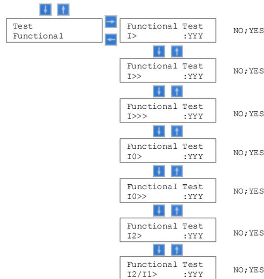
Figure 30: Functional test menu of relay REF601 / REJ601
