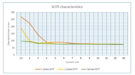
Figure 2: Switch-on to fault characteristics of relay REJ603
