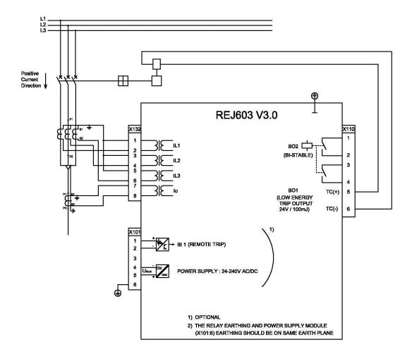
Figure 6. Terminal diagram of REJ603 V3.0 with external earth connection through CBCT
