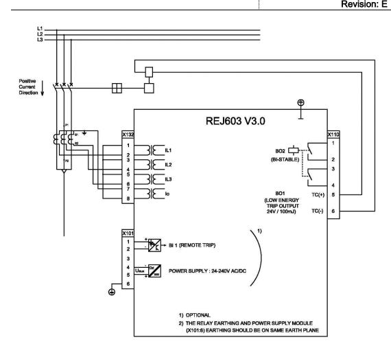
Figure 7. Terminal diagram of REJ603 V3.0 with external earth connection through residual connection
