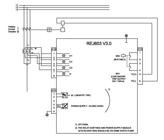
Figure 8. Terminal diagram of REJ603 V3.0 with internal earth connection
