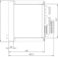
Figure 3. Dimension of REJ603 – Flush mounting
