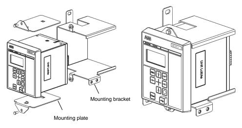
Figure 4. Typical mounting of relay in RMU (Mounting plate and bracket not supplied along with relay)
