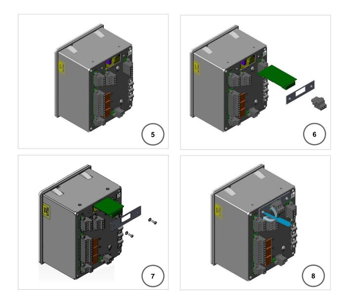
How to install communication card in relay:
