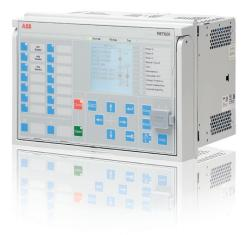
form-based blocking algorithm ensures stability at transformer energization and a fifth harmonic restraint function ensures good protection stability at moderate overexcitation of power transformers. Sensitive restricted earth-fault protection (REF) completes the overall differential protection to detect even single phase-to-ground faults close to the grounded neutral of the transformer.
