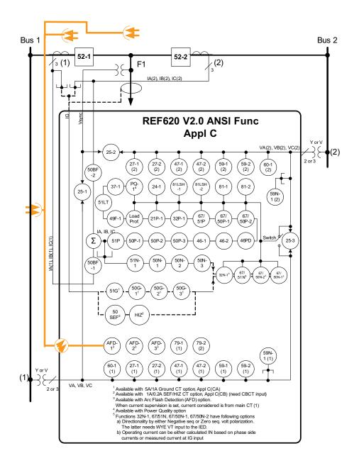
All configurations include standard metering, monitoring and control features and sequence of event, fault and digital waveform recording. Advanced Ethernet communications included standard with parallel support of DNP3 Level 2+\*, Modbus and IEC61850 and SNTP over TCP/IP. Additional RS-232 and
