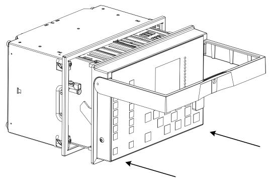
Figure 3: Installing a plug-in unit into the case
