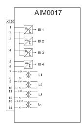
Figure 9: Example of AIM0017 card variant (4 I with 0.2/1 A lo channel)
