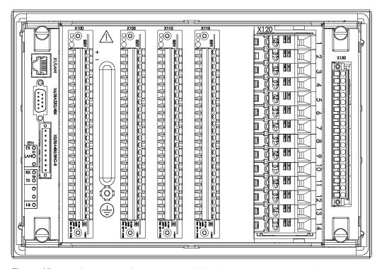
Figure 15: Rear view of an 620 series IED with communication module
