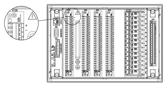
Figure 11: Connecting auxiliary voltage
