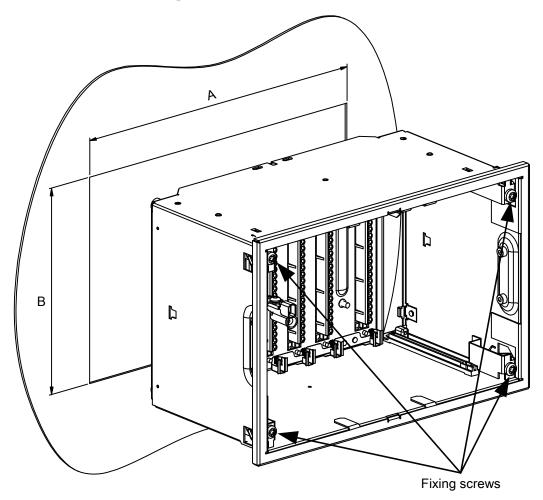
Figure 5: Flush mounting a case into a panel cut-out
