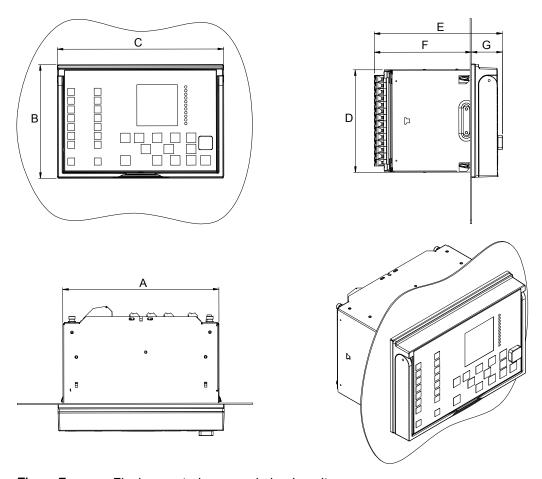
Figure 7: Flush mounted case and plug-in unit
