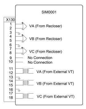
Figure 10: Example of voltage input connections to SIM0001
