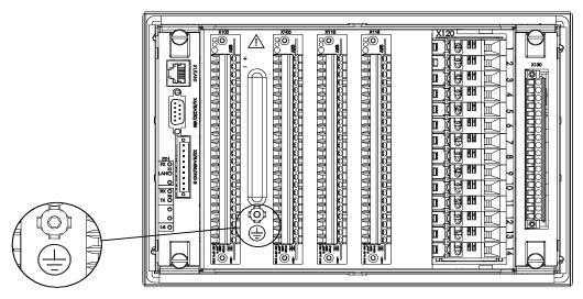
Figure 8: The protective earth screw is located between connectors X100 and X105
