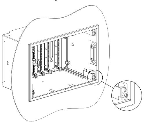
Figure 13: Loosening the fixing screws
