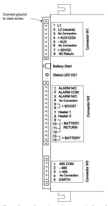
Figure 12: Connections to Uninterruptable Power Supply (UPS)
