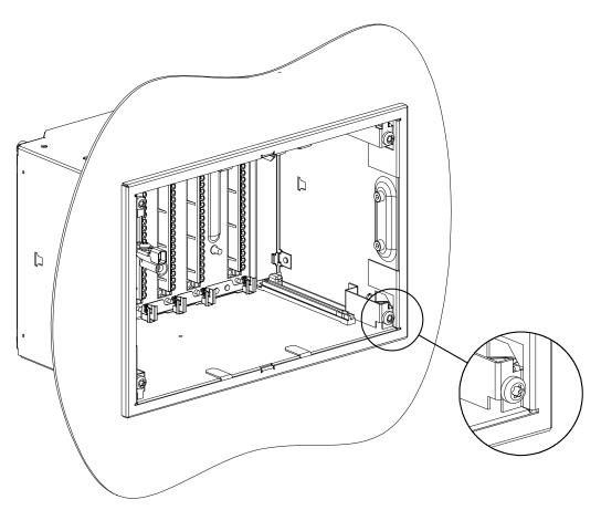
Flush mounted case, tightening the M5 fixing screws
