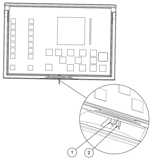
Figure 4: Sealing screw
