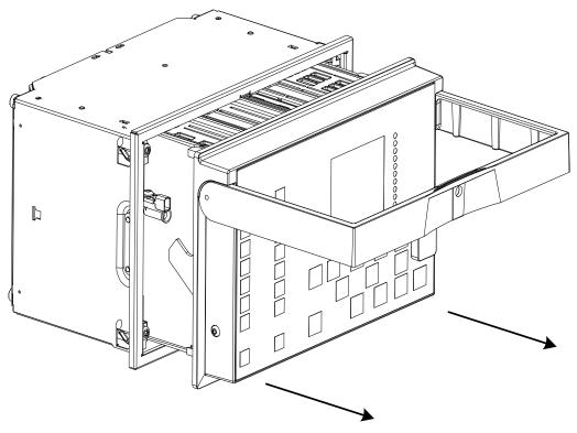
Figure 2: Detaching a plug-in unit from the case
