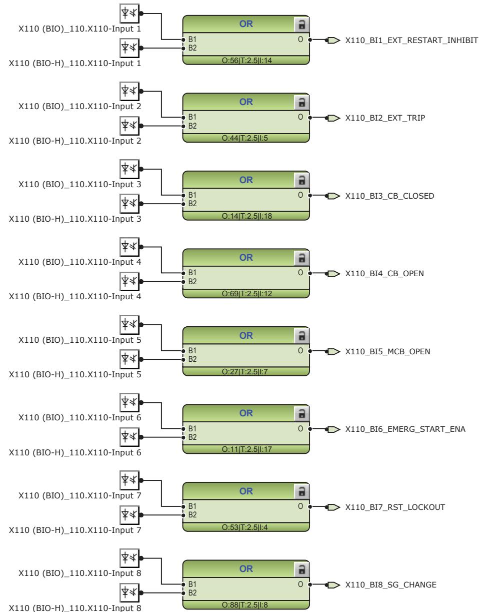
Figure 92: Default binary inputs - X110
