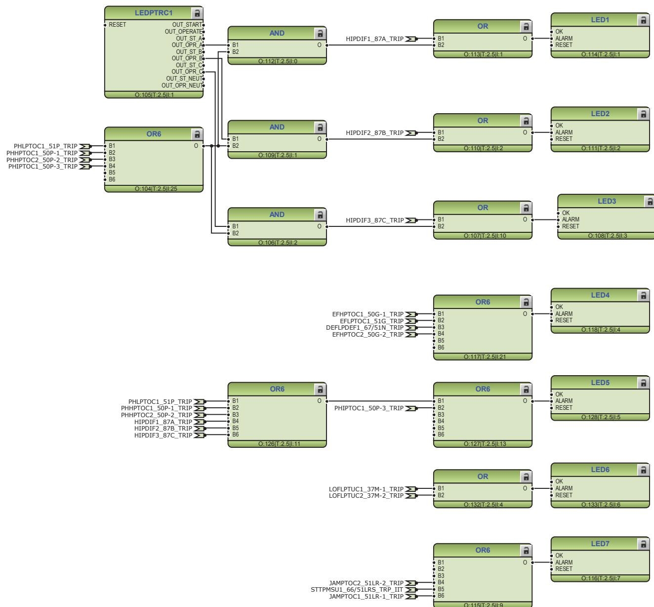
Figure 198: Default LED connections
