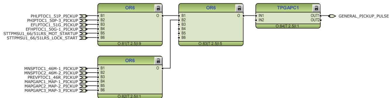
**Figure 27:** General pickup and trip signals
