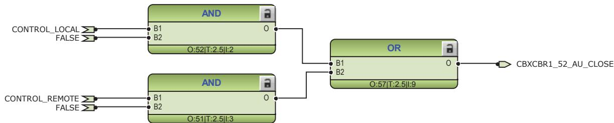
*Figure 131: External closing command for circuit breaker 1*
