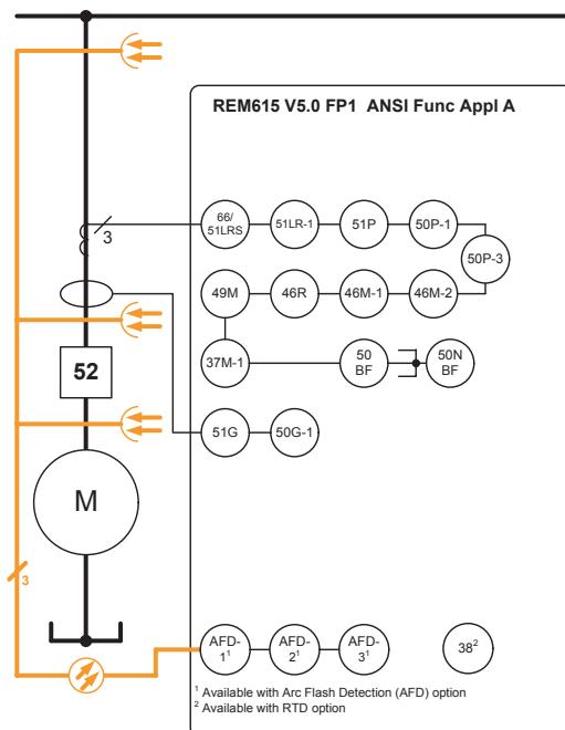
Figure 14: Functionality overview for standard configuration A
