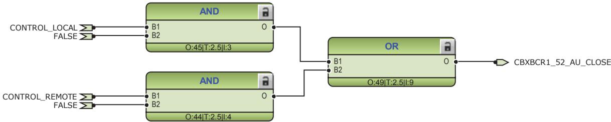
Figure 39: External closing command for circuit breaker 1
