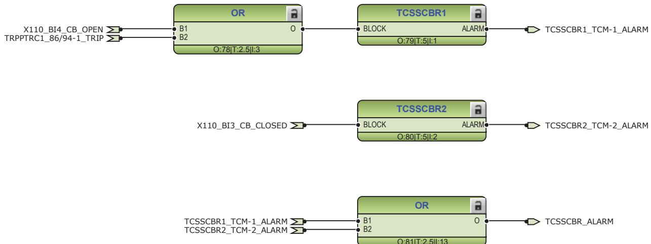
*Figure 76:* Trip circuit supervision function
