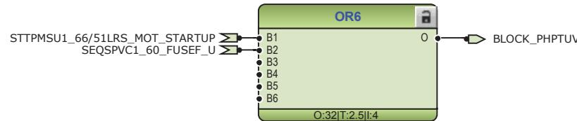
Figure 149: Blocking logic for phase undervoltage protection
