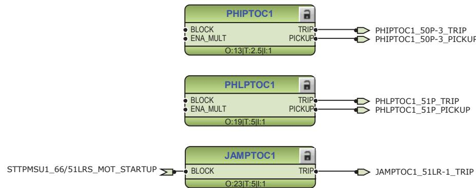
*Figure 15: Overcurrent protection functions*
