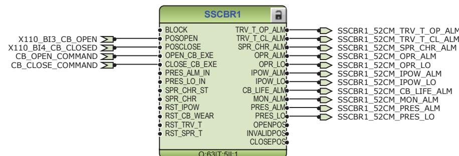
*Figure 123: Circuit-breaker condition monitoring function*
