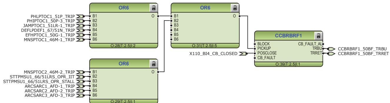
Figure 116: Circuit breaker failure protection function
