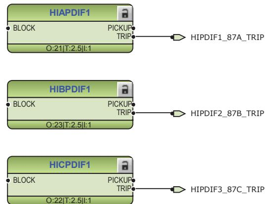
*Figure 156: Motor core-balanced current differential protection*
