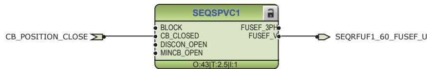
*Figure 181: Fuse failure supervision*
