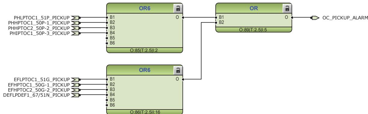
*Figure 159: Current pickup alarm*
