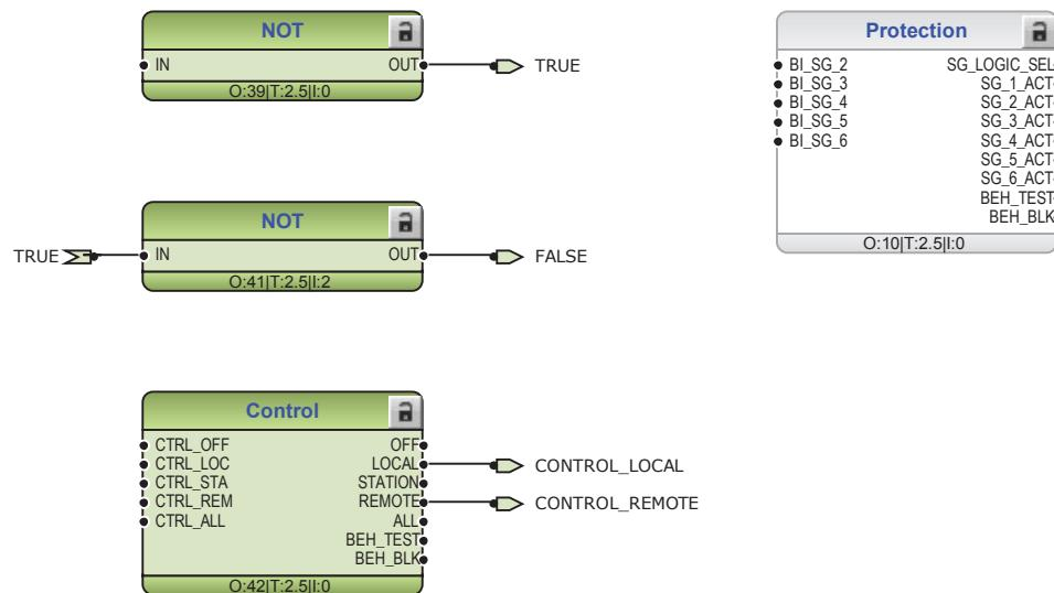
Figure 52: Functions for general logic states TRUE and FALSE, protection setting group selection and local and remote control
