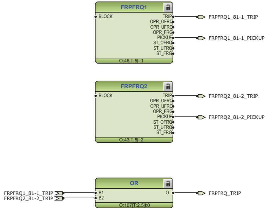
Figure 66: Frequency protection function
