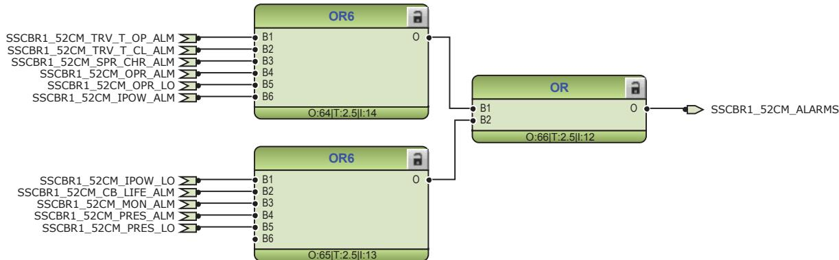
Figure 124: Logic for circuit breaker monitoring alarm
