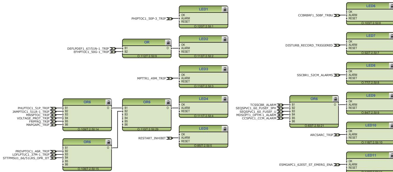
*Figure 96: Default LED connections*
