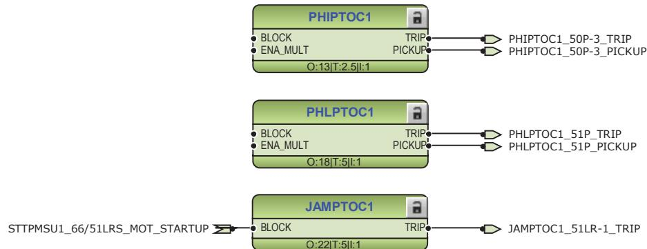
*Figure 55: Overcurrent protection functions*
