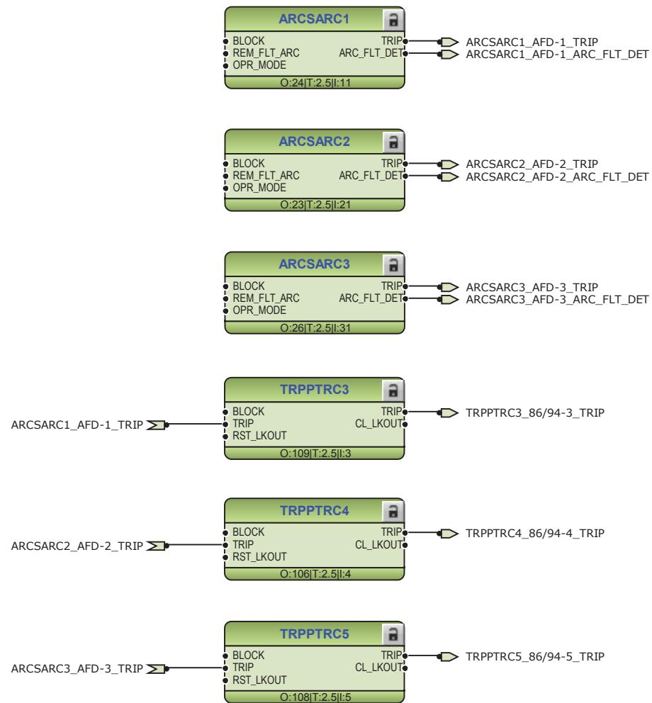
*Figure 117: Arc protection with dedicated high-speed output*
