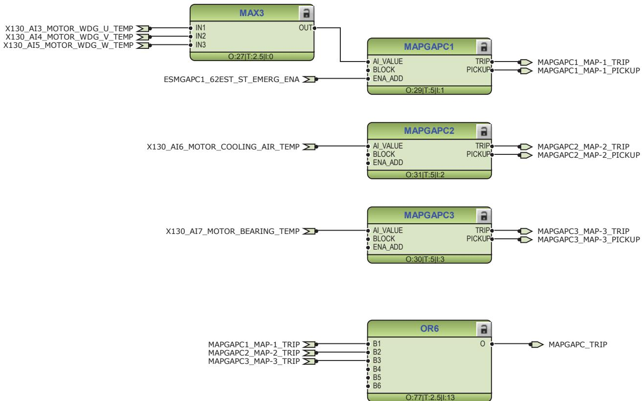
Figure 24: Multipurpose mA/RTD monitoring
