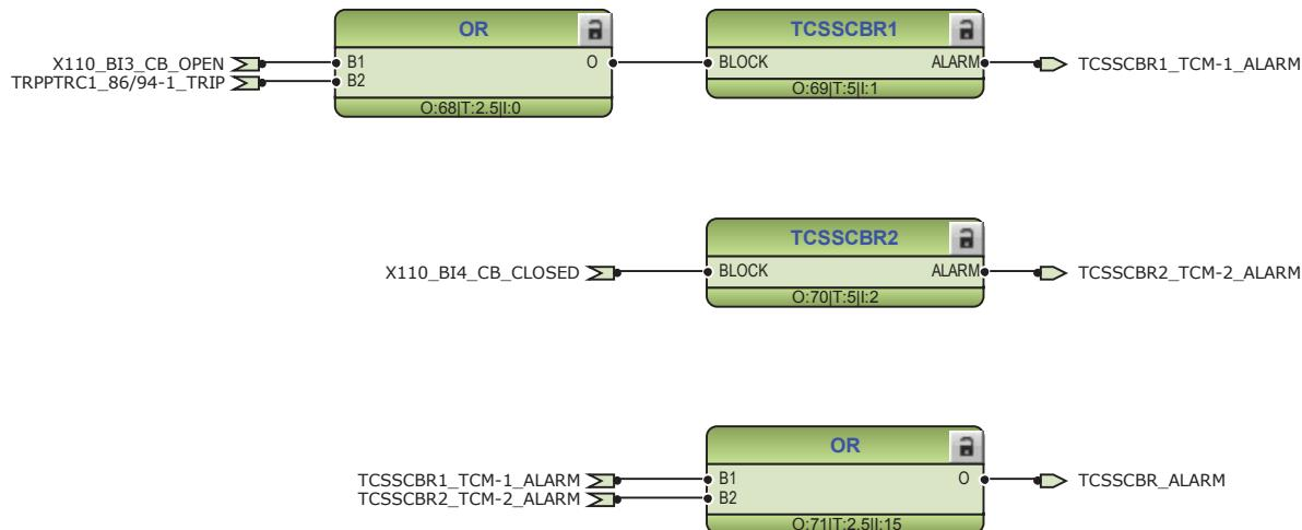
Figure 125: Trip circuit supervision function
