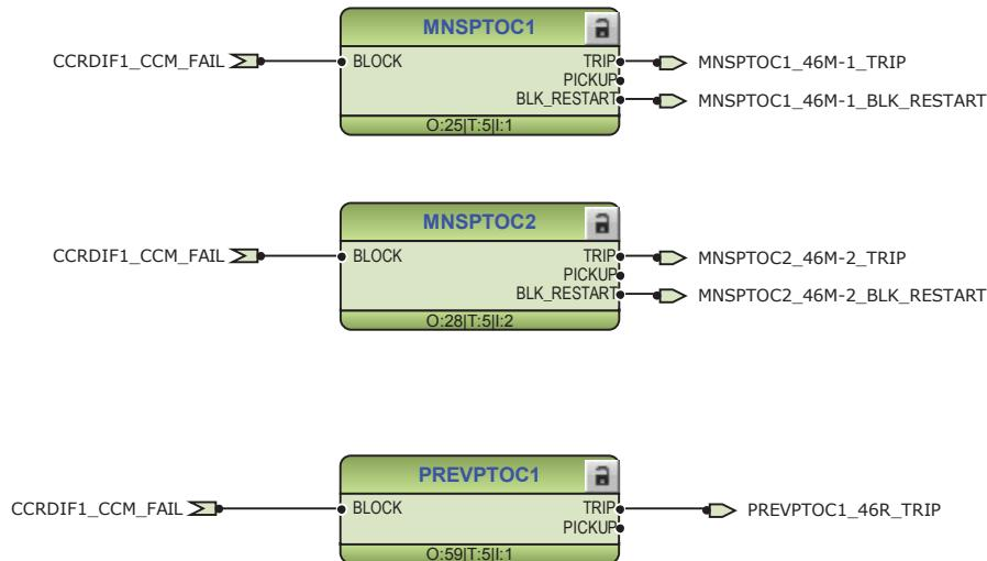
*Figure 167: Negative-sequence and phase reversal protection*
