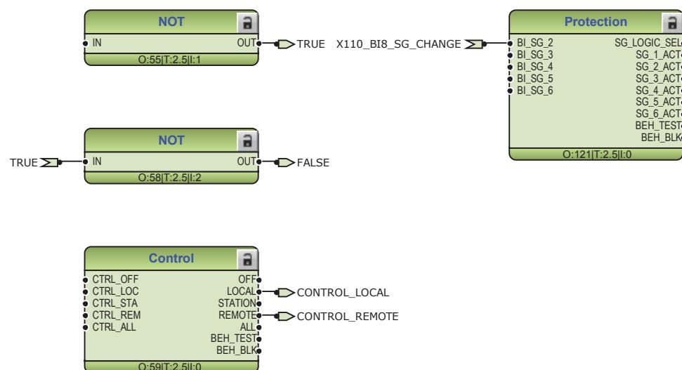
Figure 102: Functions for general logic states TRUE and FALSE, protection setting group selection and local and remote control
