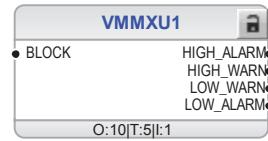
*Figure 189: Three-phase voltage measurement*
