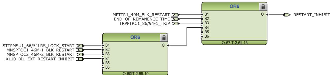
*Figure 81: Circuit breaker 1 close blocking logic*
