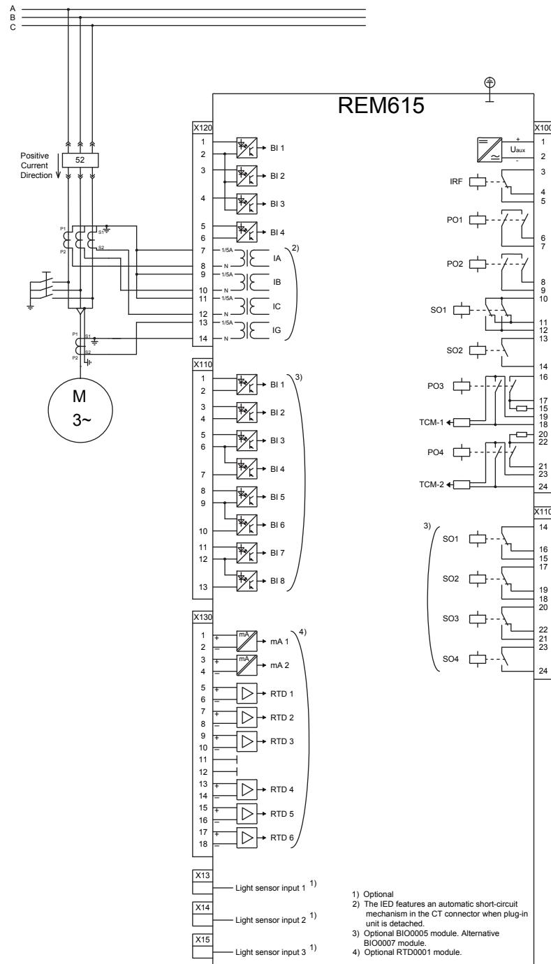
Figure 9: Connection diagram for the A configuration
