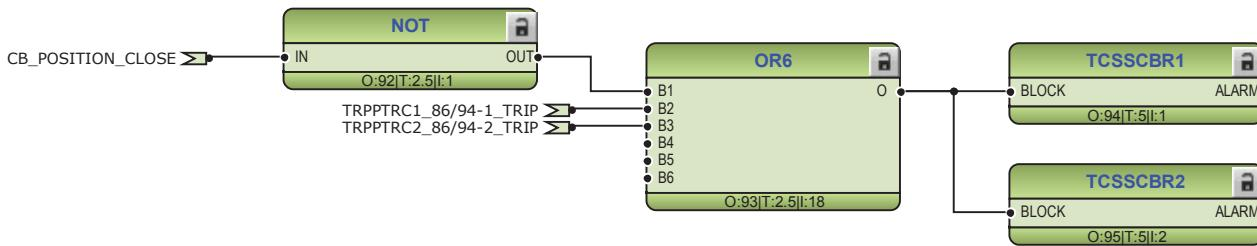
Figure 179: Trip circuit monitoring
