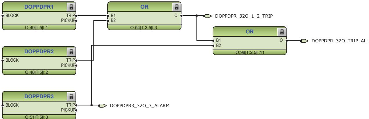
Figure 163: Directional overpower protections
