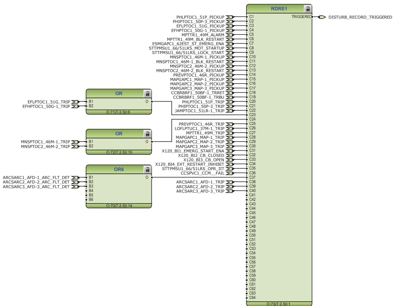
Figure 29: Disturbance recorder
