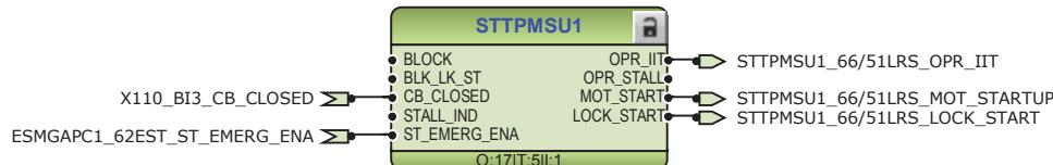
*Figure 61: Motor start-up supervision function*
