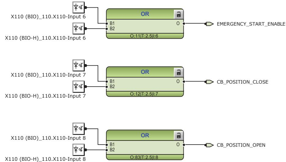
Figure 196: Default binary inputs - X110
