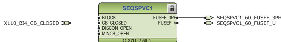
*Figure 122: Fuse failure supervision function*
