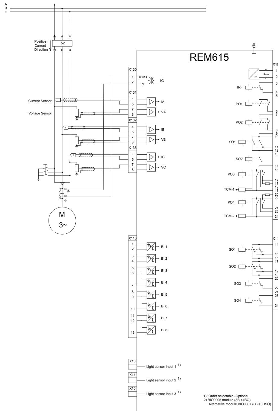
Figure 11: Connection diagram for the D configuration
