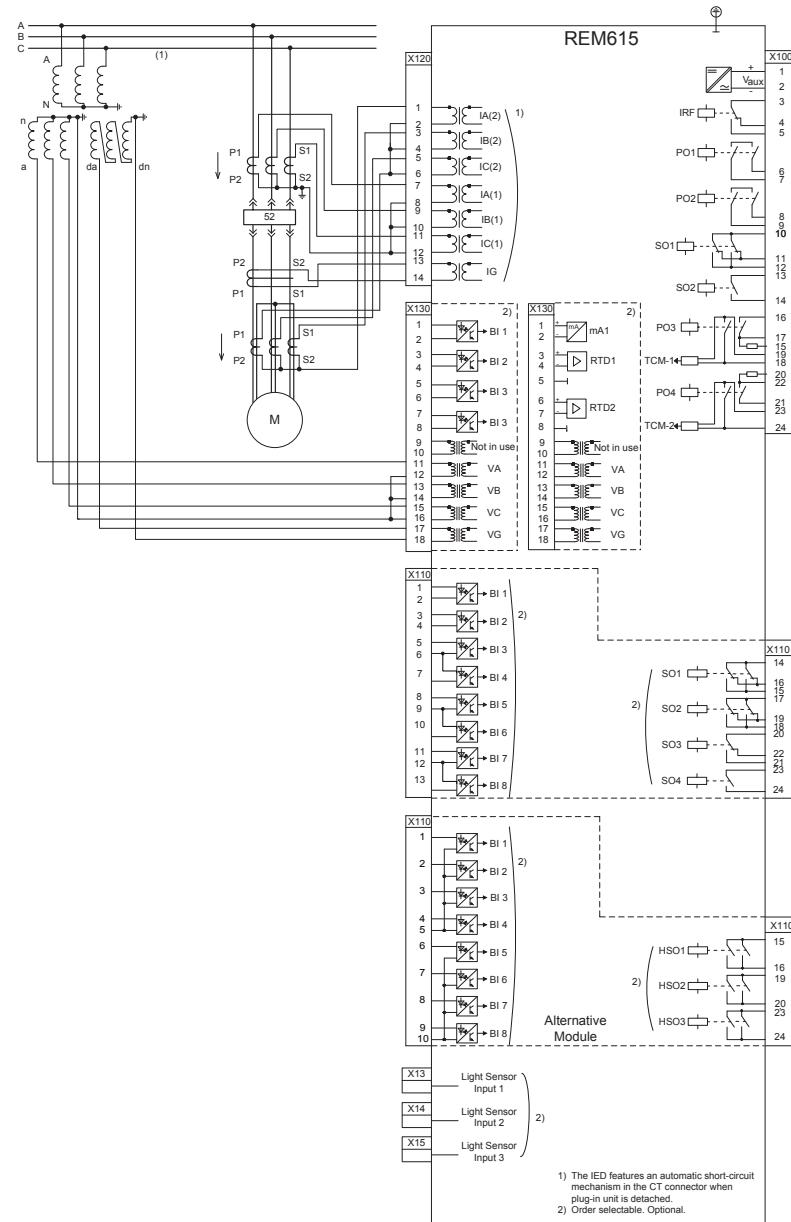
*Figure 13: Connection diagram for the E configuration with wye VT and core-balance based differential protection connection*
