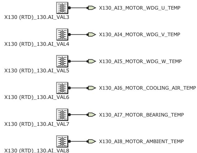
*Figure 95: Default mA/RTD inputs X130*
