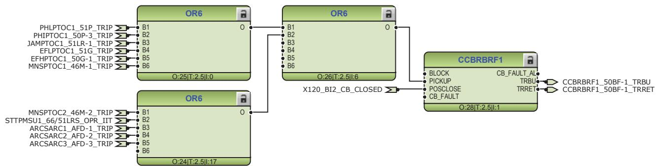
**Figure 25:** Circuit breaker failure protection function
