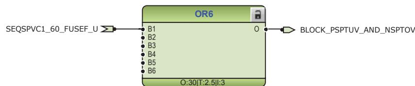
*Figure 148: Blocking logic for positive-sequence undervoltage and negative-sequence overvoltage protection*
