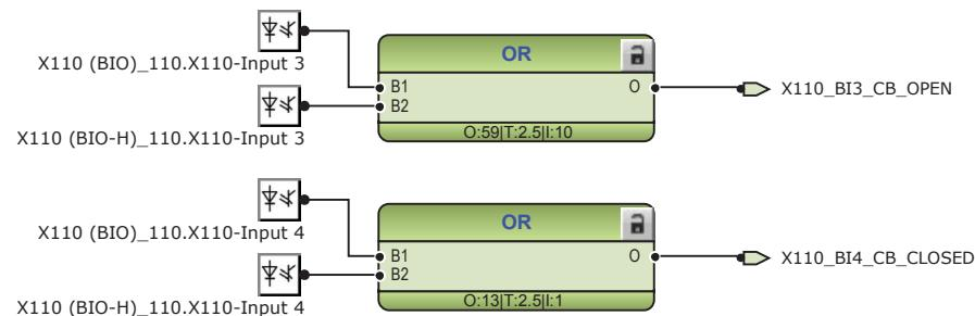
Figure 141: Default binary inputs - X110
