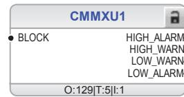
*Figure 84: Three-phase current measurement*
