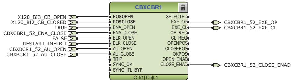
Figure 34: Circuit breaker 1 control logic
