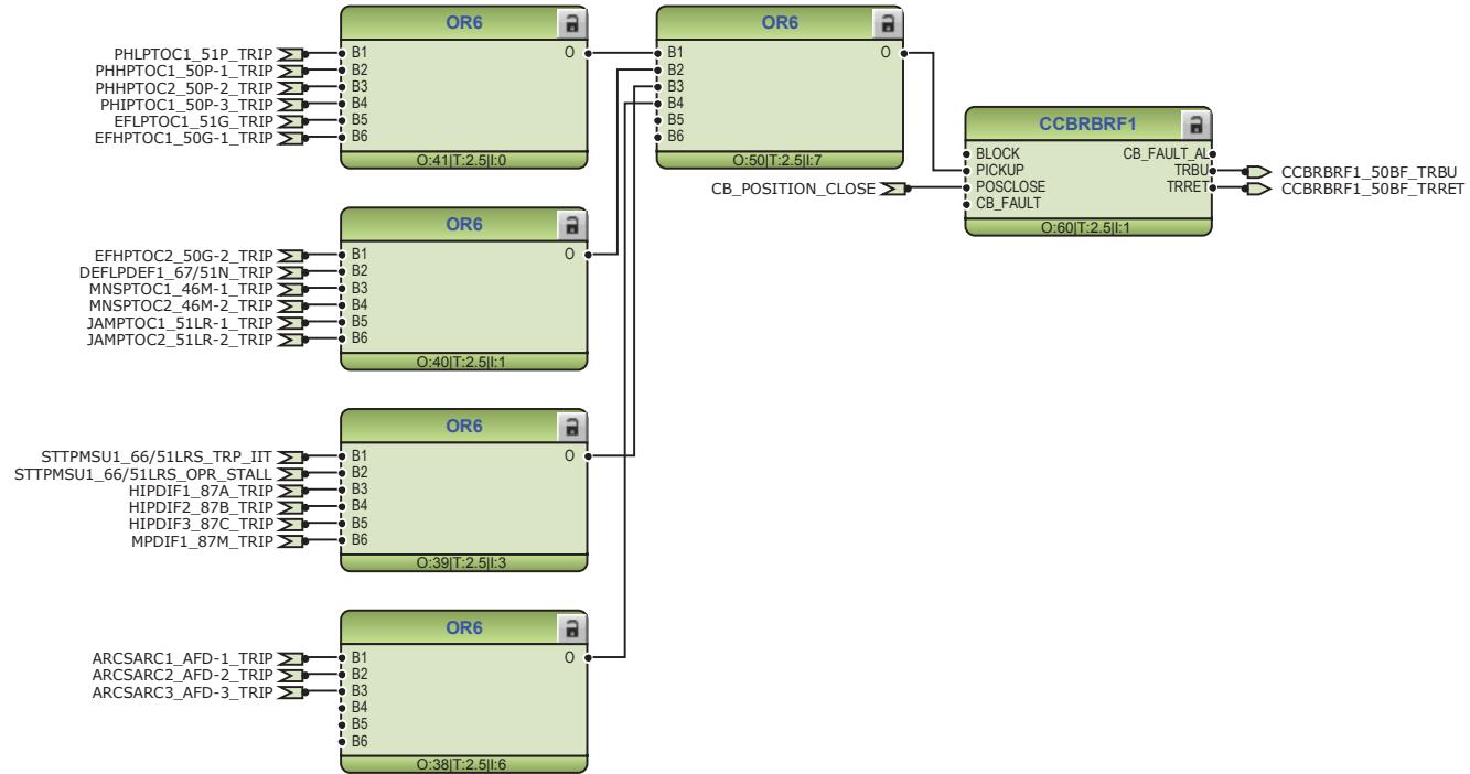
Figure 171: Circuit-breaker failure protection and associated binary output
