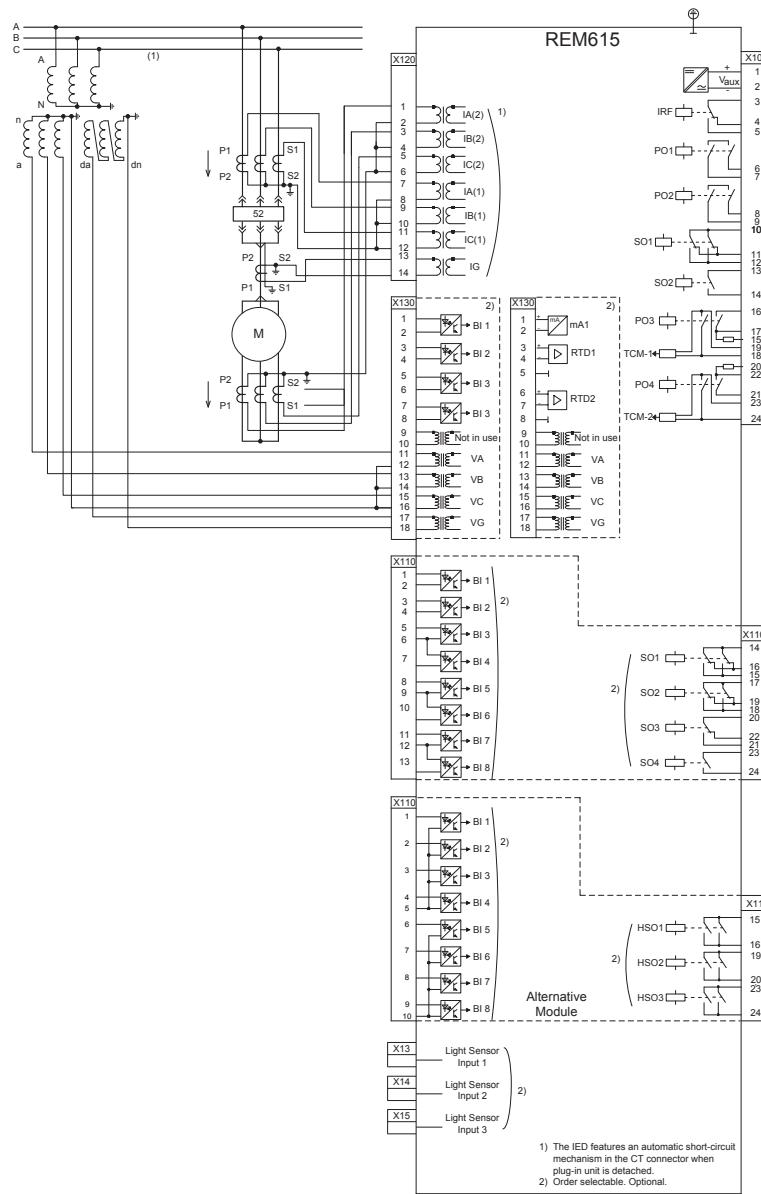
*Figure 12: Connection diagram for the E configuration with wye VT and true differential protection based connection*
