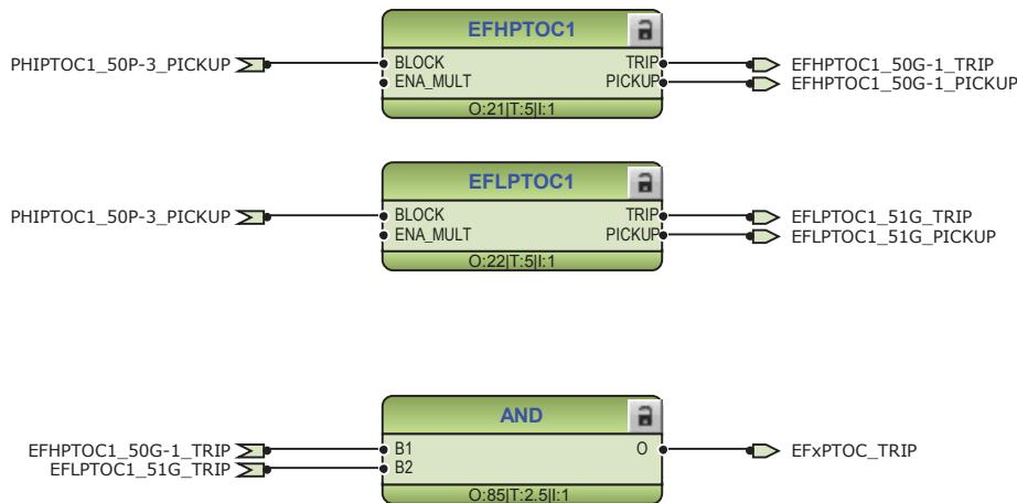
*Figure 18: Ground-fault protection functions*
