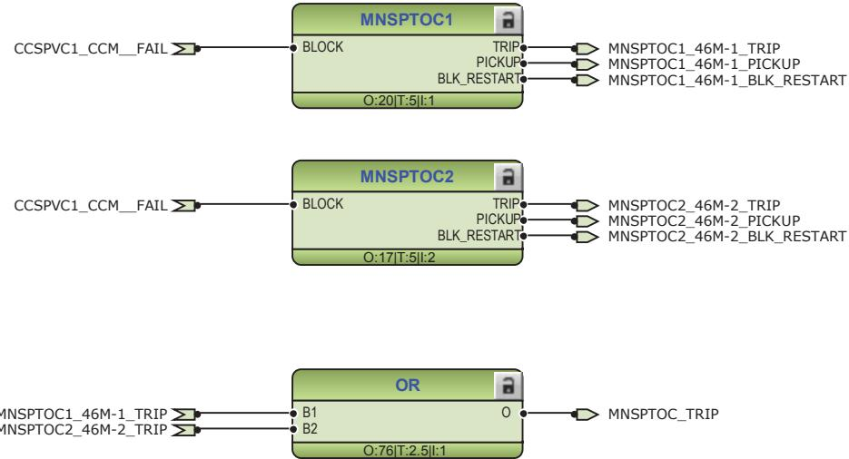
*Figure 16: Negative-sequence overcurrent protection function*
