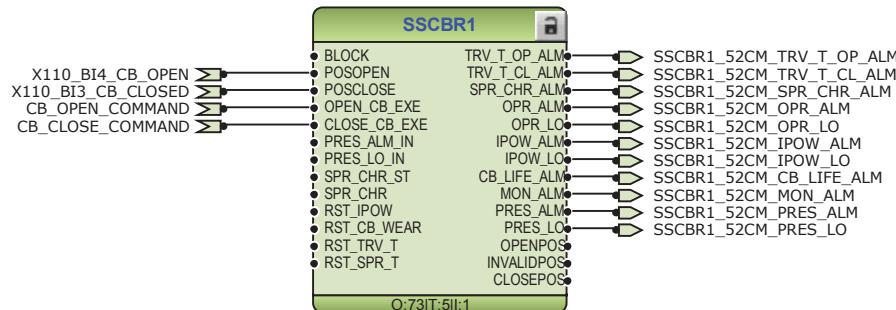
*Figure 74: Circuit-breaker condition monitoring function*
