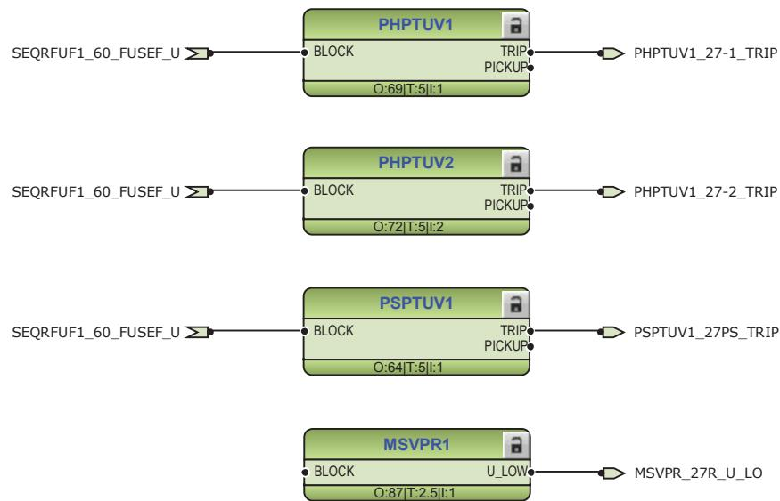
Figure 160: Undervoltage protections
