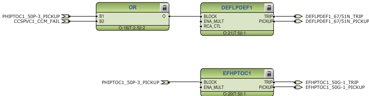
Figure 108: Ground-fault protection functions
