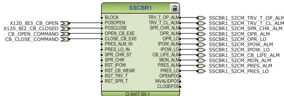
*Figure 31: Circuit-breaker condition monitoring function*
