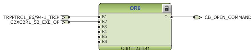
Figure 128: Signals for opening coil of circuit breaker 1
