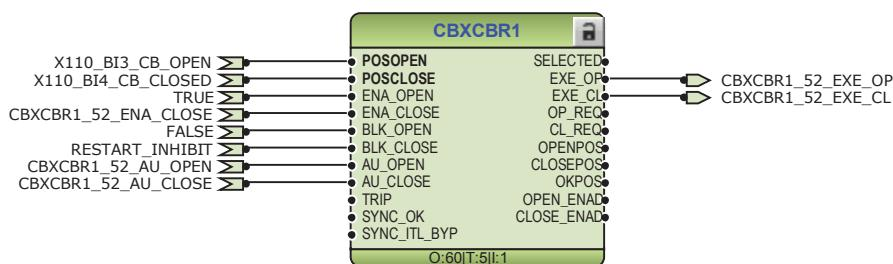
Figure 126: Circuit breaker 1 control logic
