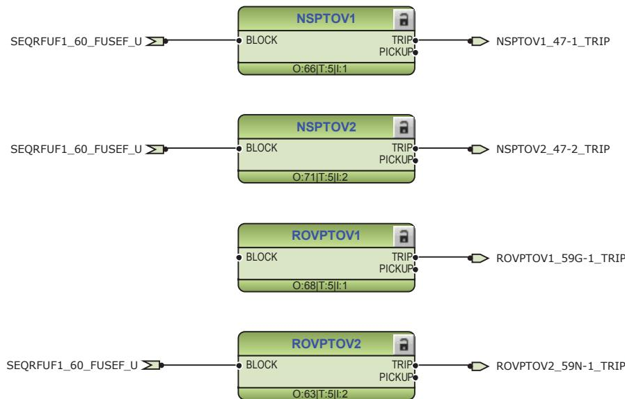
Figure 162: Negative-sequence and residual overvoltage functions
