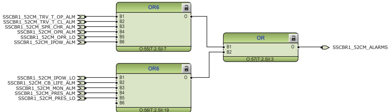
*Figure 32: Logic for circuit breaker monitoring alarm*
