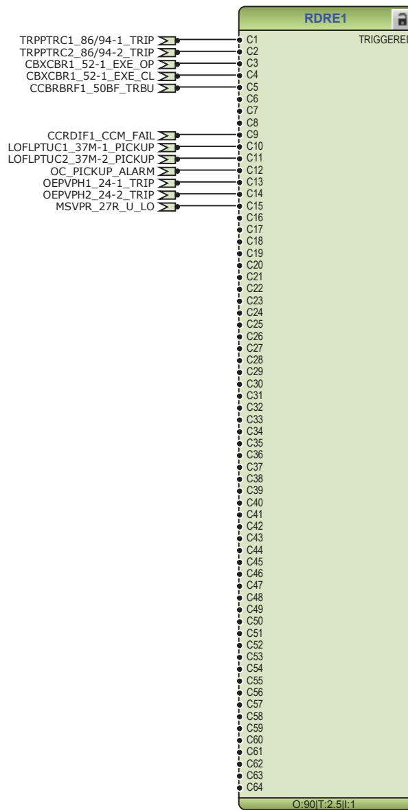
Figure 178: 64 channel disturbance and fault recorder
