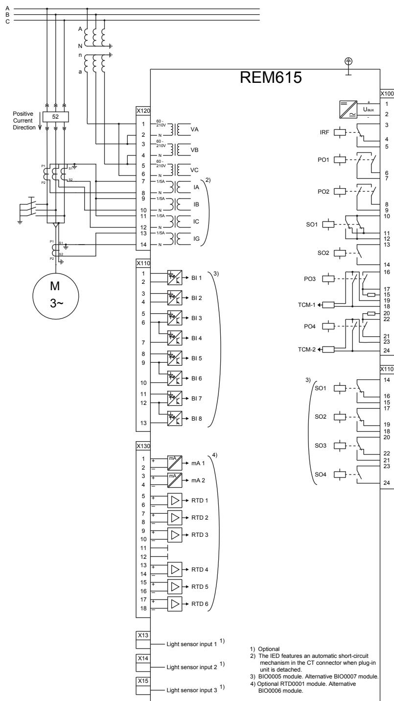
Figure 10: Connection diagram for the B configuration
