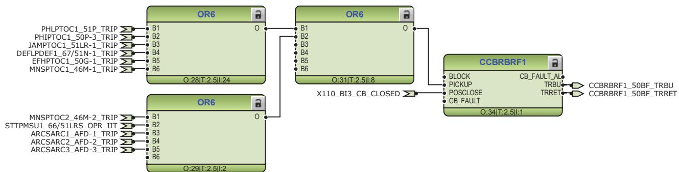
**Figure 67:** Circuit breaker failure protection function
