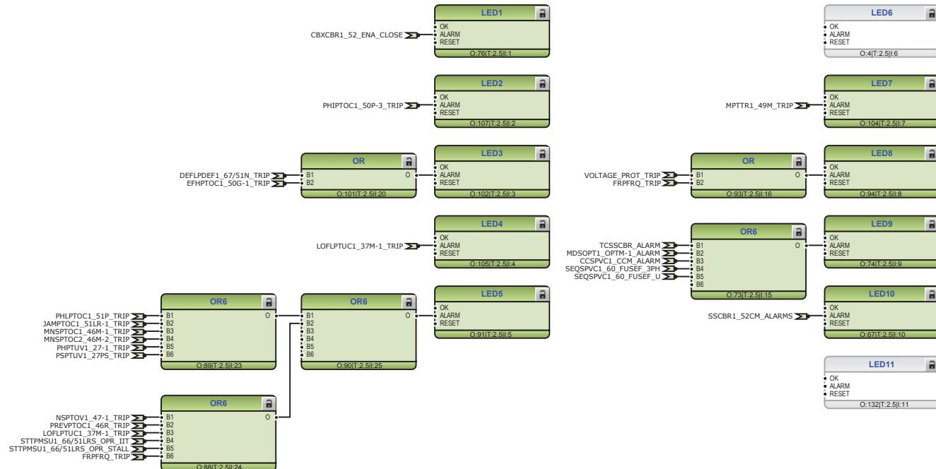
Figure 144: Default LED connections
