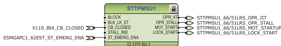
*Figure 111: Motor start-up supervision function*
