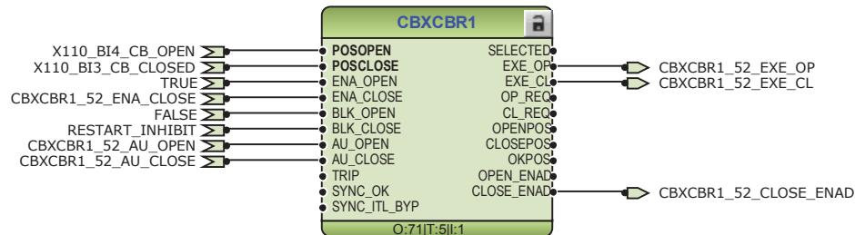
Figure 77: Circuit breaker 1 control logic
