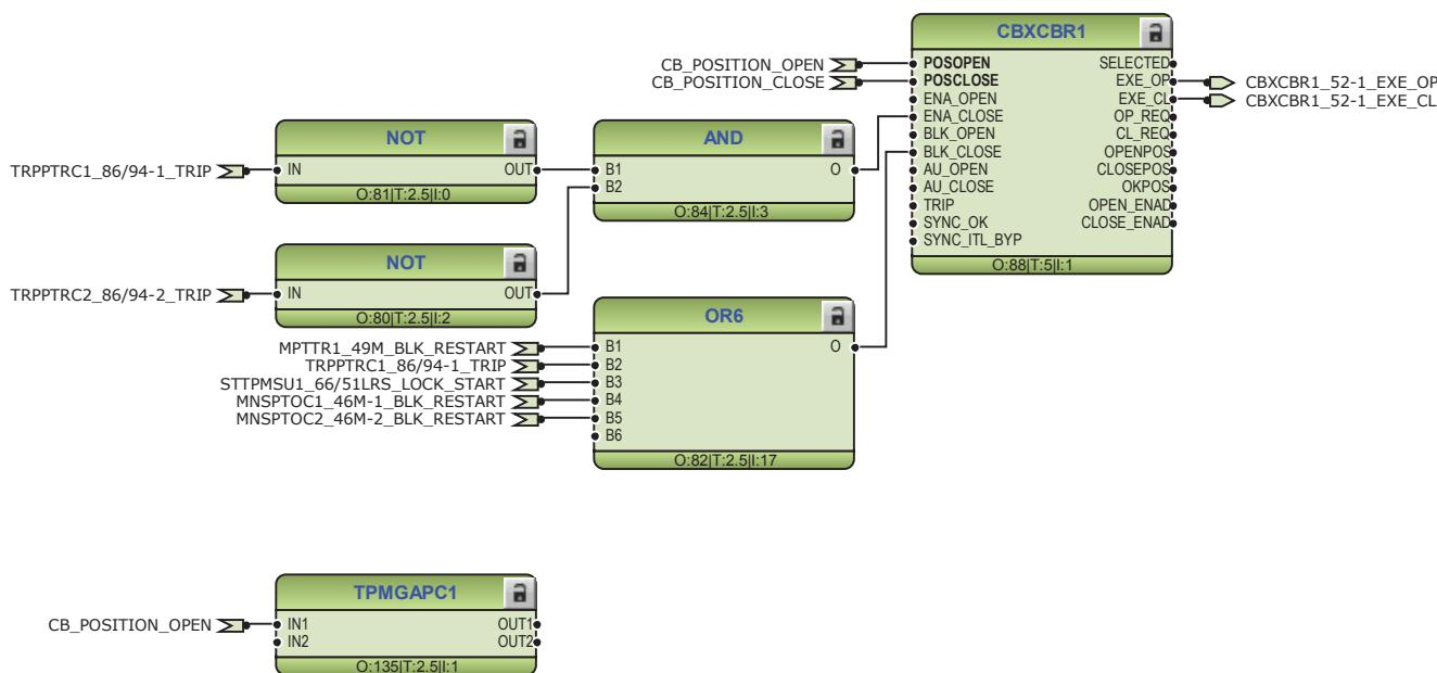
*Figure 185: Circuit breaker control*
