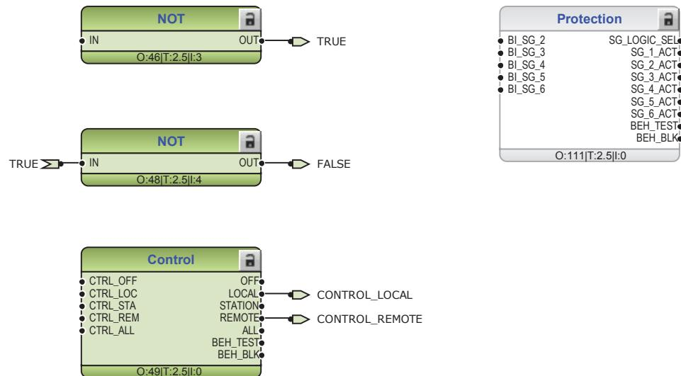
Figure 152: Functions for general logic states TRUE and FALSE, protection setting group selection and local and remote control
