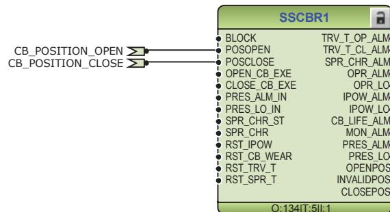
*Figure 183: Circuit breaker condition monitoring*
