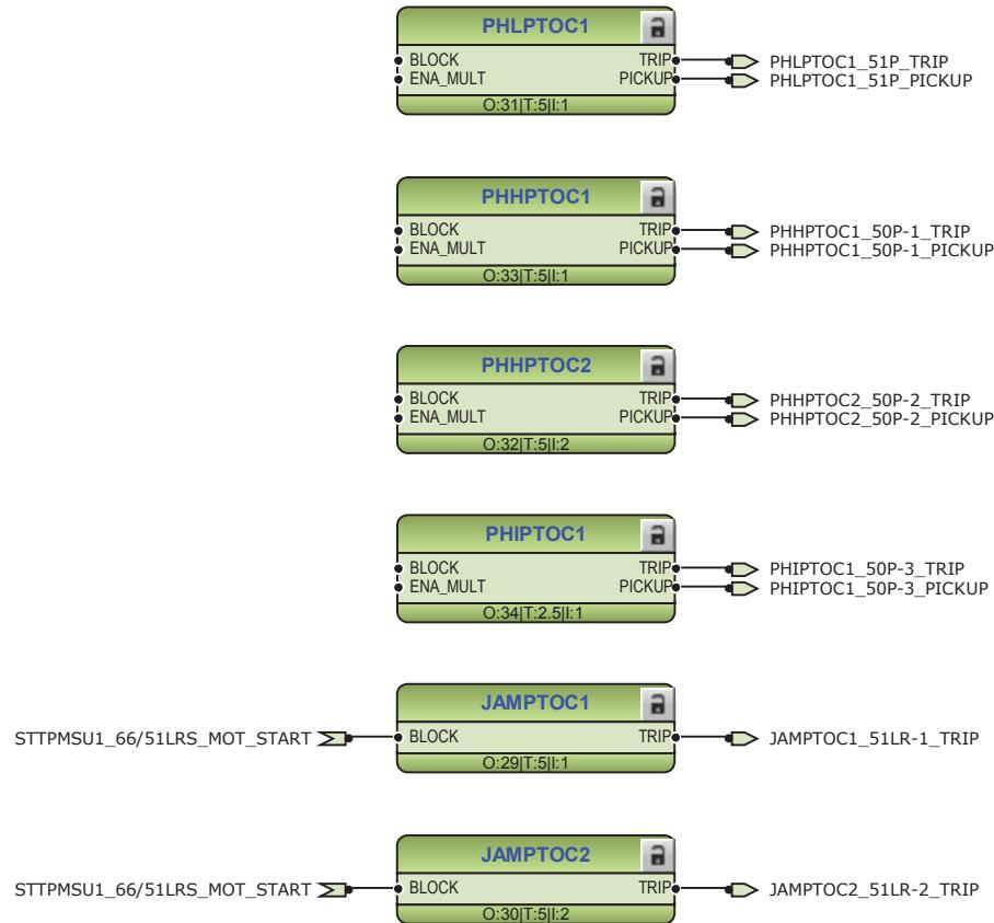
*Figure 157: Non-directional phase overcurrent protections*
