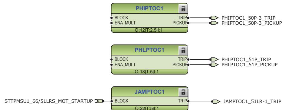
Figure 105: Overcurrent protection functions
