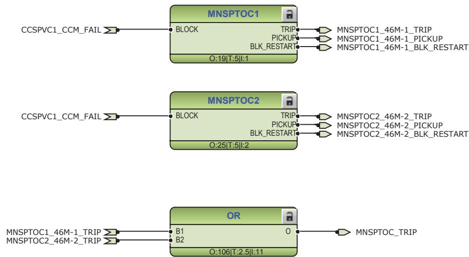
*Figure 56: Negative-sequence overcurrent protection function*
