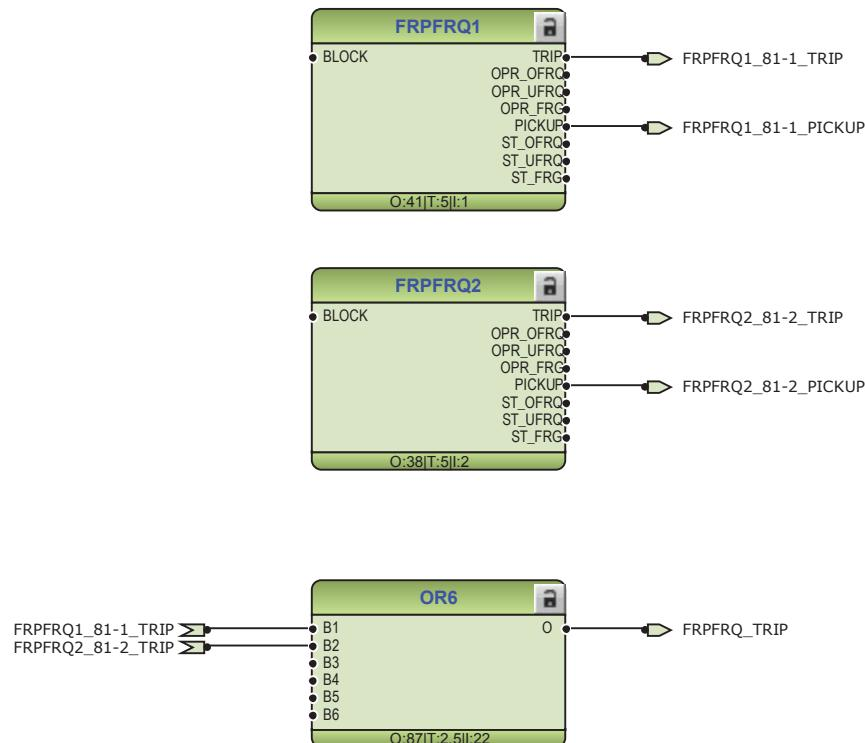
*Figure 115: Frequency protection function*
