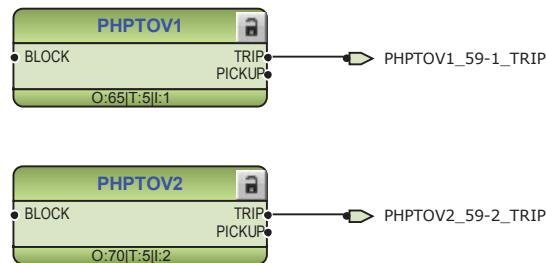
Figure 161: Overvoltage functions
