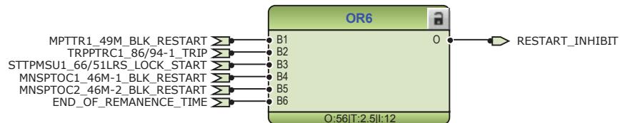
Figure 130: Circuit breaker 1 close blocking logic
