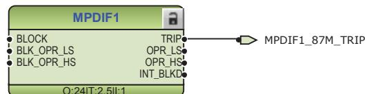
Figure 155: Motor percentage restrained current differential protection
