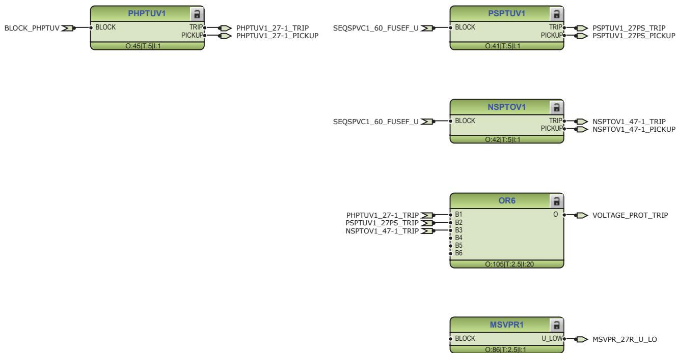
*Figure 65: Voltage protection function*
