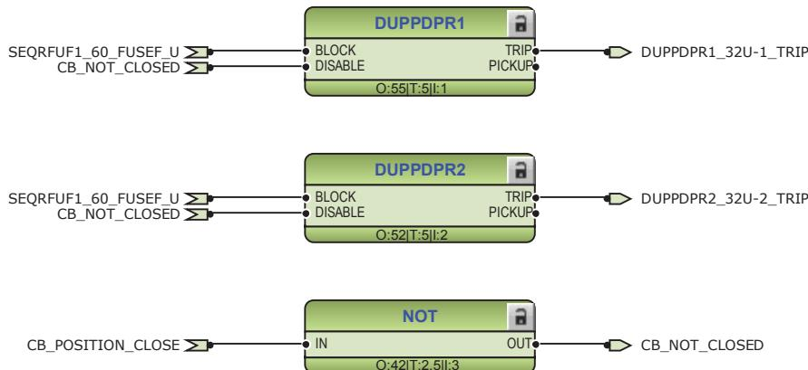
Figure 164: Directional underpower protections
