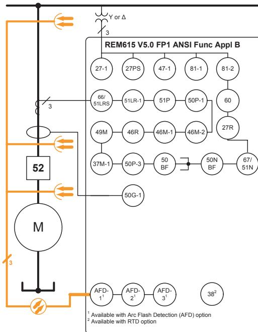
Figure 54: Functionality overview for standard configuration B
