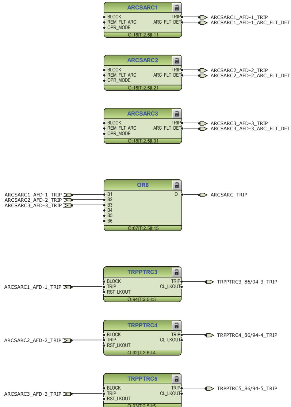
Figure 26: Arc protection with dedicated high-speed output
