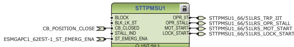
*Figure 169: Motor start-up supervision*
