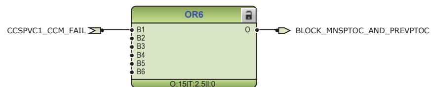
*Figure 147: Blocking logic for phase reversal and negative-sequence overcurrent protection*
