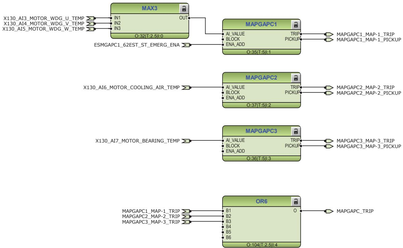
Figure 64: Multipurpose mA/RTD monitoring
