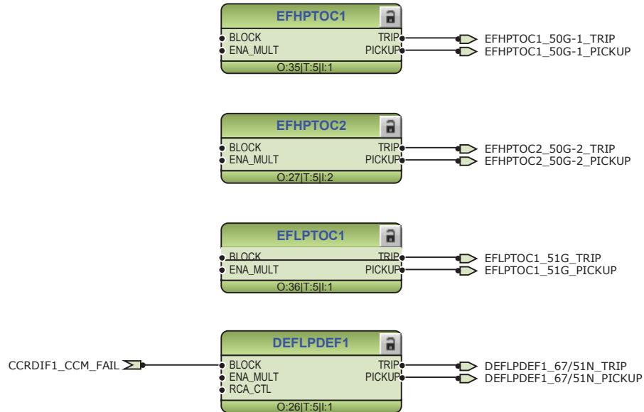
*Figure 158: Ground-fault protections*
