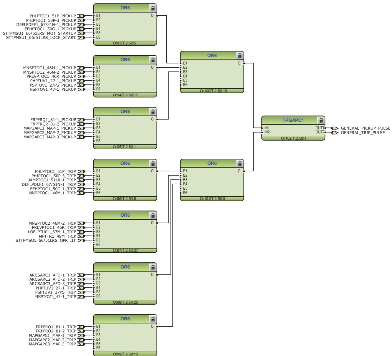
**Figure 69:** General pickup and trip signals
