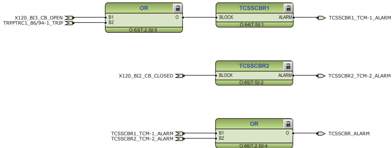
*Figure 33: Trip circuit supervision function*
