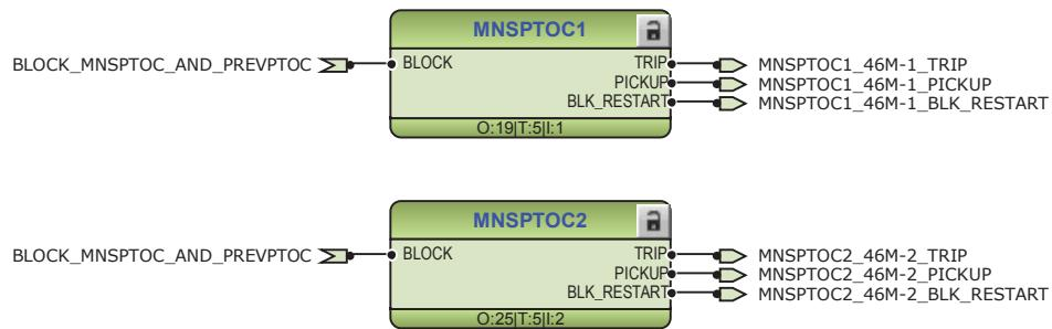
*Figure 106: Negative-sequence overcurrent protection function*
