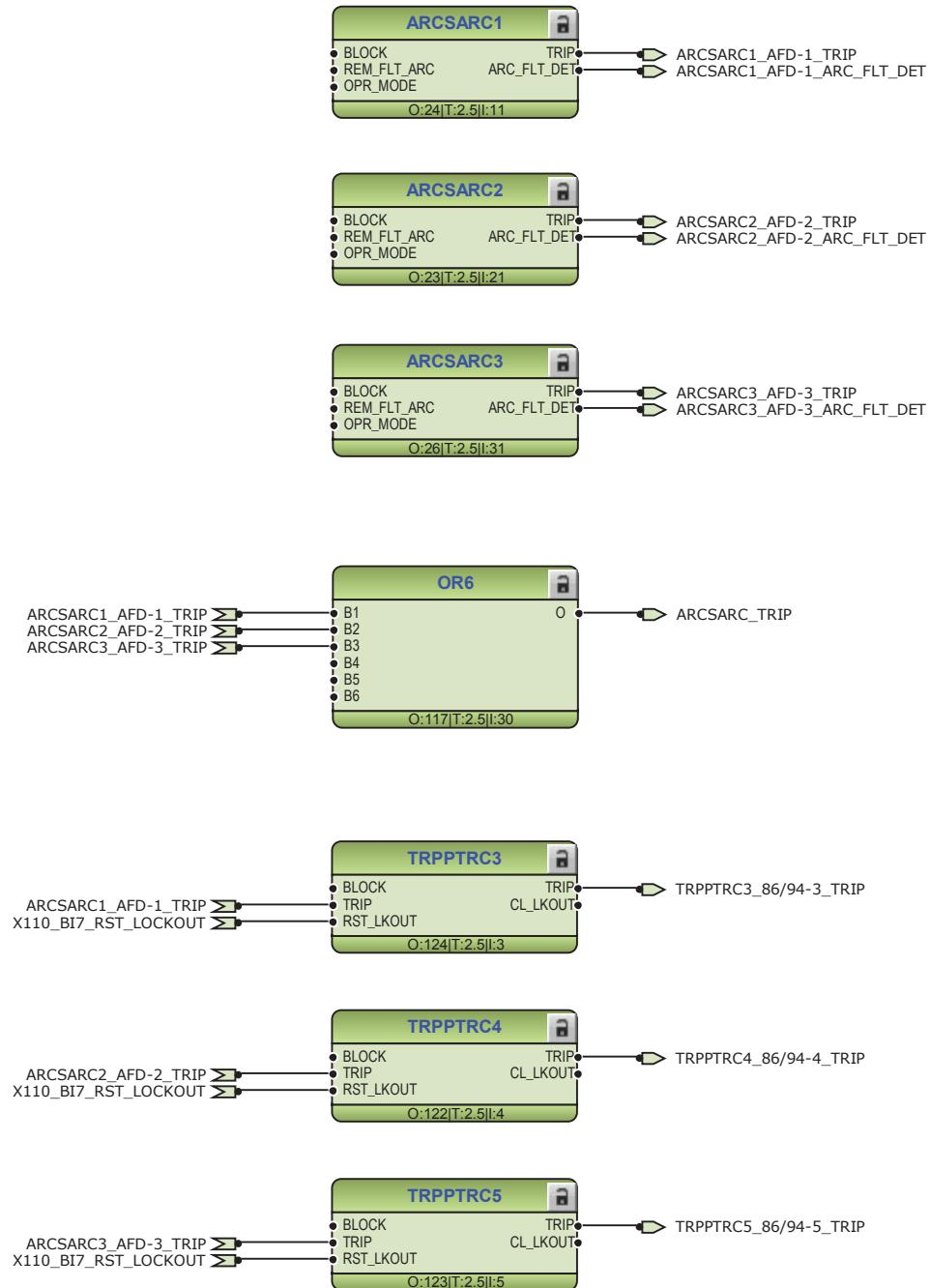
Figure 68: Arc protection with dedicated high-speed output
