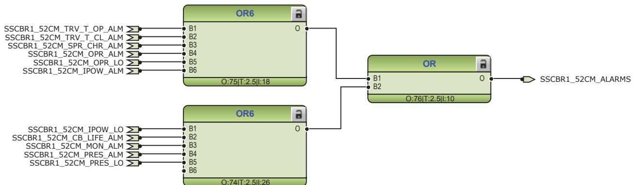
*Figure 75:* Logic for circuit breaker monitoring alarm
