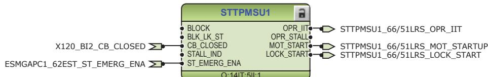
*Figure 21: Motor start-up supervision function*
