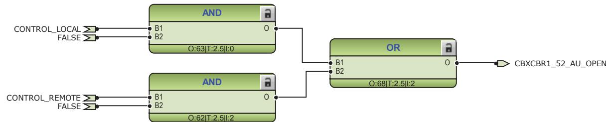
Figure 83: External opening command for circuit breaker 1
