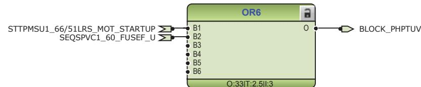
*Figure 99: Blocking logic for phase undervoltage protection*
