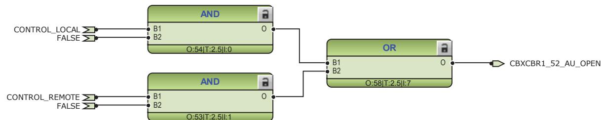
*Figure 132: External opening command for circuit breaker 1*
