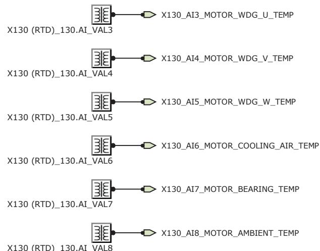
Figure 48: Default mA/RTD inputs - X130
