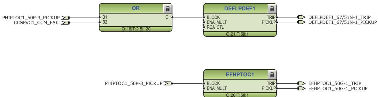
*Figure 58: Ground-fault protection functions*
