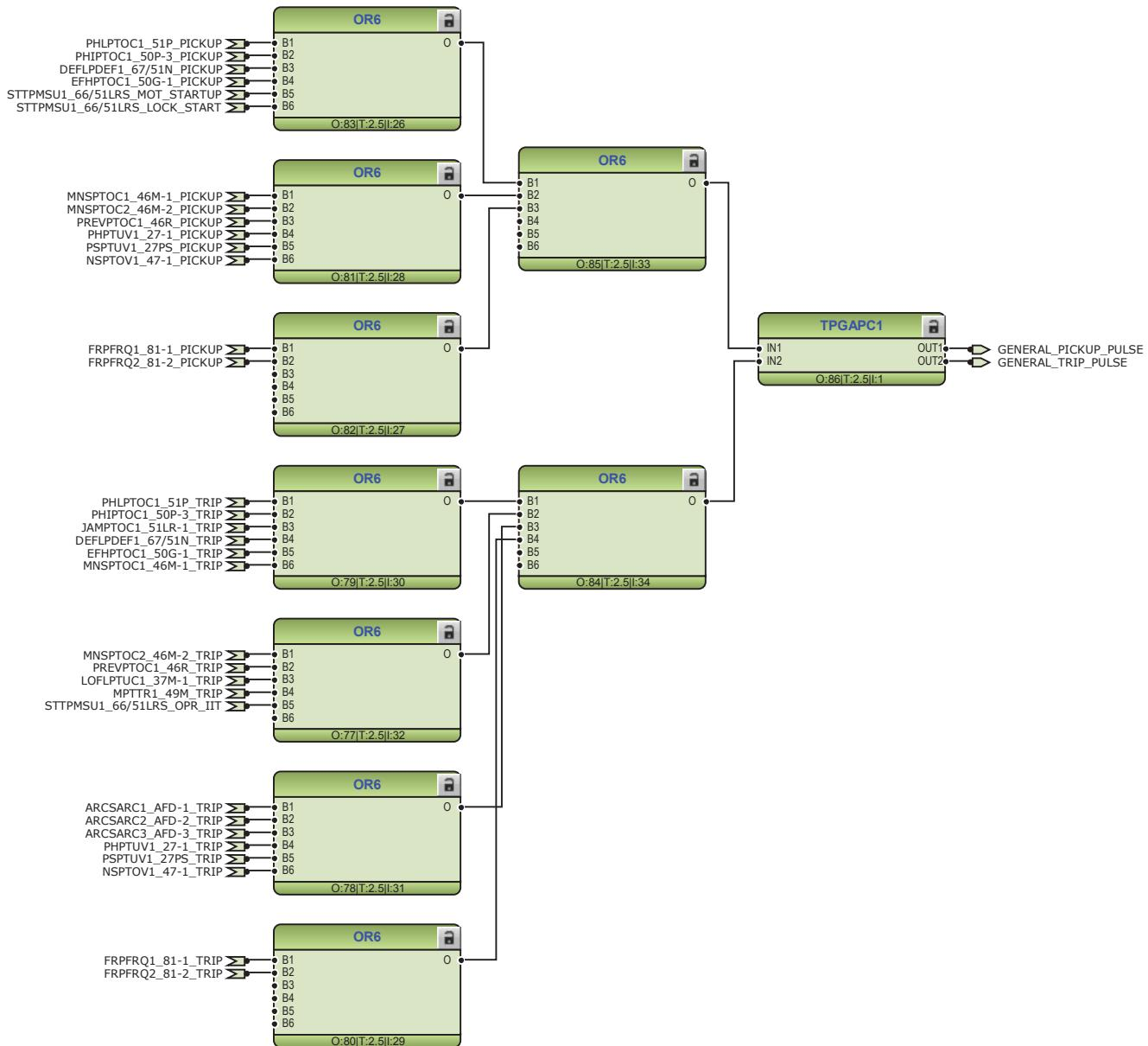
Figure 118: General pickup and trip signals
