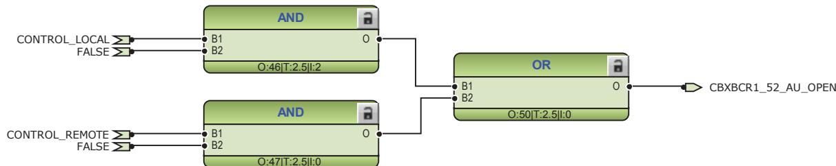
Figure 40: External opening command for circuit breaker 1
