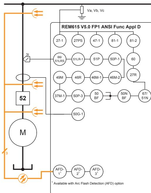
Figure 104: Functionality overview for standard configuration D
