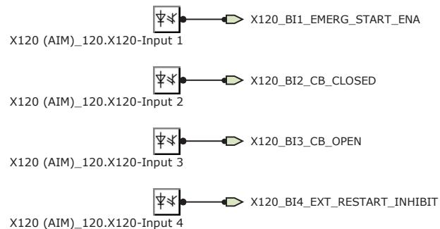
*Figure 45: Default binary inputs - X120*
