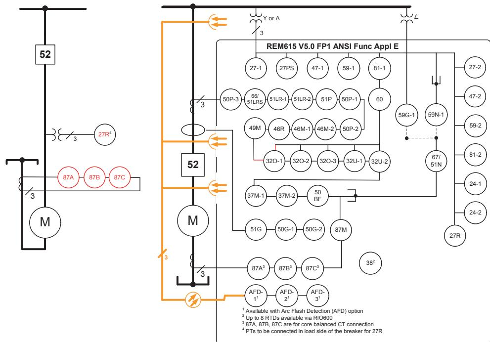
Figure 154: Functionality overview for standard configuration E
