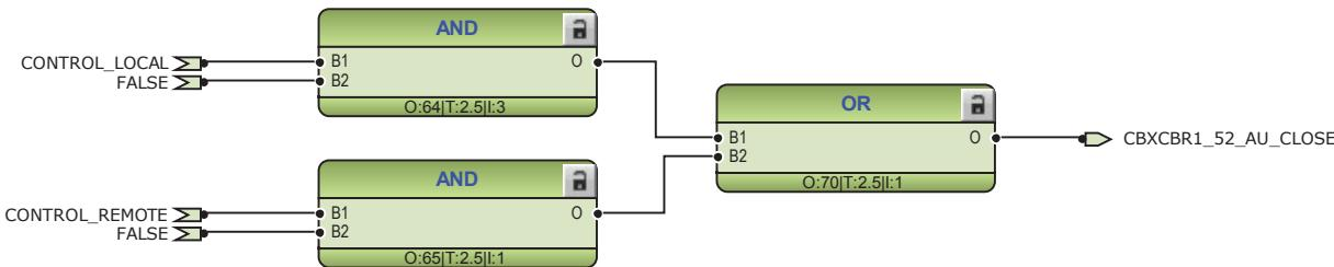
Figure 82: External closing command for circuit breaker 1
