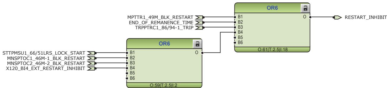
**Figure 38:** Circuit breaker 1 close blocking logic
